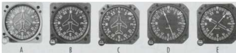
Fig. 4-46. Electric heading indicators. A. 28- or 14-volt DC free (nonslave) gyro. B. 115-volt, 400Hz (cycles) free directional gyro. C. 115-volt, 400-Hz slaved heading indicator. D. Slaved H/1 with RMI (115-volt, 400-Hz). E. Slaved H/1 and RMI with dual pointers (115-volt, 400-Hz). (Aviation Instrument Manufacturing Corporation)
