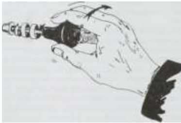
Fig. 12-3. 1. Using the lock button for large rpm adjustments. 2. Using the vernier for smoother, mmor adjustments. The propeller control is being turned to obtain higher rpm in the illustration.
