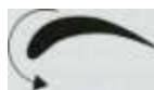
Fig. 10-66. Flexure and torsion (twist) of a wing. These will not be in phase with each other, which is one cause for onset of flutter.
