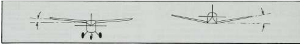
Fig. 10-56. Dihedral requirements for a high- and a low-wing airplane to obtain equivalent lateral stability.
