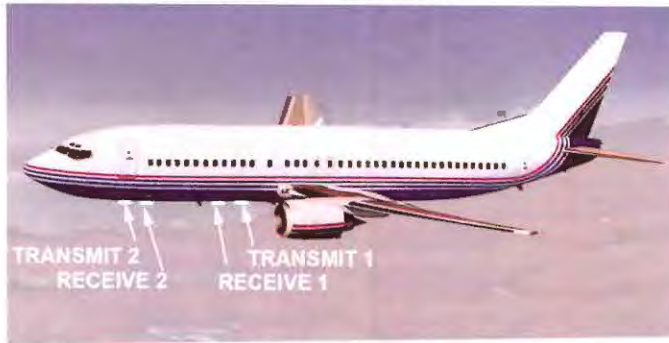
Two independent radar altimeters are installed for some instrument operations requiring separate antenna installations.
