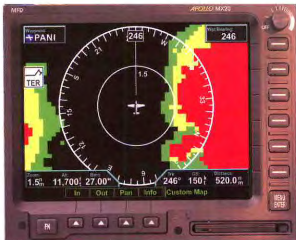
The 360-degree compass rose is a horizontal situation indicator. The red, yellow and green areas are terrain warnings.
