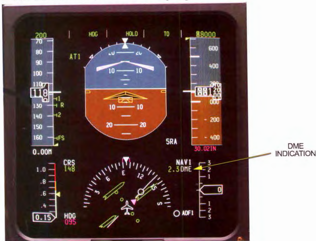
DME distance appears on the EFIS screen, near the compass rose (horizontal situation indicator). "NAV 1" shows it's reading data from the No. 1 VOR receiver.
