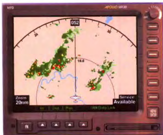
Weather shown here is not from aircraft radar, but signals from NEXRAD, a nation-wide system of government ground radars. The pilot may select weather images from any area of the country.
