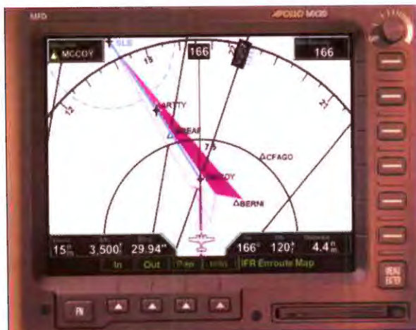
Navigational charts for enroute and approach phases of flight. When the airplane lands, the chart changes to a taxi diagram.
