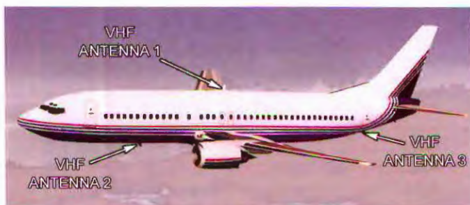
Three VHF com radios are often carried aboard airlines; the antenna locations are shown above. VHF com 1 and 2 are for communicating with air traffic control. VHF com 3 operates in the ACARS system for what is commonly called “company communications.”
