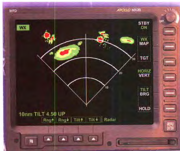
This screen shows weather radar images and works with several makes of radar sets.
