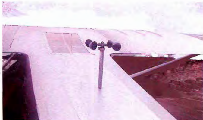
Wind-driven anemometer powered Lindbergh's earth-inductor compass
