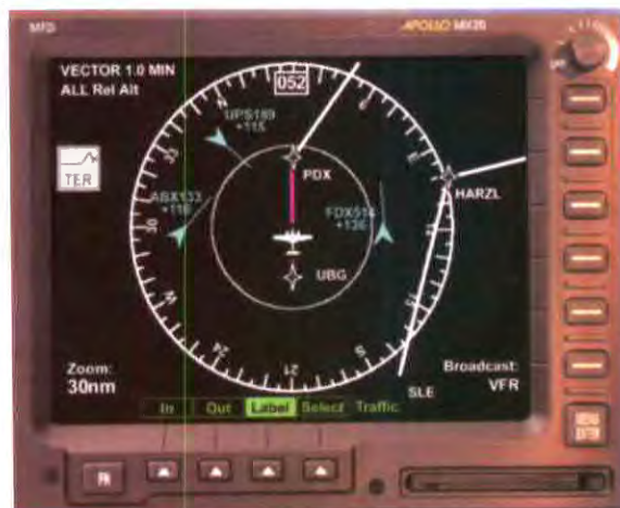
Horizontal Situation Indicator with waypoints along the route. Also shown is nearby traffic; targets appear as small blue arrowheads.
