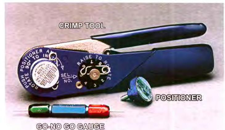
This crimp tool has wide application among miniature and sub-miniature connector types. It delivers a standard 8-impession crimp. When the handles are squeezed, a ratchet controls maximum pressure. A selector knob sets the correct wire depth. The "go-no go" gauge checks the tool's accuracy. The "positioner" holds the contact in the correct position. The model shown is the DMC AFM, also known as "Little Blue."
