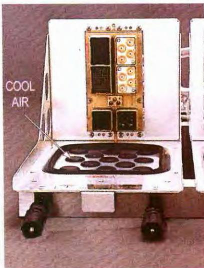
Holes in bottom of ARINC-type tray admit air to cool avionics.
