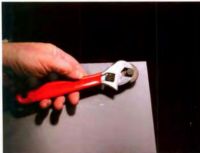
The hole punch cuts into the panel as its nut and bolt are tightened with a wrench.
