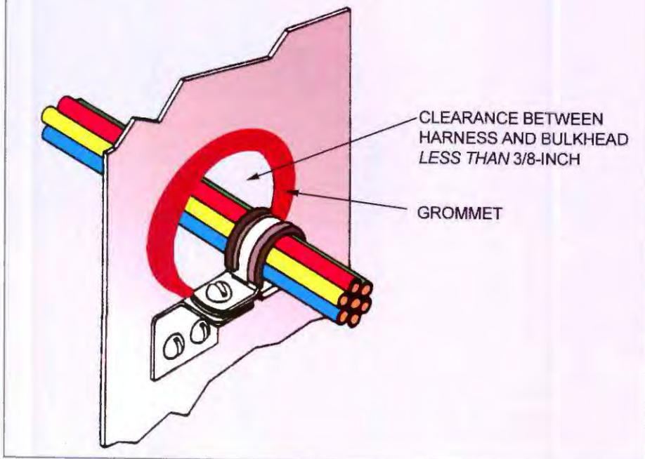
If there is less than 3/8-inch clearance, add a grommet to the hole. There are many openings in an airframe for running wire harnesses. They're known as "lightening holes" because they lighten the airframe. They are not "lightning" holes.
