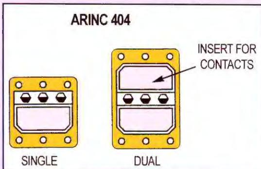
ARINC 404 is aboard airliners that began production during the 1960's. This includes first models of the Boeing-727, -737, -747 and Airbus-300. Instruments and radios operate on conventional (analog) principles, which require fewer pins than today's avionics. These connectors are set up for various equipment by different inserts (which hold the contacts). The ARINC 404 connector is still needed on most recent airliners.
