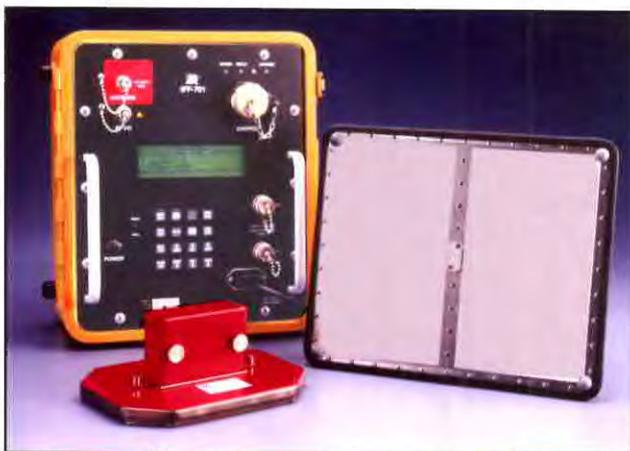
The IFF-701 is a flightline transponder tester. It performs single checks or an autotest that runs 30 tests automatically. The tester communicates with the aircraft through its antenna. The red object at the lower left is an antenna shield, which covers one aircraft antenna in installations where there are two transponders (in an anti-collision, or TCAS, system).
