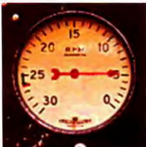
Tachometer from a 1931 Piper Cub is a 3-inch instrument that shows one function: RPM.
