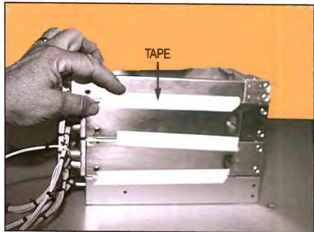
While wiring a radio stack on the workbench, tape the sides of the trays together. This keeps the trays stable while you wire the harnesses at the rear. Remove the tape just before installing the stack in the airplane.
