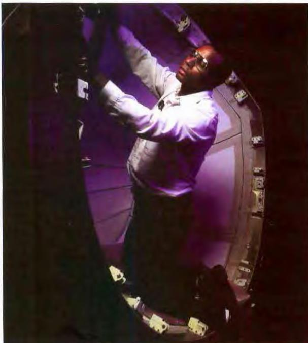
Quartz radome used on the Airbus A-320.
