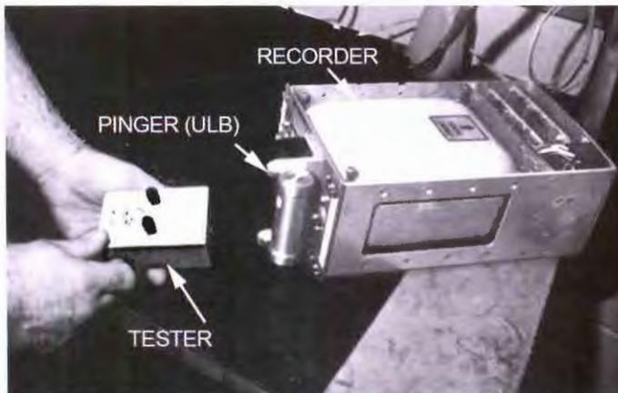
When testing the underwater locator beacon (the "pinger") the tone is ultrasonic and cannot be heard by the ear. The tester receives the tone and converts it down to the range of human hearing. To start the pinger operating, one end is moistened to simulate an underwater condition.
