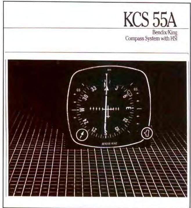
Typical manufacturer's manual for General Aviation, in this illustration a Bendix-King compass system with a horizontal situation indicator. Always check the model number on the unit and compare it with the manual. For example, the model name "KCS 55A" may not be the same as "KC 55," although the illustration may appear the same.
