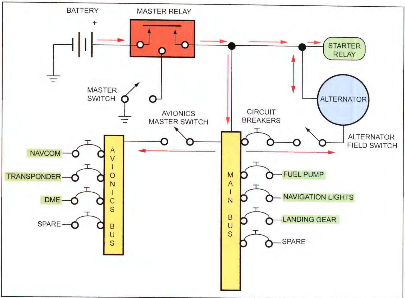
The electrical system for a single-engine airplane. Starting at the upper left, there is a storage battery with its negative terminal grounded to the metal airframe and engine block. To energize the electrical system, the pilot turns on the master switch which operates the master relay. The relay keeps heavy starting currents from moving through the master switch—and delivers those currents to the starter relay. The red arrows show the distribution of current through the system.
