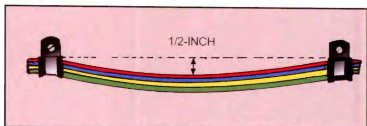
Install clamps at distances no more than 24 inches apart. When you grab the wire bundle and give it a *slight* pull, it should not move axially (to the left or right in this illustration). The bundle may droop up to 1/2-inch under normal conditions. That slack may be exceeded if you are sure the bundle cannot touch a nearby surface and suffer damage from abrasion (rubbing).
