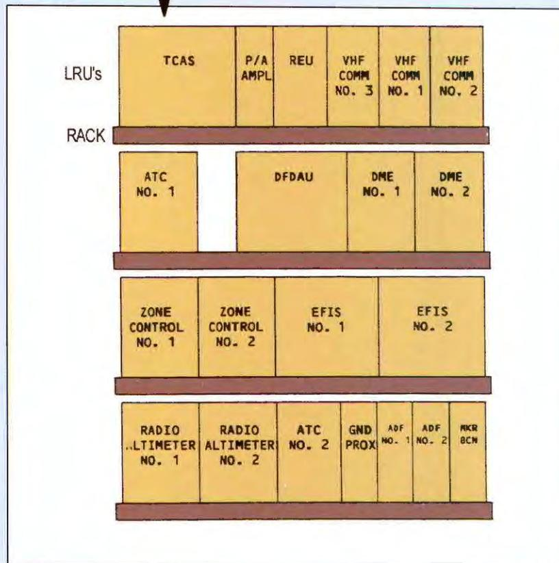
Typical mounting for remote avionics in an airline installation (a Boeing-737). Located below and behind the flight deck is the "E/E bay," a compartment for electronics and electrical systems. The LRU's are slid into racks and locked in trays. The rack shown here contains nav, com, display, transponder, radio altimeter, ADF and other systems.
