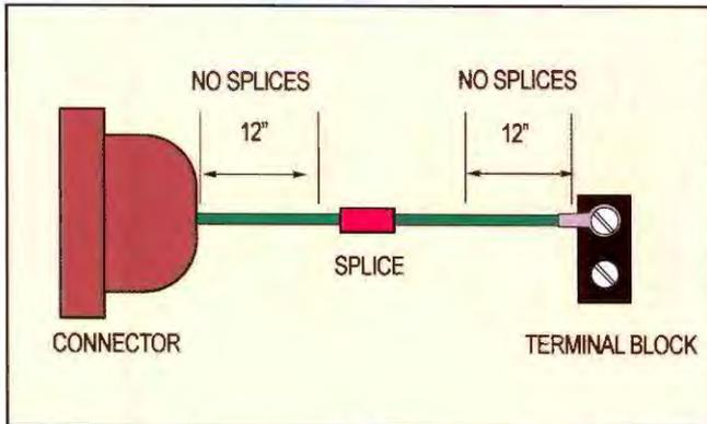
Avoid splicing a wire more than once in a segment, which runs between any two terminal points, such as a connector, terminal block or disconnect point. (There are certain exceptions.) Note that a splice should not be less than 12 inches from the terminal points at either end.
