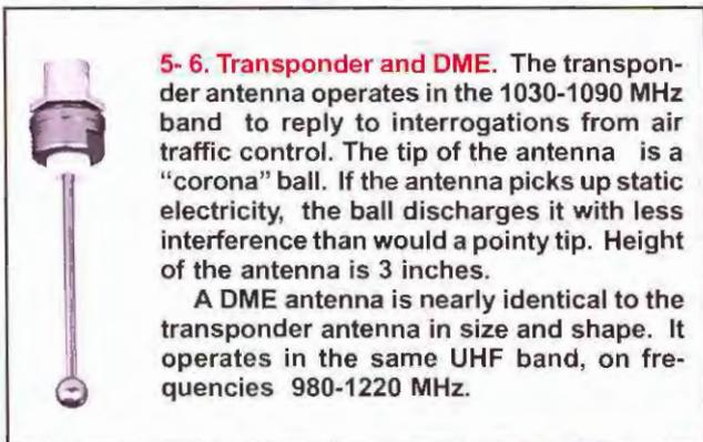
**5- 6. Transponder and DME.** The transponder antenna operates in the 1030-1090 MHz band to reply to interrogations from air traffic control. The tip of the antenna is a "corona" ball. If the antenna picks up static electricity, the ball discharges it with less interference than would a pointy tip. Height of the antenna is 3 inches.
