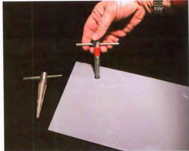
A hand reamer cuts holes in panel for switches, controls and other small items. First, a pilot hole is made with an electric drill.
