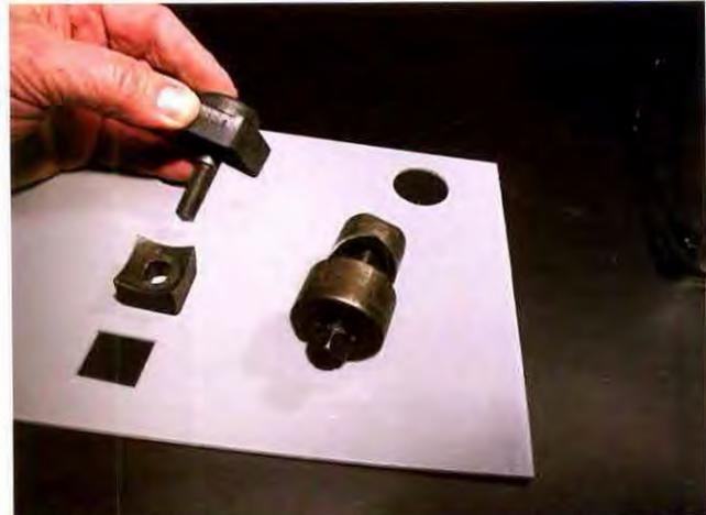
A hole punch cuts neat round or square holes in panel. A square one is at the left, the other is a round one. Punches are also made for cutting odd-shaped holes required by some instruments.
