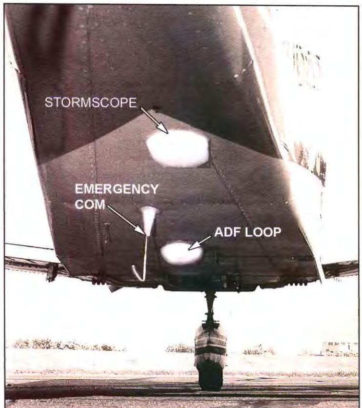
**Belly of a single-engine aircraft. Stormscope antenna is for weather (lightning) detection. The ADF loop is forward. Between them is a "bent-whip" com antenna to connect a handie-talkie during radio or electrical failure. Some pilots also use it to listen for clearances while waiting on the ground with the engine off.**
