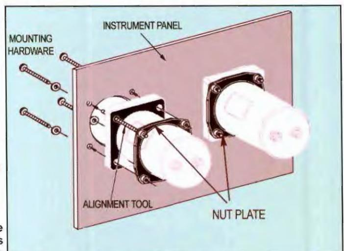
A nut plate is installed by sliding it onto the back of the instrument. To make it match holes in the panel with holes in the nut plate, the installer inserts an alignment tool through one hole, as shown. It's removed when all holes line up, and mounting screws can be inserted.
