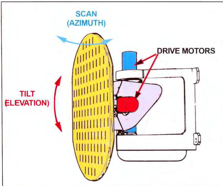
Mounted in the nose of the aircraft, the weather radar antenna sends and receives up to about 300 miles. Scanning motion (side to side) covers an arc of about 120 degrees ahead of the aircraft. The tilt motor keeps the antenna pointed high enough to avoid receiving returns from the earth's surface and cluttering the display. If the antenna is tilted down for the mapping mode, the pilot sees large geographical features such as lakes and coastlines.
