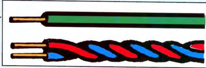
Twisted pair is less susceptible to picking up, or radiating, interference. Twisted pair cables are often shielded for further protection.
