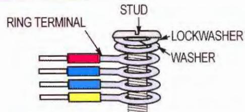
Do not put more than 4 ring terminals under the head of one stud. If more wires must connect, put *three* ring terminals under a stud, plus a *bus bar* (see below). The bar is a short heavy wire or jumper that joins two adjacent studs. This allows three more wires on the second stud, as shown.
