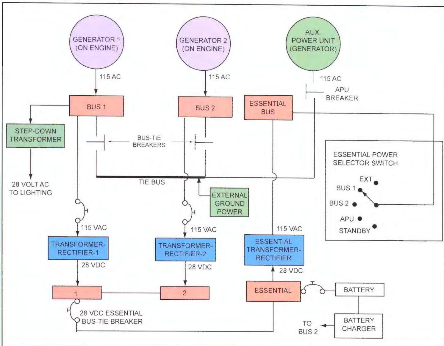
Simplified diagram of the electrical system for a large air transport twinjet. It is designed to give the pilot many options for restoring power in the event of engine failure or other interruption to electrical power. The main features of the system:
