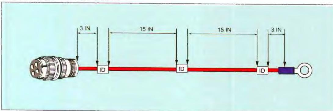
Individual wires should be marked. The recommended spacing is an identification ("ID") marker within three inches of where the wire originates (in this example, a connector, and within three inches of where it ends at the ring terminal at the right). Along the wiring run a
