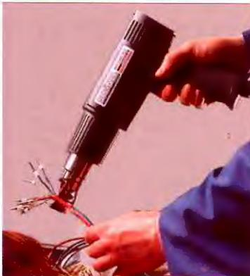
A heat gun (also called a "hot air" gun) is essential for heat-shrink tubing and solder-sleeving.
