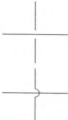
Two additional ways of showing two conductors crossing without making electrical contact
