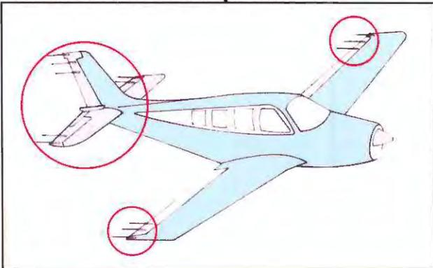
Typical locations are shown for static wicks on trailing edges of wings and tail. Manufacturers of wicks provide drawings for most aircraft that show exact locations.
