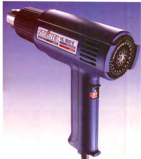
A heat gun like this Steinel 1802 has selectable temperature from 120 F to 1100 F (50 C to 650 C). It consumes 1500 watts at 120 VAC.
