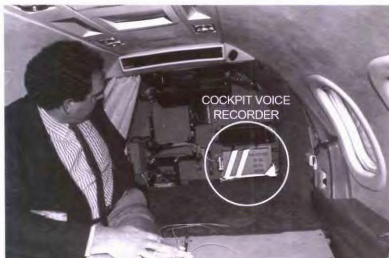
Line replaceable unit (LRU) for a cockpit voice recorder shown located in the aft fuselage of a Learjet. It is usually on the pressurized, or cabin, side.
