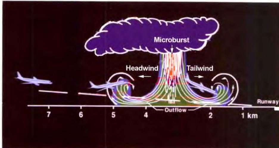
Wind shear---a sudden change in wind direction or speed---is most hazardous when the aircraft is close to the ground, as during an approach. Windshear mostly affects pure jet aircraft because of slow turbine "spool-up" time; a delay of about 4 to 7 seconds after the pilot calls for full power.
