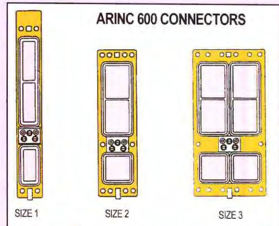
ARINC 600 appeared with the new generation of "digital" airliners during the 1980's, including the Boeing-757, -767 and Airbus A-320. Because of the advanced systems, ARINC 600 provides more contacts in a small area.
