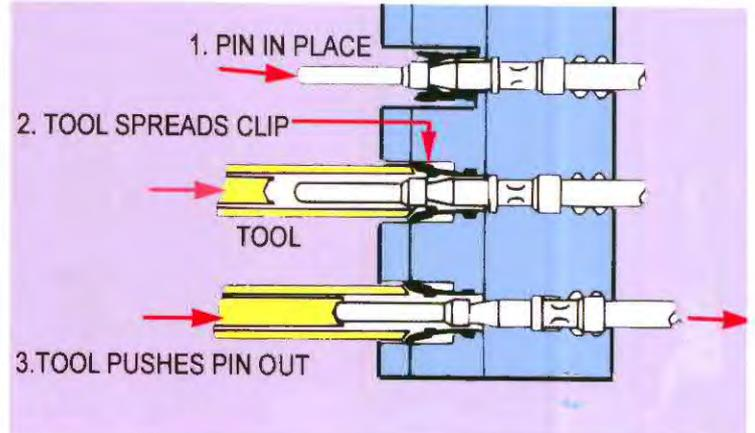
To release pins (1) from a connector, the removal tool is inserted over the pin (2). When the tool seats, it spreads a spring which retains the pin. Now when the tool is pressed further, the pin is pushed (3) out. Shown here is a "front release" connector. Other connectors may be "rear release," but the principle is similar.
