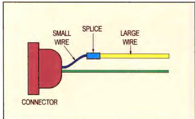
An exception to "one-splice-per-segment" is shown above. If a wire is too large for the connector, splice it to a smaller wire. The small wire from the connector, known as a "pigtail," can be crimped to a connector contact.
