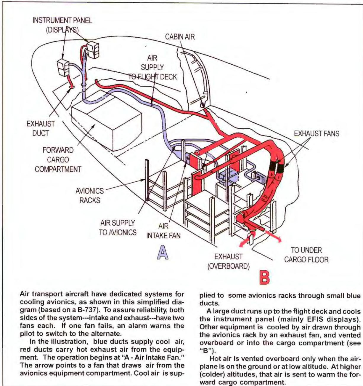
**Fans.** Choose a cooling fan designed for avionics. To be sure, look at the catalog description; it should say PMA and TSO (Parts Manufacturers Authorization and Technical Standard Order---both FAA certifications.) They have brushless DC motors (which eliminate sparking and interference) and are 14- or 28-volt DC.
