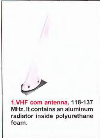
**1. VHF com antenna, 118-137 MHz.** It contains an aluminum radiator inside polyurethane foam.
