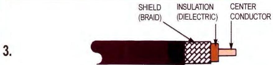
The cable jacket, shield and insulation are trimmed back.
