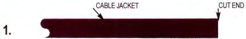
Coaxial cable is trimmed to the desired length. Cut the end of the cable squarely or it won't fit easily into the connector.
