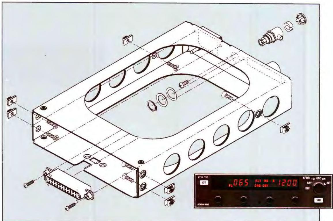
Pictorial illustrations in a manual, like this one for a Bendix-King transponder tray, are essential for mounting hardware. The drawing shows where to assemble connectors and gives details on fastening the tray to the instrument panel.
