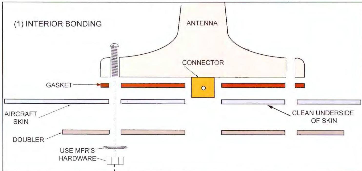
In this approach, the antenna bonds through its mounting screws to the aircraft skin *inside* the fuselage. The inside area, therefore, must be clean and corrosion-free. After clean-up, apply Alodine to the bare skin to slow future corrosion.
