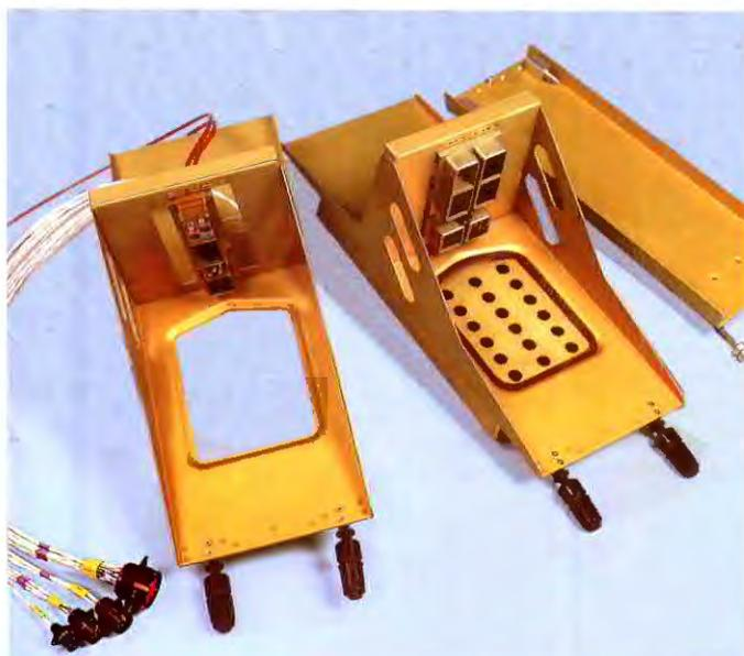
ARINC trays are designed with variations to accommodate different cooling, connector and radio sizes. The black knobs, which lock in the equipment, have a mechanism which cannot be overtightened and damage the connectors.
