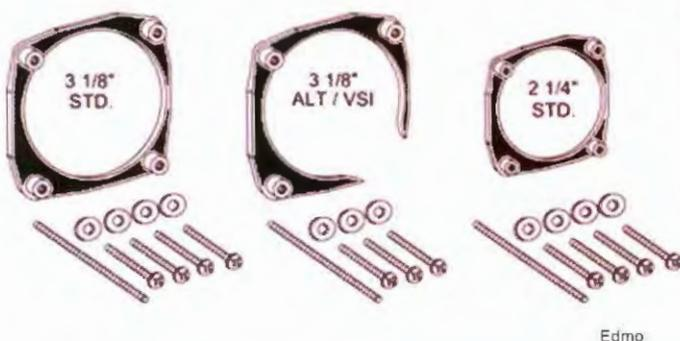
"Nut rings" make the installation job easier. They come in standard 2- and 3-inch sizes. There are two versions of the 3-inch; note the one in the center, "ALT/VSI" which has a cut-out at the lower right. This allows space for the altimeter knob after the instrument is installed. ALT is for altimeter, which has a knob adjusted by the pilot (for barometer setting). VSI (vertical speed indicator) has a small screw adjustment for zeroing the needle.
