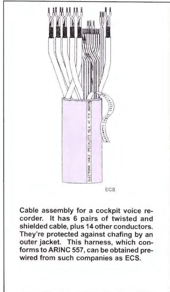
**Cable assembly for a cockpit voice recorder. It has 6 pairs of twisted and shielded cable, plus 14 other conductors. They're protected against chafing by an outer jacket. This harness, which conforms to ARINC 557, can be obtained pre-wired from such companies as ECS.**
