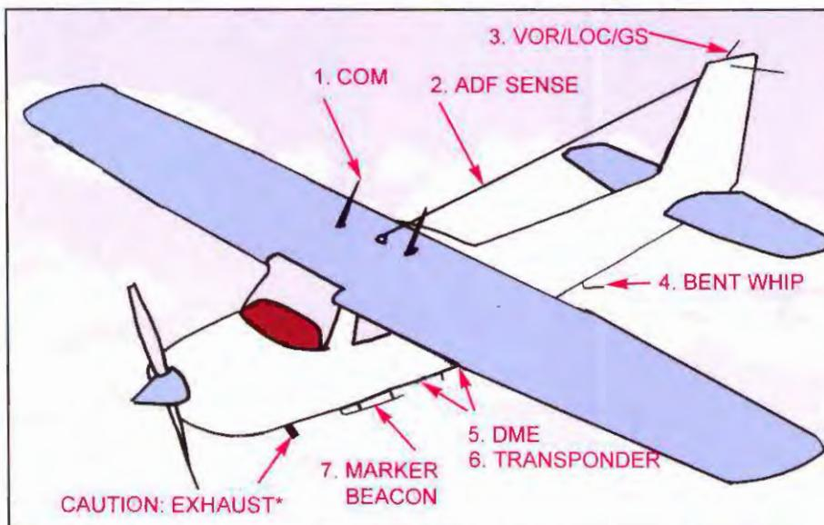
Don't locate an antenna on the belly in line with an exhaust pipe. It becomes coated and discolored. Locate antennas as close as possible to the
