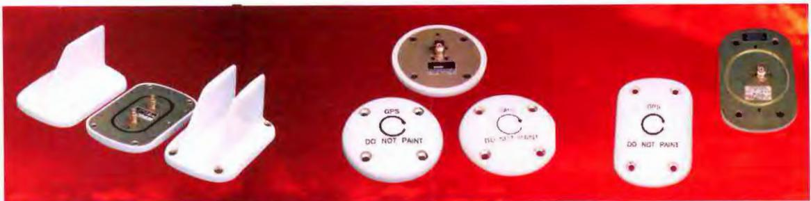
Directional antennas for TCAD (collision avoidance) system. Mounts on top and bottom of fuselage.
