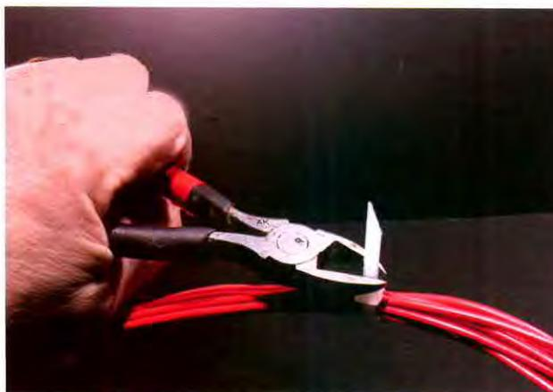
Cut the tab flush with the locking part of the tie wrap.
