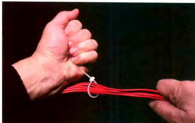
When installing a tie wrap, don’t overtighten it. Pull the tab until the tie wrap is snug around the harness.
