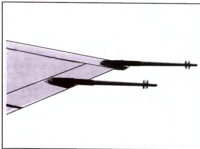
Static wicks reduce P-static by drawing the electrical charge from the airframe and discharging it quietly into the atmosphere. The construction of the wick produces a lower "corona," or discharge, voltage than the airframe.
