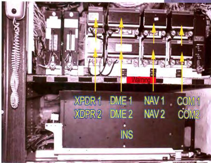
Most LRU's (line replaceable units) are in the lower fuselage. Examples shown include: transponder (XPDR), DME, NAV (VOR receiver) and Com (VHF). Each radio is duplicated for safety. The large dark area in the center ("INS") is the rack for an inertial navigation system (which has been removed for repair).
