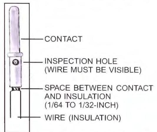
In this type of contact, there is an inspection hole. Bare wire must be visible through the hole. There must also be a small space between the contact and the insulation.
