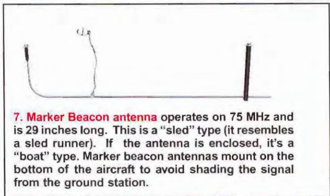
**7. Marker Beacon antenna** operates on 75 MHz and is 29 inches long. This is a "sled" type (it resembles a sled runner). If the antenna is enclosed, it's a "boat" type. Marker beacon antennas mount on the bottom of the aircraft to avoid shading the signal from the ground station.
