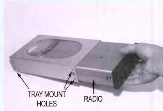
Radio is shown sliding into mounting tray. Holes in the tray are for fastening the tray to the instrument panel.
