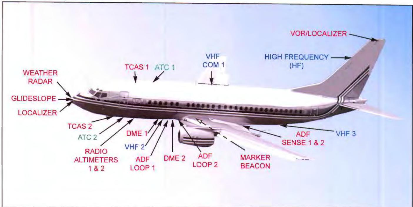
Shown above is a Boeing 737. Antennas divide into three categories, often known as CNI, for Communication, Navigation and Interrogation. Navigation antennas are shown in red, communications in blue. The two interrogation antennas (green) are for ATC, which is the airline term for "transponder."
