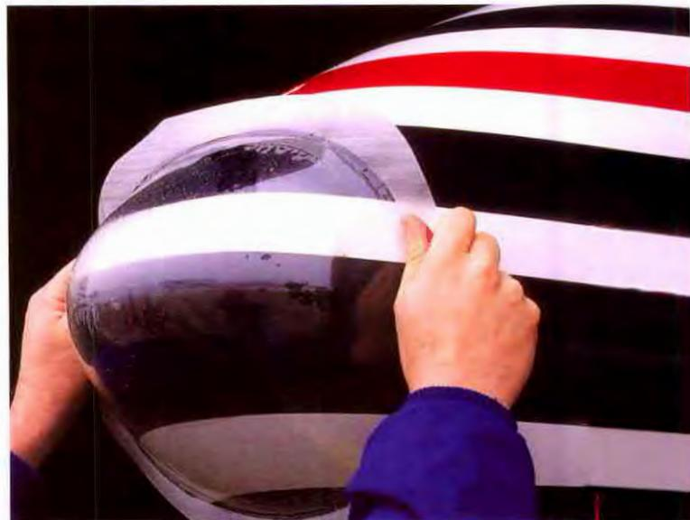
A pre-formed boot made of polyurethane may be applied over the radome for added protection. It reduces the effects of rain, snow, sleet, insects, sand and ultra-violet light
