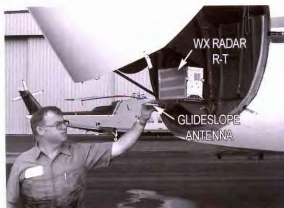
Nose cone is lifted on a corporate jet to reveal glideslope antenna. Weather radar antenna is inside the cone. Above glideslope is the weather radar transmitter-receiver.
