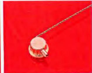
4. Completed job. It takes a fraction of the time required by manual safety wiring and eliminates sharp ends.
