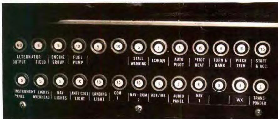
Circuit breaker panel using “recessed button” type breakers. Having no buttons protruding from the panel, they cannot be pulled out by the pilot to disable a circuit.
