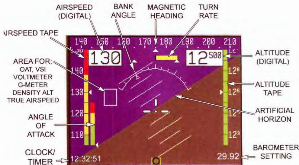
This Dynon 4-inch EFIS screen is only slightly larger than the Piper Cub tachometer above.
