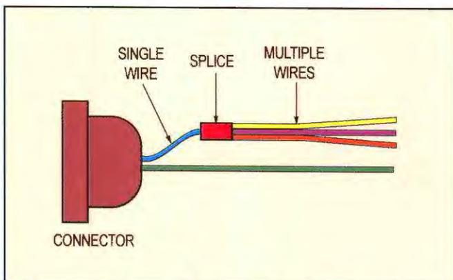
Another exception is when multiple wires need to go to one pin on a connector. They can be spliced to a single wire at the connector.
