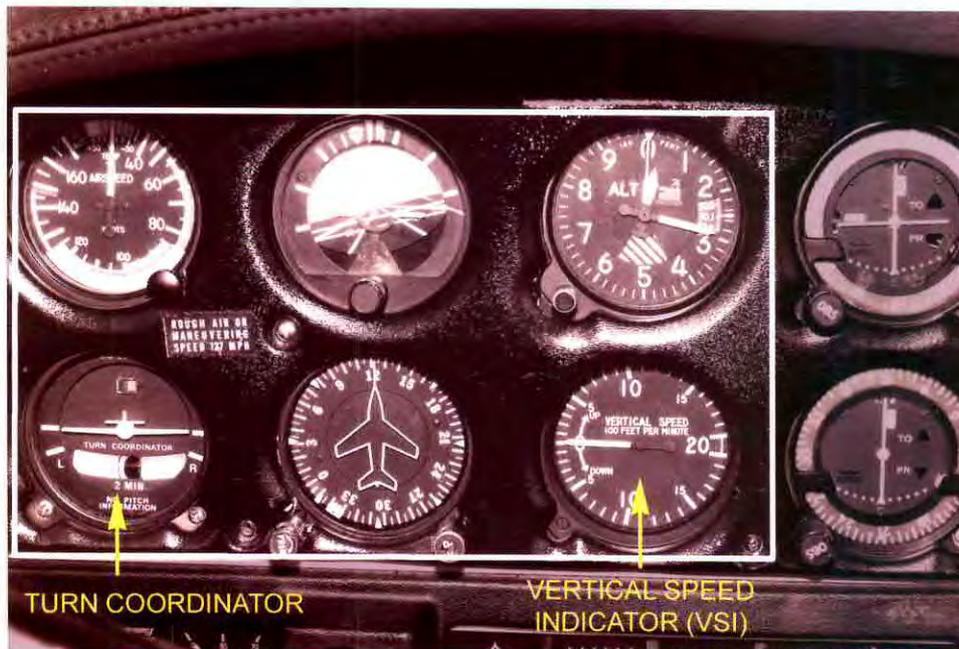
Most light aircraft—Cessna, Piper and Mooney, for example, add the two lower instruments to the basic T; the turn coordinator and vertical speed indicator. This equips the airplane for basic instrument flying. Some technicians call this the “six pack.”
