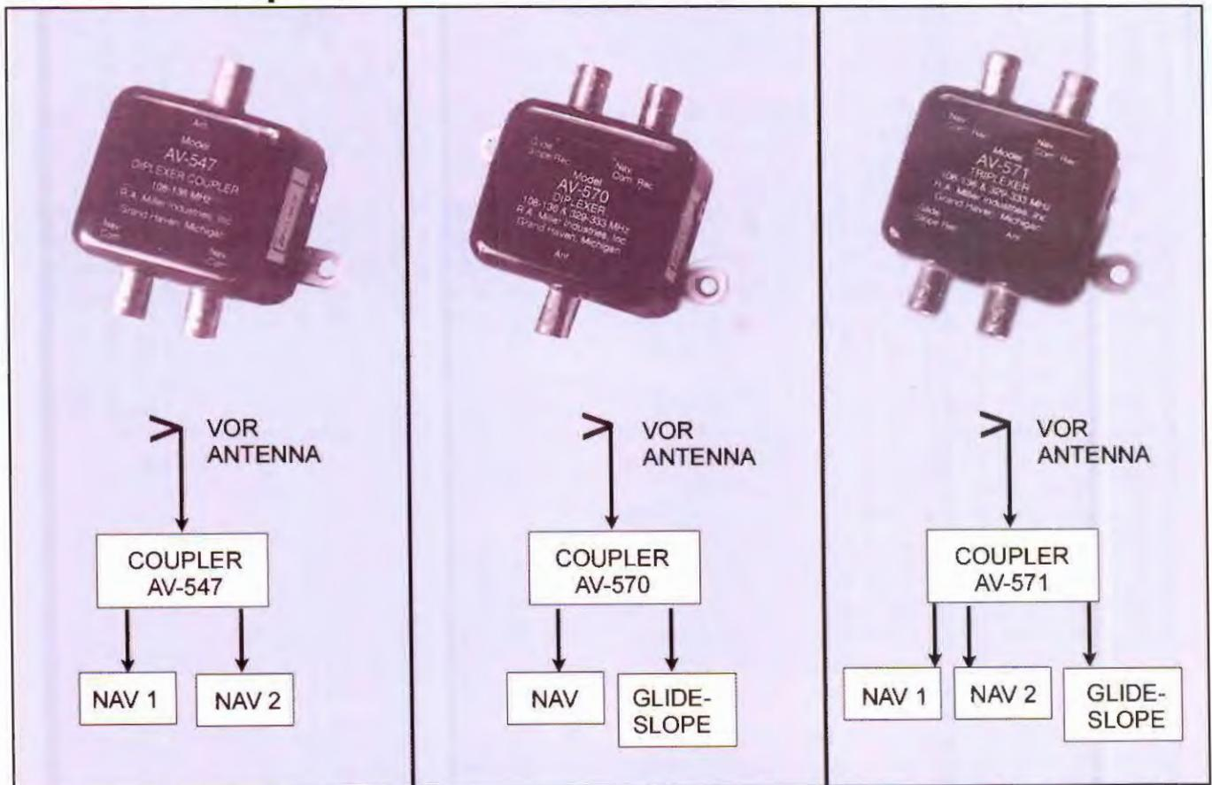
The coupler splits the signal from a single antenna to feed two VOR navigation receivers. As in most couplers, it is only for receivers, which operate on very low-level signals. All couplers reduce the antenna signal by splitting, but there is ample signal strength remaining to do the job.
