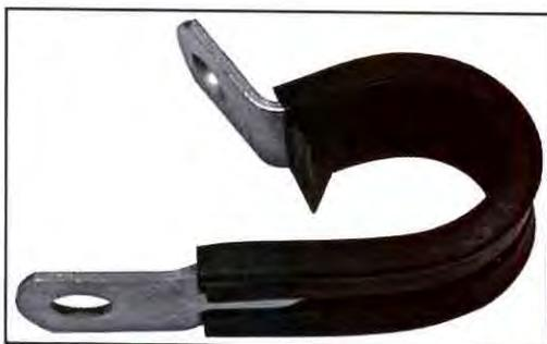
The Adel clamp is often selected for supporting wire harnesses in aircraft. It has a cushioned liner to reduce chafing on wire insulation. The clamp is made in several sizes to accommodate wire bundles of varying thickness.
