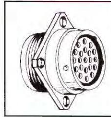
Circular connector with bayonet coupling.
