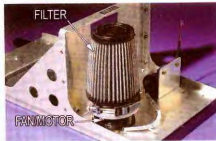
Cooling fan is built into ARINC tray for some airline avionics. A filter removes particles to extend equipment life and raise MTBF (mean time between failure).
