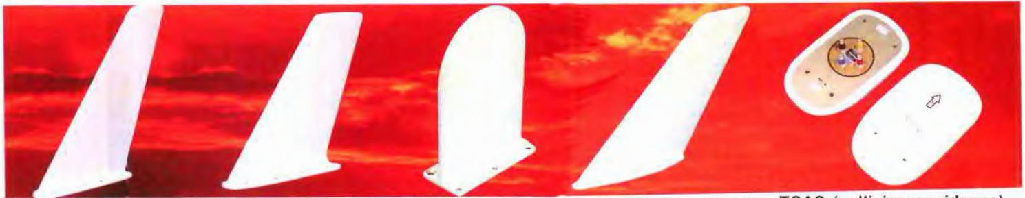
VHF Com, will operate a power rated at 100 watts. Has internal duct for hot air de-icing. Used on Boeing, Lockheed and Douglas.
