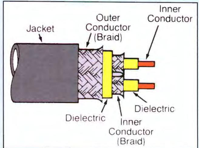
Dual coaxial cable contains two separate coaxial cables covered by a common outer jacket.
