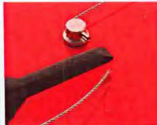
3. As the tool is squeezed it crimps a ferrule on the wire and applies correct tension. The wire is trimmed flush with ferrule.
