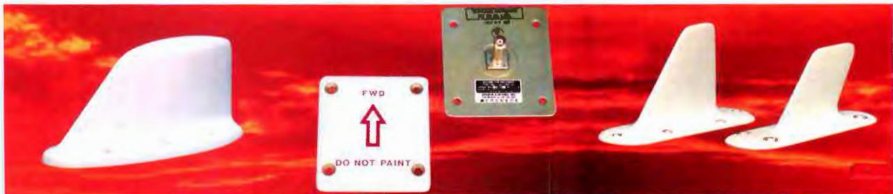
Satcom antenna for operating in Aero-L and Aero-C bands of INMARSAT satellite. It is a low-gain antenna for moving data on 1.5-1.6 GHz.
