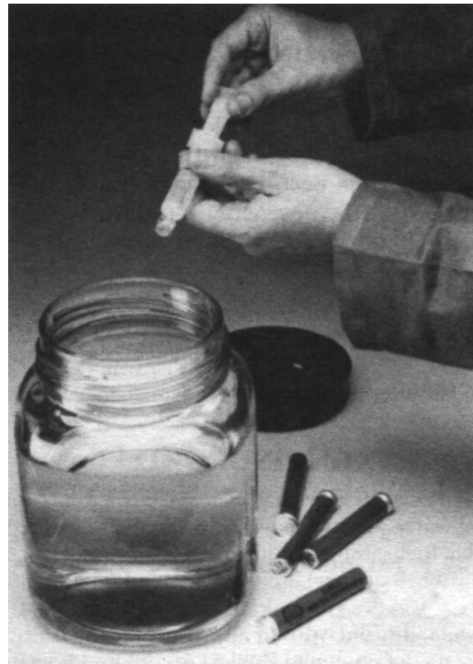
FIG. 1—5 mL syringe and detector capsule. (Reprinted courtesy of Shell International Trading Co., London, England.)
