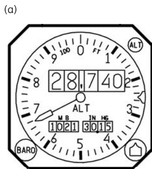
2.3 (a) Altimeter display (b) Altimeter schematic
