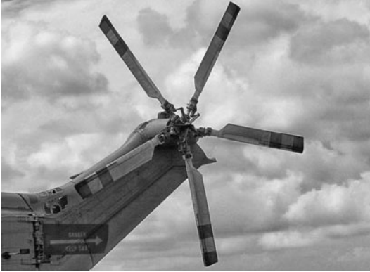
9.7 Tail rotor: (a) Conventional (b) Fenestron®
