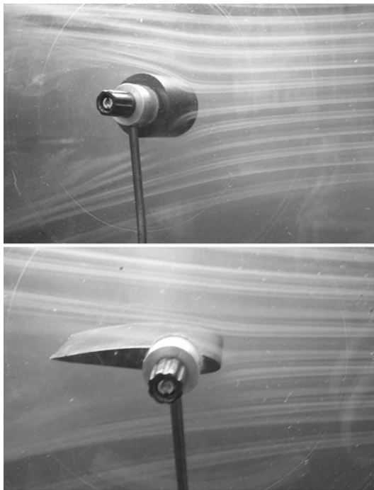
7.20 Smoke generator: flows over a cylinder/aerofoil
