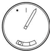
Bank angle too small – A/C tends to slide outwards
