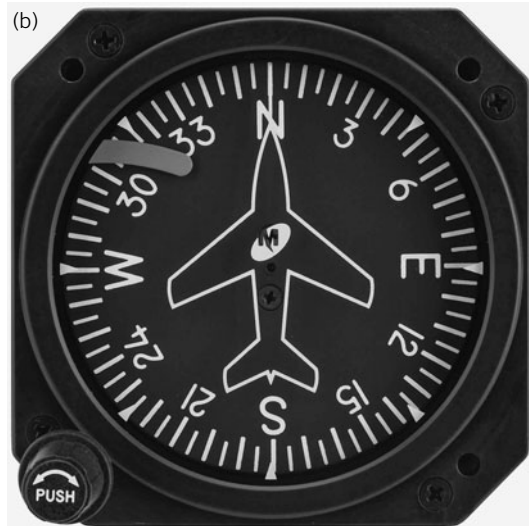
4.12 Directional gyro (a) Internal view (b) DG display
