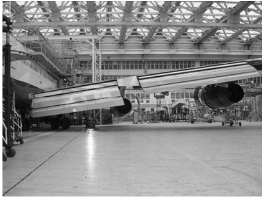
7.57 Trailing-edge flap system of a Boeing 747-400
