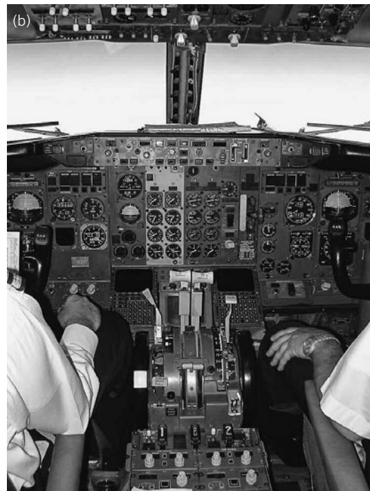
4.4 Instrument panel: (a) GA aeroplane (b) Transport aeroplane
