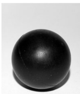
Fig. 4-46. Projectile of the MR-35 «Punch», rubber hollow sphere, Diameter 35 mm.
