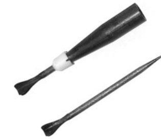
Fig. 2-28. 5.56 × 45 cartridge with flechette, left : cross-section, above : flechette, with and without sabot.
