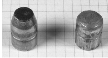
Fig. 4-20. Winchester semi-jacketed bullet, 454 Casull. Left: Before firing. Right: after firing into a simulant. The bullet has only undergone slight mushrooming at the tip. Its diameter has not increased.
