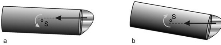
Fig. 2-57. Shoulder stabilization. a. The resultant of the asymmetric distribution of pressure on the face of the projectile generates a stabilizing moment. b. At larger angles of incidence, this moment has a destabilizing effect ( S = centre of gravity).
