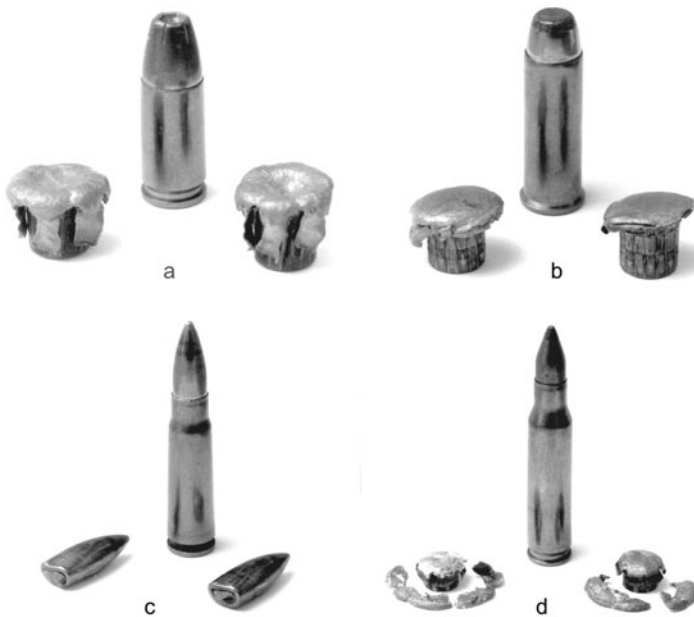
Fig. 3-50. Similarity of deformation in soap (left) and gelatine (right). a. 9 mm Luger, Winchester Subsonic. b. 44 Rem. Mag. SJFP. c. 7.62 × 39, jacketed spitzer. d. 308 Win. SJ Cone.
