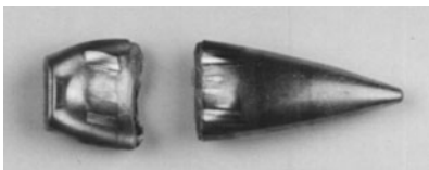
Fig. 3-7. Full metal-jacketed bullet ( 7.62 \times 51 ) after being fired into a block of soap. Part of the lead core was forced out of the jacket and the bullet has fractured at the cannelure.
