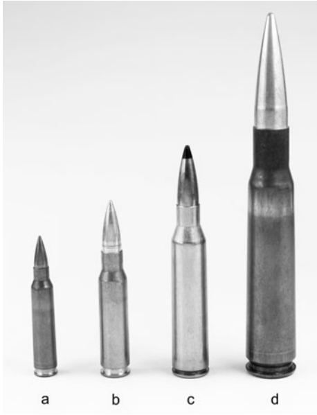
Fig. 2-22. Sizes of military cartridges: a. 5.56 mm NATO (5.56 × 45, 223 Rem.), b. 7.62 mm NATO (7.62 × 51, 308 Win.), c. 338 Lapua Magnum (8.4 × 69), d. 50 Browning (12.7 × 99) with solid brass A-Max bullet. The second number of the metric designation is the case length in mm.
