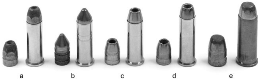
Fig. 2-19. Revolver cartridges and bullets: a. 38 Spl SJHP b. 38 Spl Metal Piercing c. 38 Spl Winchester Hydra-Shok d. 357 Magnum, Remington Golden Saber e. 44 Rem. Mag. SJFP
