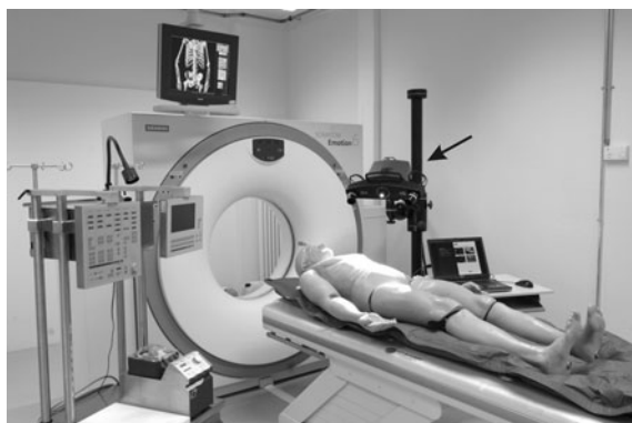
Fig. 5-12. Forensics laboratory with 3D surface scanner (arrowed) and CT scanner.
