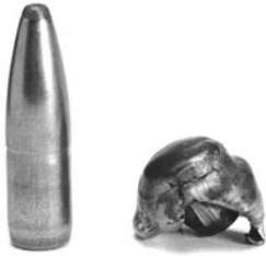
Fig. 3-11. Semi-jacketed bullet, calibre 7.62 \times 51 (308 Win.) and the deformed remains of the bullet after being fired into a soft medium.
