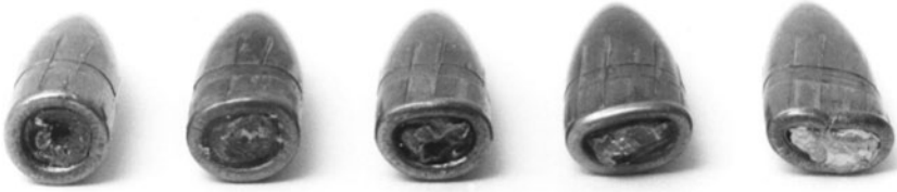
Fig. 3-29. Deformation of the tail of a bullet in gelatine as a function of impact velocity (KNEUBUEHL). From left to right: 600 m/s, 630 m/s, 670 m/s, 690 m/s and 710 m/s (7.62 × 39 bullet).
