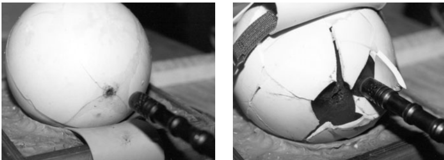
Fig. 5-28. (left) Near-contact shot into head model, fired from a 7.5 mm Stgw 57 assault rifle. Distance between muzzle and target: approx. 5 cm. The bullet has passed through cleanly, depositing little energy on the way. The fracture pattern corresponds to that observed in the real-life case.
