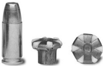
Fig. 4-18. Federal Expanding Full Metal Jacket, 9 mm Luger. Deformation in a simulant.
