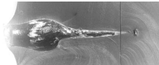
Fig. 4-15. Channel of a 44 Rem. Mag. fragmentation bullet in soap. Note the large fragment.
