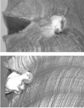
Fig. 4-54. A Bean Bag “non-lethal” 12-bore projectile. The bag containing lead shot weighs 40 g. At 5 m, it penetrated approximately 8 cm into soap (top), whereas at 7 m it penetrated only approximately 3.5 cm (bottom).
