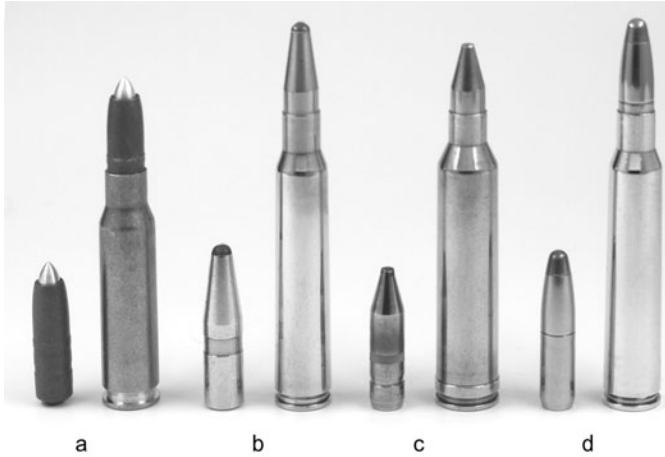
Fig. 2-23. Hunting cartridges and bullets: a. 308 Win. with Brenneke TAG, b. 7 × 64 with Hirtenberger ABC, c. 7 mm Rem. Mag. with RWS conical spitzer bullet, d. 7 × 64 with RWS partition bullet. Same scale as Figs. 2-20 and 2-21.
