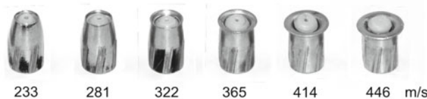
Fig. 3-35. A number of bullets from the experiment in Fig. 3-34, with the corresponding velocities.
