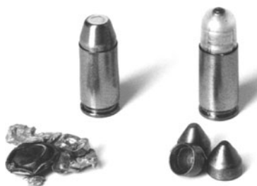
Fig. 4-16. Fragmentation bullets. Left: Velex explosive bullet (with fragments from simulant). Right: Triplex bullet. Both 9 mm Luger.
