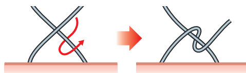
Fig. 3.2 Forming a half-hitch. Cross the threads and pass one end under the crossing to emerge on the other side.
