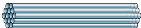
Fig. 4.27 A coherent bundle of glass fibres. They transmit light in a constant relationship within the fibres throughout the bundle.
