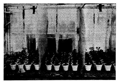
Fig. 1. Remote view showing bays 1, 2, 3, 5, 6, 7 and ion supply (emitter) heads as black objects above the *Exacum affine*, var. petite. Note wire mesh (grounded) isolating the bays from each other.
