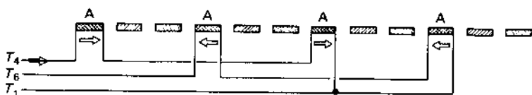
Fig. 4-91. The groups of the A phase are connected in series for four-pole operation at high speed. Constant H.P.
