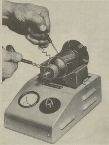
Fig. 6-77. An external growler. This is used for testing armatures for shorts, opens and grounds. (Crown Industrial Products)
