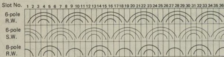
Fig. 2-50. A typical layout of coils in a two-speed capacitor-start motor.
