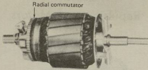
Fig. 3-4. A rotor having a radial commutator with bars perpendicular to the shaft. (Wagner Electric Company)
