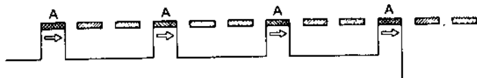
Fig. 4-87. Groups connected so that eight poles will be formed instead of four. All the arrows point in the same direction.
