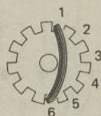
Fig. 9-21. View of the armature from the end opposite the commutator to determine the coil pitch.
