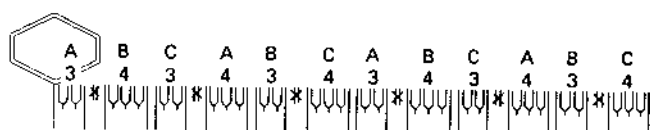
Fig. 4-107. Laying out groups for a three-phase, four-pole, 42-coil, series star (1Y) connection.
