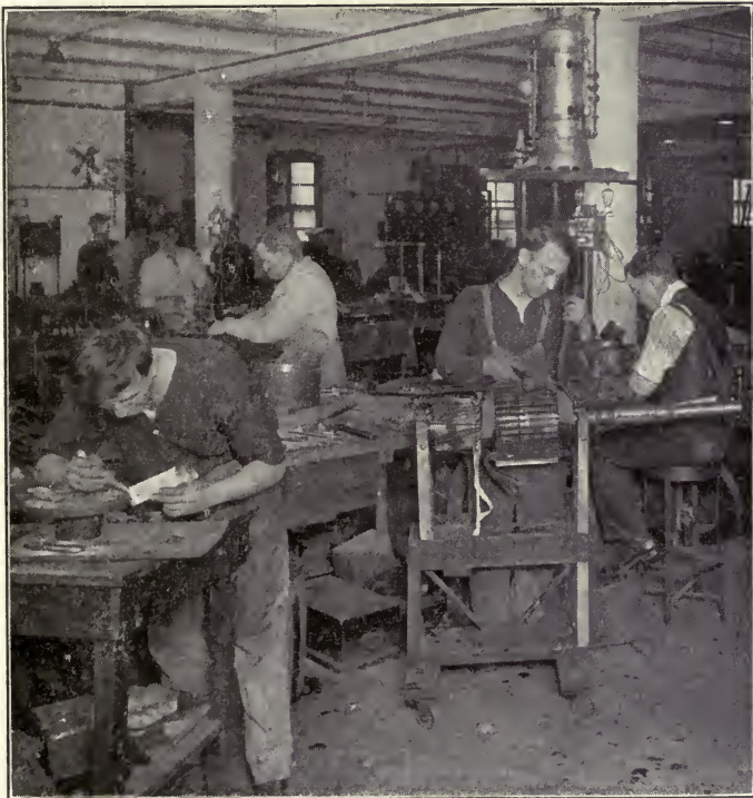
FIG. 72.—Portable floor stand for winding small direct-current armatures. The operator is shown shaping the end connections with a fiber drift.
