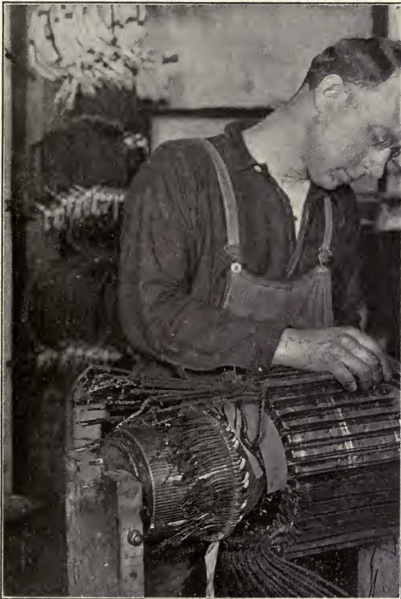
FIG. 91.—Inserting the top sides of coils in an armature. The leads of the bottom coil sides are shown connected to the commutator. Note the band of insulation between end connections.
