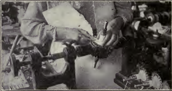
FIG. 57.—Winding the first coil in the slots of a small direct-current motor.
