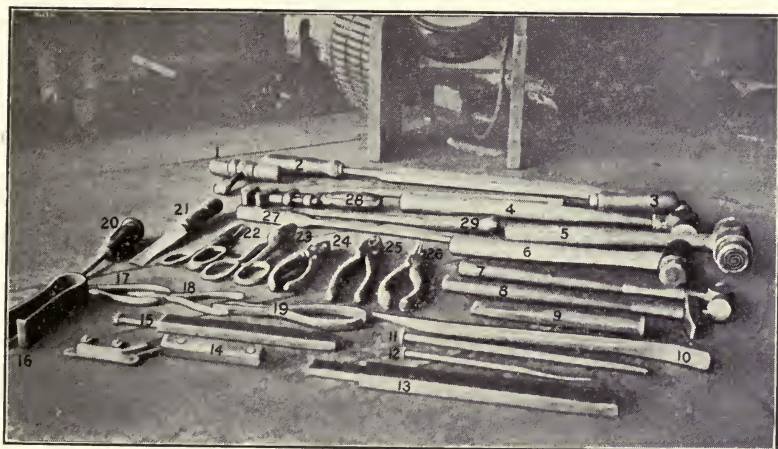
FIG. 275.—Armature winders' hand tools. (Numbers refer to their names and uses, page 446.)
