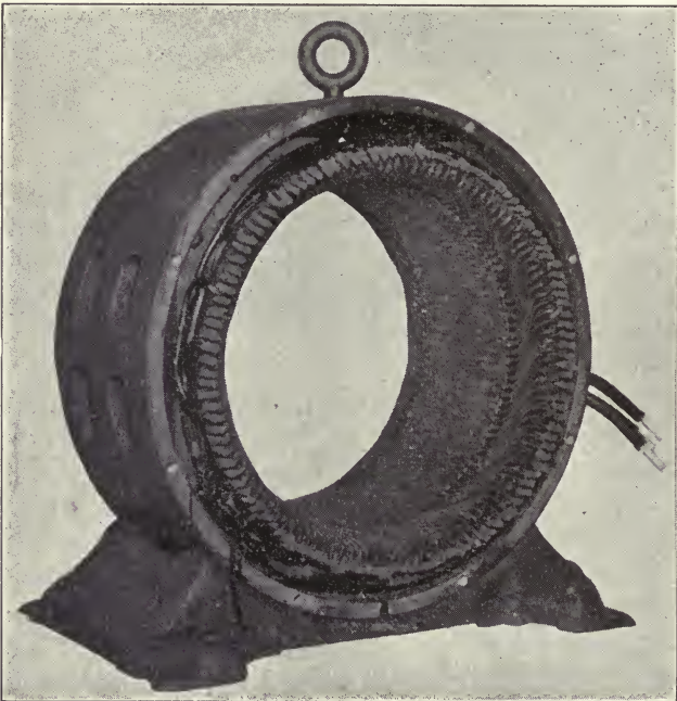
FIG. 188.—Stator of a 100-hp., 3-phase, 8-pole, 220-volt, 60-cycle, 120-coil, 120-slot, induction motor completely wound with pole-phase-groups properly cross connected.
