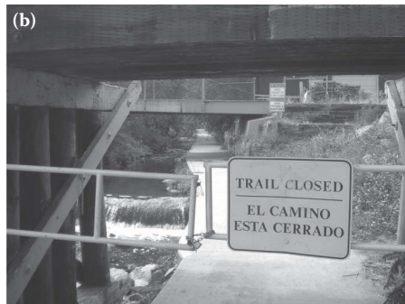
Figure 7.23 Public safety on and along urban floodplains. (a) Vertical and sloping composite drop and (b) trail between high banks without exit.
