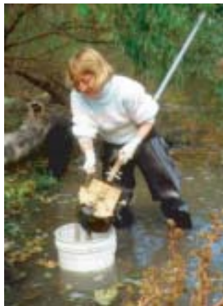
Figure 5.69 Collecting sediment with an Ekman dredge.
