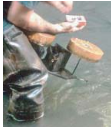
Figure 6.121 Diatometer for artificial substrate periphyton sampling.
