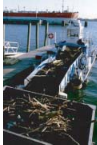
Figure 3.24 New York booms and skimmers for the control of floatable discharges.
