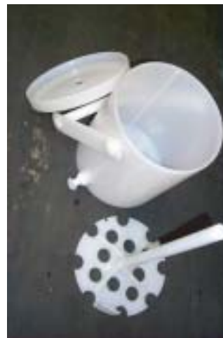
Figure 5.13 Churn splitter used to divide sample into individual bottles for separate preservative treatments and storage conditions, plus for preparing QA/QC split samples for independent analyses.
