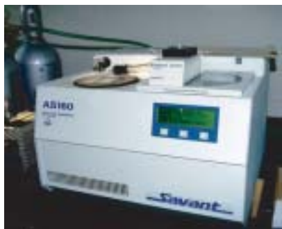
Figure E.20 Automatic vacuum/centrifuge concentrator (Savant AS 160).
