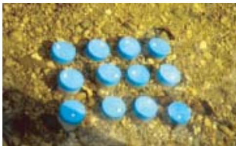
Figure 6.168 Chambers for conducting sediment bioaccumulation studies.
