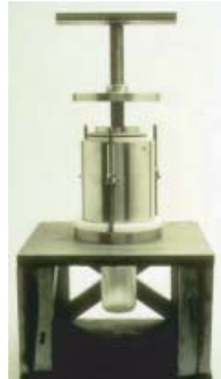
Figure 5.79 Pore water squeezer — stainless steel with Teflon liner.
