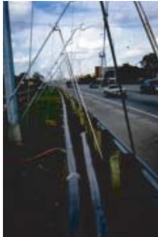
Figure 5.54. Sprinklers at freeway washoff test site in Austin, TX.
