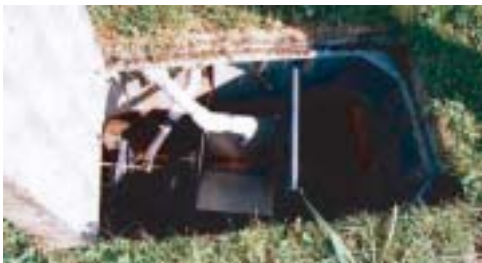
Figure 6.35 Tipping bucket flow measurement device for measuring groundwater flows at UW test plot.
