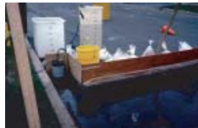
Figure 5.53. Runoff collection area for Toronto washoff tests.
