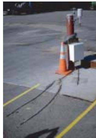
Figure 6.56 Pavement temperature monitoring by WI DNR.
