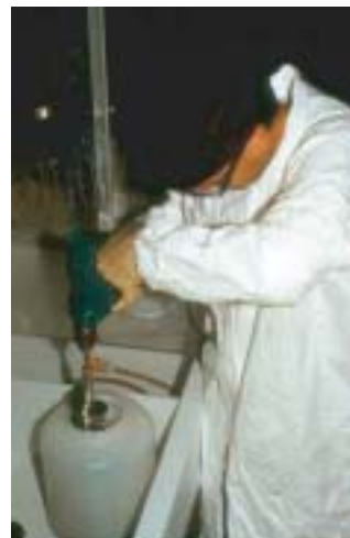
Figure 5.78 Mixing sediment with a drill auger.
