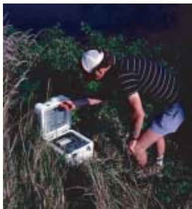
Figure 6.68 ° Older YSI DO meter for continuous monitoring. (Courtesy of Wisconsin Department of Natural Resources.)
