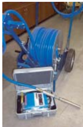
Figure 5.40 Grundfos Redi-Flo2 pump sampler with controller.
