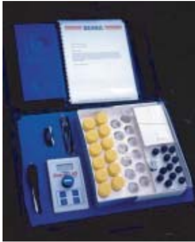
Figure 6.75 PetroFlag kit for field analyses of BTEX.
