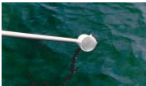
Figure 5.33 Manual dipper sampler.
