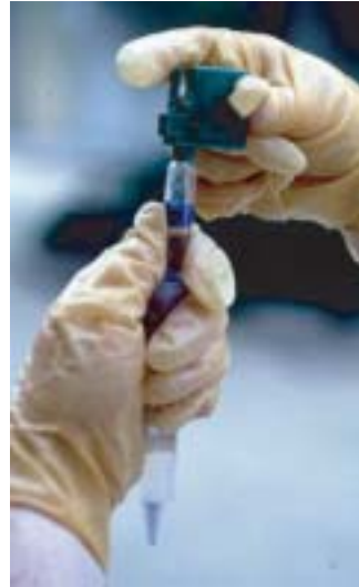
Figure 6.87° Extraction step 1 for use of the CHEMetrics detergent test kit.
