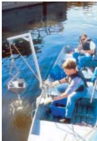
Figure 5.67 Winch with Ponar dredge.
