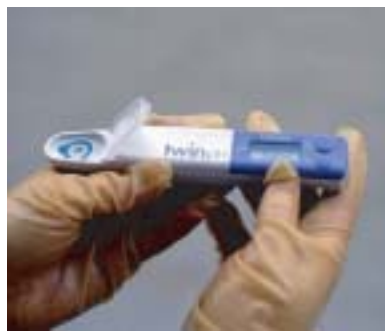
Figure 6.85 Horiba Twin pH meter reading sample.
