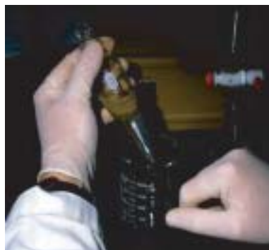
Figure E.17 Extract in centrifuge vial.
