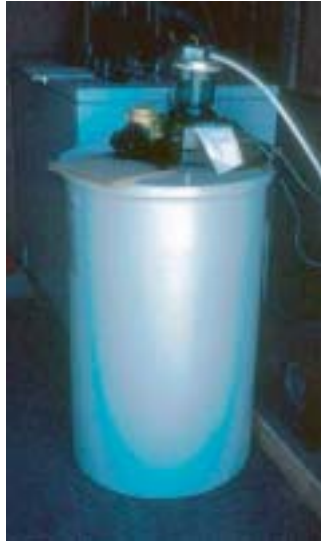
Figure 5.23 .Automatic sampler with large base for monitoring wide range of flows, with large chest freezer USGS discrete sampler in background, at Bellevue, WA.
