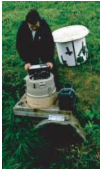
Figure 6.19 Automatic sampler at outfall at USGS flowmeter test site for collecting real-time dye samples for calibration of flowmeters.
