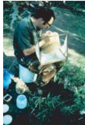
Figure 4.8 Removing benthic macroinvertebrate samples from Surber sampler.
