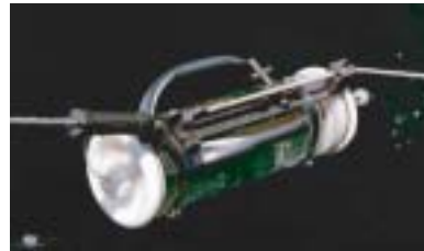
Figure 5.38 .Tripped vertical water sampler being withdrawn from water with messenger resting on trigger mechanism.
