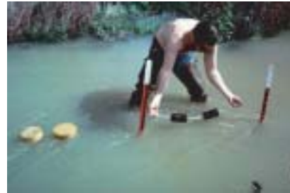
Figure 6.127 Periphyton sampler in place, plus Hester-Dendy samplers.
