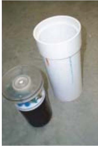
Figure 5.50 Prototype WI DNR/USGS automatic sheetflow sampler.
