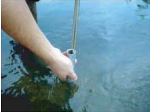
Figure 5.92 Placement of mini-piezometers into support tubing.
