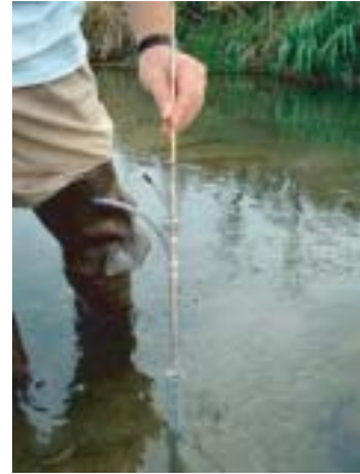
Figure 5.93 Placement of mini-piezometer array into sediments via temporary support pipe.
