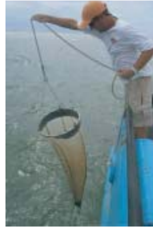
Figure 6.128 Net sampler for plankton.
