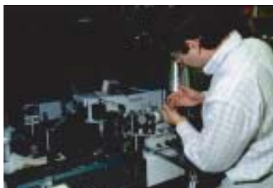
Figure 6.81 ° Laser fluorescence analysis of heavy metals being adapted for field analyses by UAB Physics Department.
