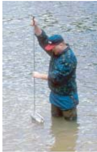
Figure 5.45 .Depth-integrated sediment sampler being readied for use.
