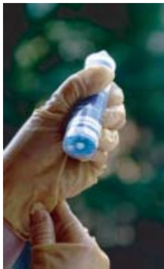
Figure 6.92° Reading the detergent concentration with the color comparator.
