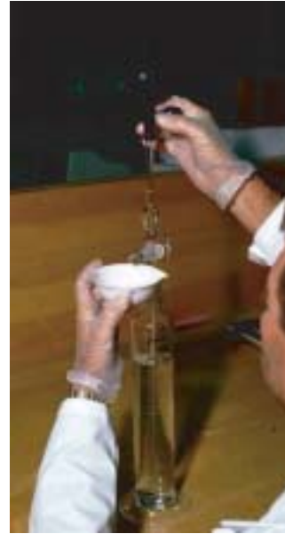
Figure 6.104 Andreason pipette for particle size determinations.
