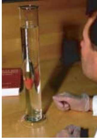
Figure 6.103 Hydrometer analyses for particle size determinations.
