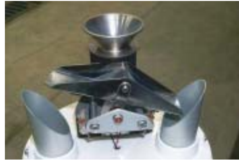
Figure 6.21 Close-up of tipping bucket rain gauge mechanism.
