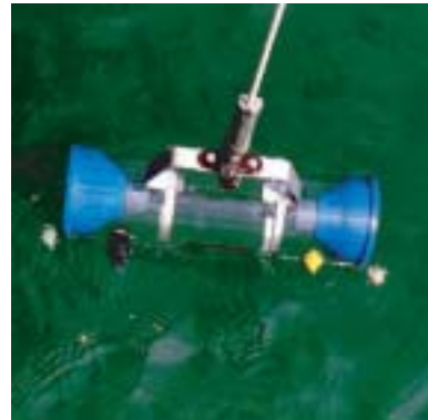
Figure 5.36 .Tripped horizontal water sampler being withdrawn from water with messenger resting on trigger mechanism.
