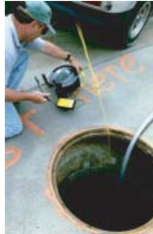
Figure 6.67 Petrosense used to measure hydrocarbons in manhole water.
