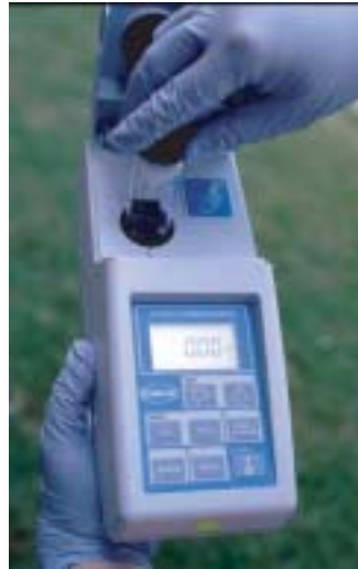
Figure 6.60 HACH 2100P field turbidimeter.
