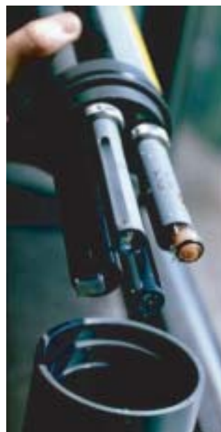
Figure 6.69 YSI 6000 sonde detail showing several probes.
