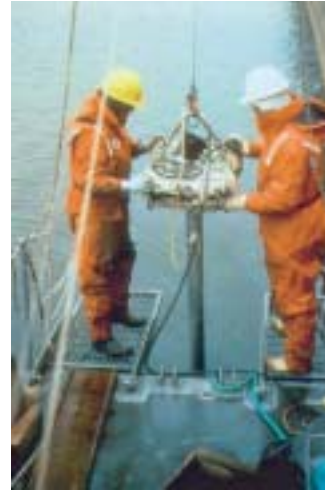
Figure 5.75 Lowering vibratory corer.
