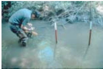
Figure 6.126 Periphyton sampler, two styrofoam floats with eight glass microscope slides in rack.
