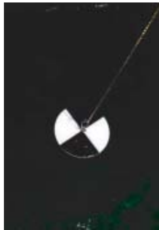
Figure 6.58 Secchi disk being lowered into lake for transparency measurement.
