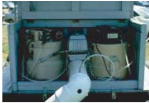
Figure 5.24 .Double monitor setup for simultaneously monitoring influent and effluent at small treatment device in Birmingham, AL.
