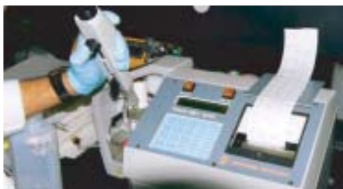
Figure E.11 Anodic stripping voltammeter (Outo kompku) for heavy metal analyses.
