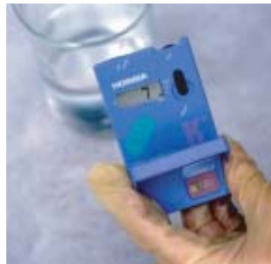
Figure 6.94 Horiba Cardy ion selection electrode for potassium.
