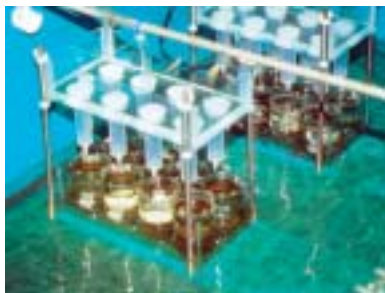
Figure 6.149 EPA whole sediment, overlying water renewal design.
