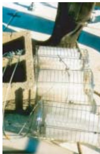
Figure 6.124 Artificial substrates (polyethylene mesh) in BBQ baskets secured to cinder blocks.
