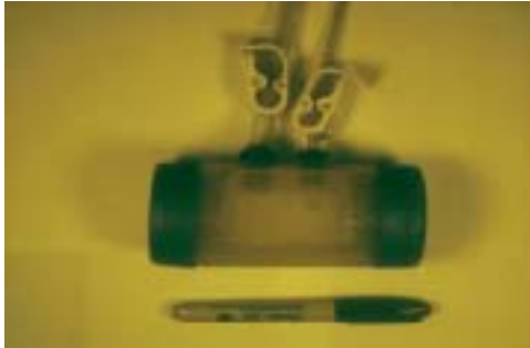
Figure 5.86 Medium-volume peeper with large aperture mesh for water sampling.
