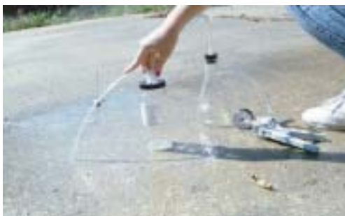
Figure 5.47 Sheetflow sampler operated by hand vacuum pump.
