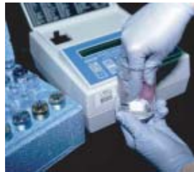
Figure 6.93 HACH AccuVac fluoride method.
