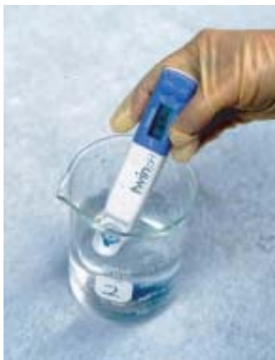
Figure 6.84 Horiba Twin pH meter dipped in sample.
