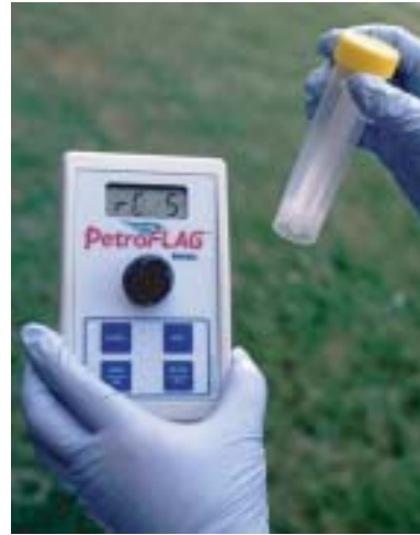
Figure 6.76 Sample being read using PetroFlag.
