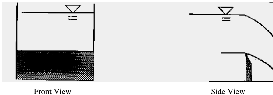
Fig. 2.8 Sharp crested weir installed in a rectangular channel
