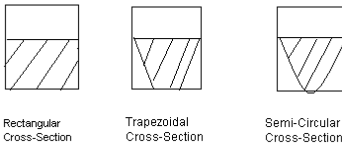
Fig.9.3 Types of Channel Cross Sections
