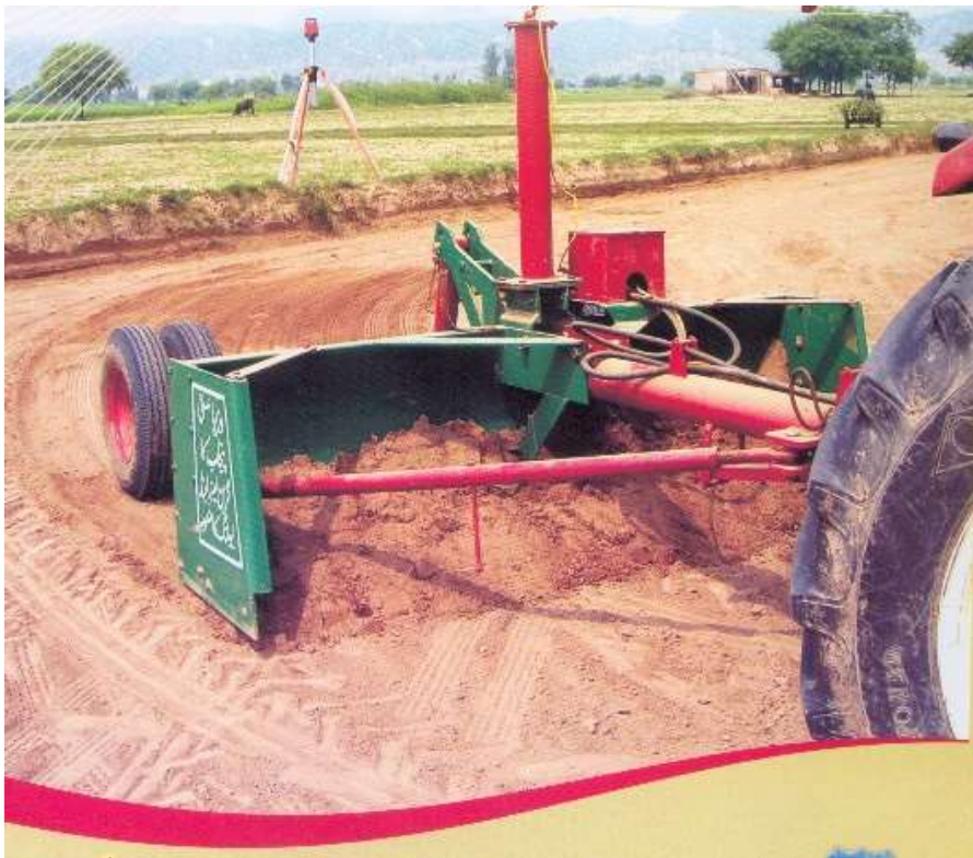
Fig. 8.13 Scraper Mast and Hydraulic System in Laser Land Leveling
