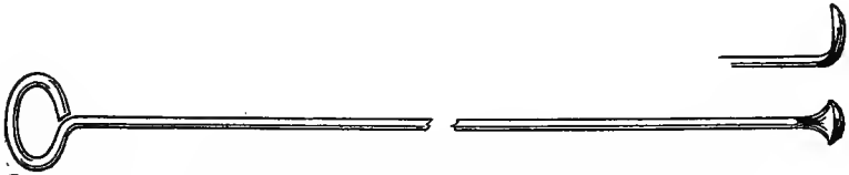
FIG. 5. A GOOD TYPE OF SPOON FOR CLEANING OUT THE BOTTOMS OF BORE HOLES
