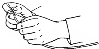
3. Slip cap on end of fuse.
