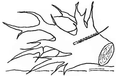
FIG. 25. LOCATION OF A HOLE BORED INTO A PULLED STUMP FOR SPLITTING. SOME PREFER TO BORE SUCH A HOLE IN THE SAME DIRECTION AS THE NATURAL HOLLOW (FIG. 24)
