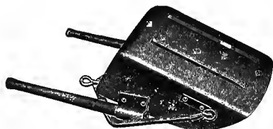
FIG. 78. DRAG SCRAPER SUITABLE FOR MOVING BLASTED GROUND IN FINISHING FISH PONDS, GRADING ROADS, FILLING GULLIES, AND DOING MANY OTHER CLASSES OF WORK
