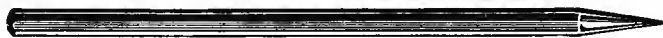
FIG. 45. PUNCH FOR MAKING THE BORE HOLES. THIS IS DRIVEN WITH A HEAVY HAMMER (See page 19)
