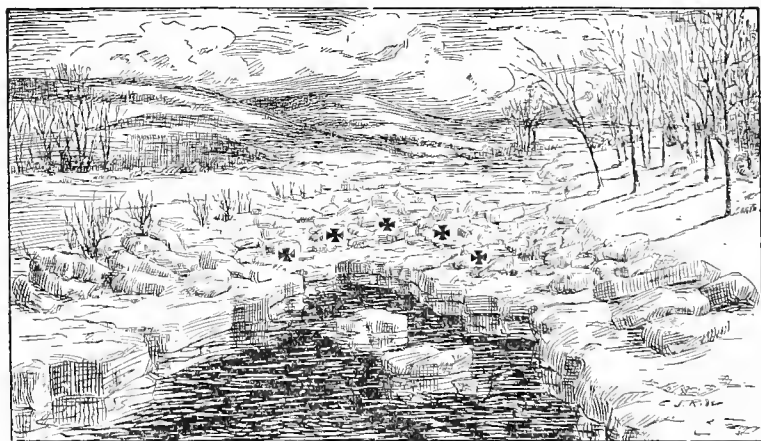
FIG. 76. DIAGRAM SHOWING LOCATION OF ROW OF HOLES FOR BLASTING AN ICE GORGE
