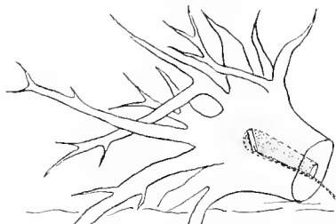
FIG. 24. SHOWING LOCATION OF A CHARGE OF EXPLOSIVES IN A HOLLOW-PULLED STUMP
