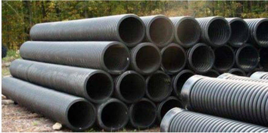
Fig. 9.3. High-density polyethylene (HDPE) drain pipes.
