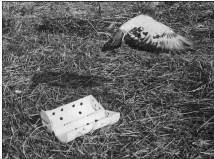
When the halves spring apart, the hinged edges throw the bird into the air. Leon's launchers accommodate one pigeon or two quail.
