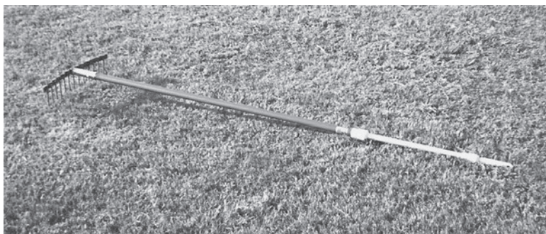
Figure 29.10 Lake and aquatic rakes, though expensive, are available for sale. Fishing nets and butterfly nets can also be helpful but have their own limitations, such as the strength of the net when trying to recovery something covered in silt or dirt or by collecting underwater life. This “cadaver rake,” created over 20 years ago, has been used by many agencies. It is an extendible pool-cleaning pole with a piece of slightly curved metal and tenpenny nails attached.
