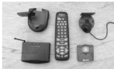
FIG. 4.7. Motion-activated remote video system. Inexpensive video devices are available to record a dog's separation activities throughout the day. A motion-sensitive infrared detector turns on a remote VCR and turns it off again after a short period. A similar device could be devised to activate an air-pump odor dispenser and feeder described in Chapter 3 (see Systematic Desensitization , Figure 3.5).
