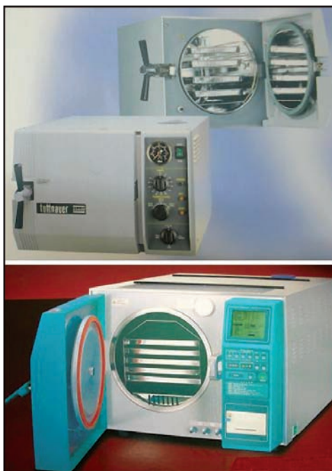
Fig. 7.2: Hot air sterilizer with automatic control of temperature 0 degree to 200 degrees
