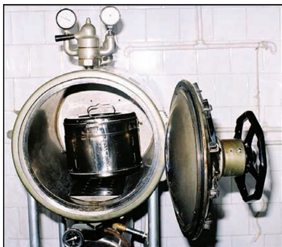
Fig. 7.1A(2): Autoclave with door open. Inside drums, trays can be kept with the material to be sterilized
