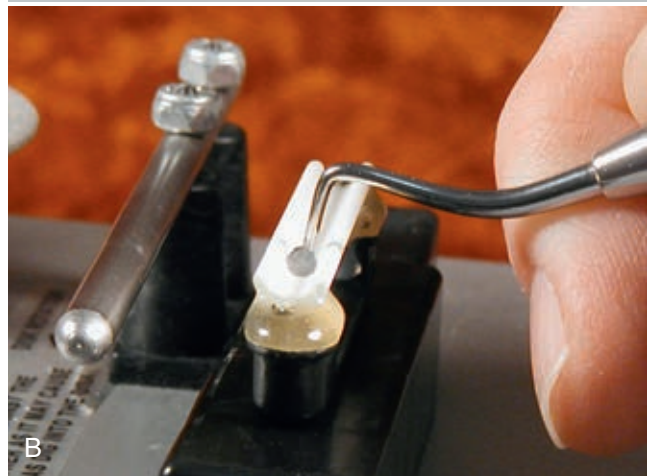
Online Fig. 23-1 A , The Rx Honing Machine shown is used as mechanical sharpener for many different types of dental instruments. It has two spindle drives, one clockwise and the other counterclockwise, to which can be mounted different types of disks and hones to polish and sharpen various types of dental instruments. B , The RX Honing Machine shown using a ceramic hone to sharpen a Black spoon dental instrument to extend the life of the instrument.
