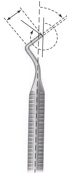
Fig. 6-3 Instrument shank and blade design (with primary cutting edge positioned close to handle axis to produce balance). The complete instrument formula (four numbers) is expressed as the blade width (1) in 0.1-mm increments, cutting edge angle (2) in centigrades, blade length (3) in millimeters, and blade angle (4) in degrees.
