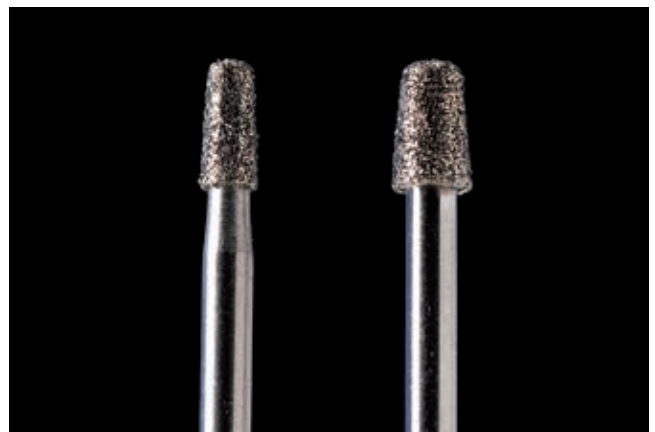
Fig. 11-12 Typical diamond rotary instruments used for ceramic inlay or onlay tooth preparations.
