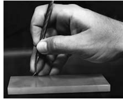
Online Fig. 23-2 Sharpening an instrument. Maintaining the proper angle of bevel and angle of the cutting edge to the stone is aided by resting the fingertips on the stone.
