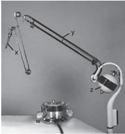
Online Fig. 23-10 Typical equipment when an electric motor is used as the source of power: foot control with rheostat (w), belt-driven straight handpiece (x), three-piece adjustable extension arm (y), and electric motor (z).
