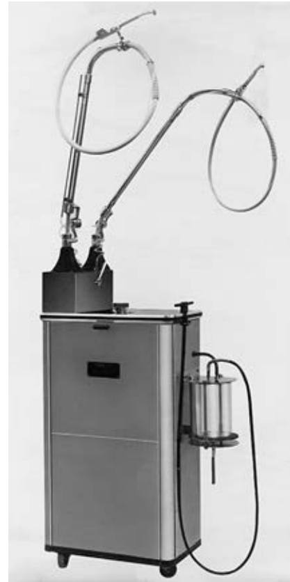
Online Fig. 23-12 Turbo-Jet portable unit (circa 1955). A small turbine in the head of the angle handpiece is driven by water circulated by a pump housed in the mobile base.
