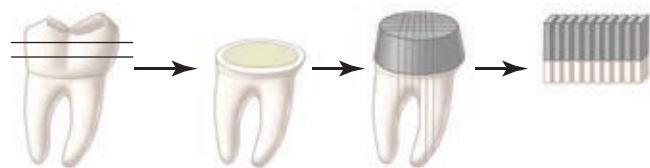
Fig. 4-25 Preparation of specimens for microtensile bond strength testing.
