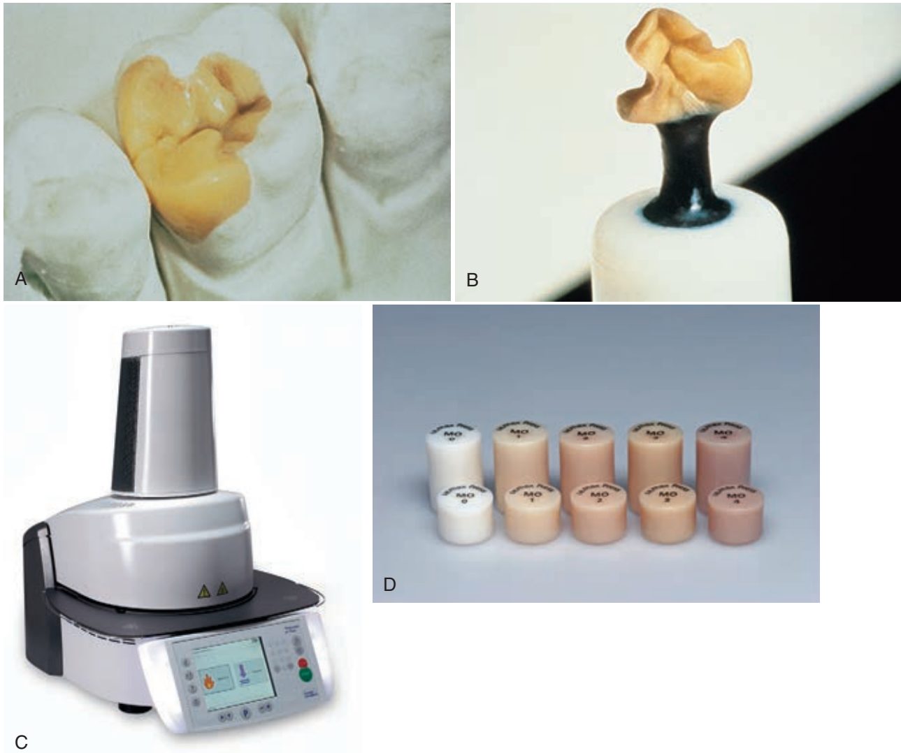
Fig. 11-4 Fabrication of a pressed ceramic onlay. A , Wax pattern. B , Wax pattern on sprue base, ready to be invested. C , Device for pressing heated ceramic (Programat EP 5000). D , Selection of ceramic ingots used for forming the restoration. (Courtesy of Ivoclar Vivadent Inc., Amherst, NY.)
