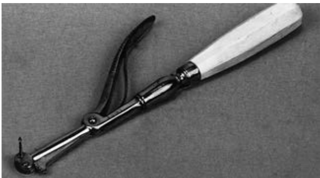
Online Fig. 23-8 Early angle hand drill for indirect access preparations (circa 1850). The bur is activated by squeezing the spring-loaded handle.
