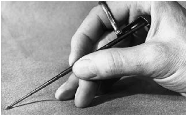
Online Fig. 23-7 Early straight hand drill for direct access preparations (circa 1800). The back end of the bur shank fits into a finger ring while the front end is rotated with the thumb and the forefinger.
