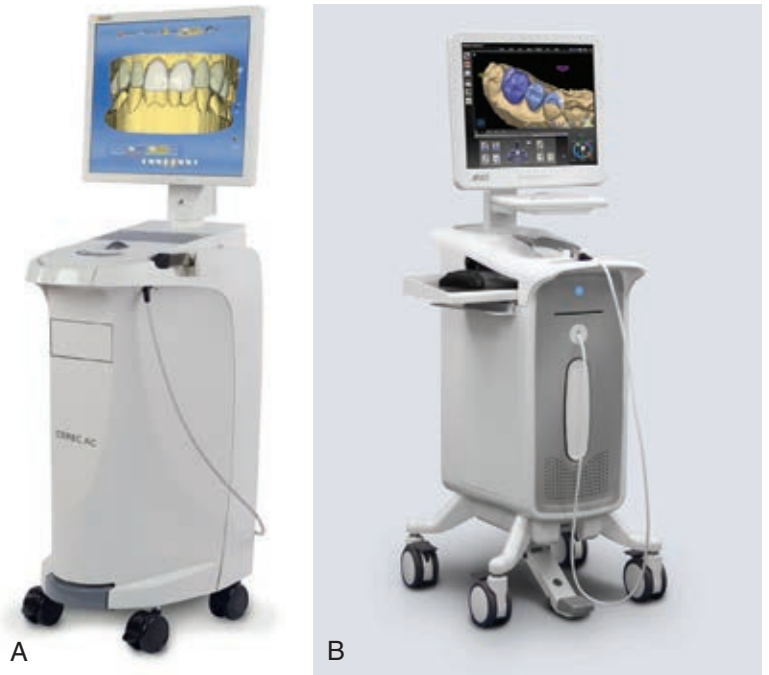
Fig. 11-5 CEREC AC (A) and E4D (B) computer-aided design/computer-assisted manufacturing (CAD/CAM) devices. These chairside units are compact and mobile. (A, Courtesy Sirona Dental Systems LLC, Charlotte, NC. B, Courtesy D4D Technologies, LLC, Richardson, TX.)
