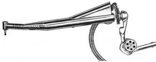
Online Fig. 23-11 Page-Chayes handpiece (circa 1955). The first belt-driven angle handpiece to operate successfully at speeds greater than 100,000 rpm (revolutions per minute).
