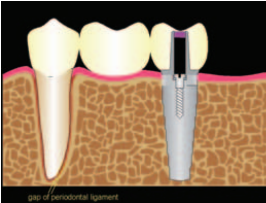
Figure 15.4a. Scheme of tooth-implant connected bridge. The gap of the periodontal ligament allows a damped anchorage.
