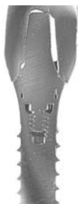
Figure 16.9. A single-stage or transmucosal-type dental implant in cross-section. This is a specimen prepared for laboratory testing and was not used clinically. Note that the crown rests on the external shoulder of the implant body. Load transfer from the occlusal table to the implant is focused on this external shoulder, resulting in inward compressive forces rather than externally directed hoop stresses. This implant design may provide superior resistance to fatigue fracture in areas of heavy occlusal load. This design also provides abutment retrievability and may be used for screw-retained or cement-retained reconstructions.
