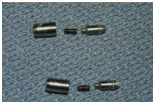
Figure 16.3. Fractured abutment screws from an external hex implant restoration. The cause of failure was most likely fatigue fracture resulting from loss of preload across the bolted implant to abutment joint.
