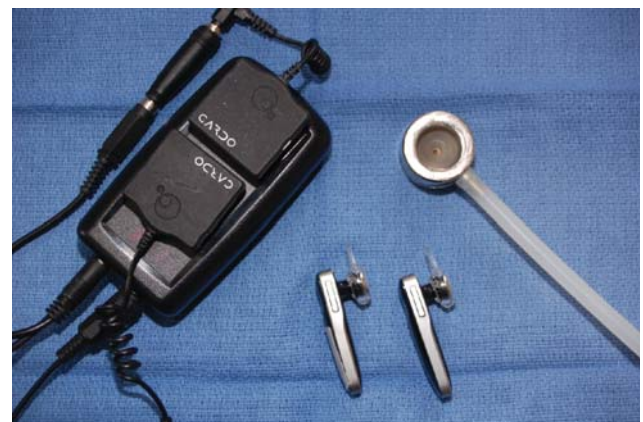
Figure 24.1 A pre-tracheal stethoscope fitted with two headsets, so that both doctor and assistant can monitor airway noise simultaneously.
