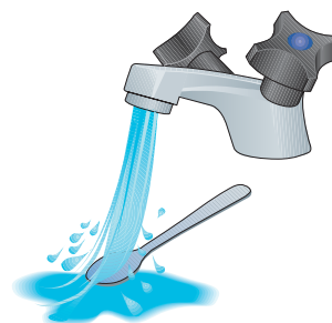
Fig. 6.1.4 Heat transfer by convection. Example: The spoon is rinsed in running cold water. Heat is absorbed by the water and the spoon gets cooler, until the spoon and the water are at the same temperature.
