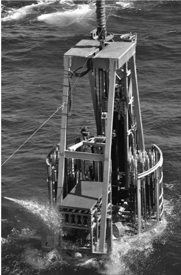
Figure 11.4 Remotely controlled seafloor drilling rig for sampling and in situ testing. (Designed and built by Gregg Marine, Moss Landing, CA, and reproduced with permission.)
