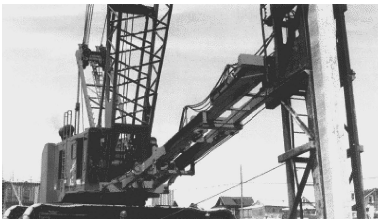
Figure 3.3 ICE 225 spotter with optional front lead rotation. (Courtesy of International Construction Equipment, Charlotte, NC.)
