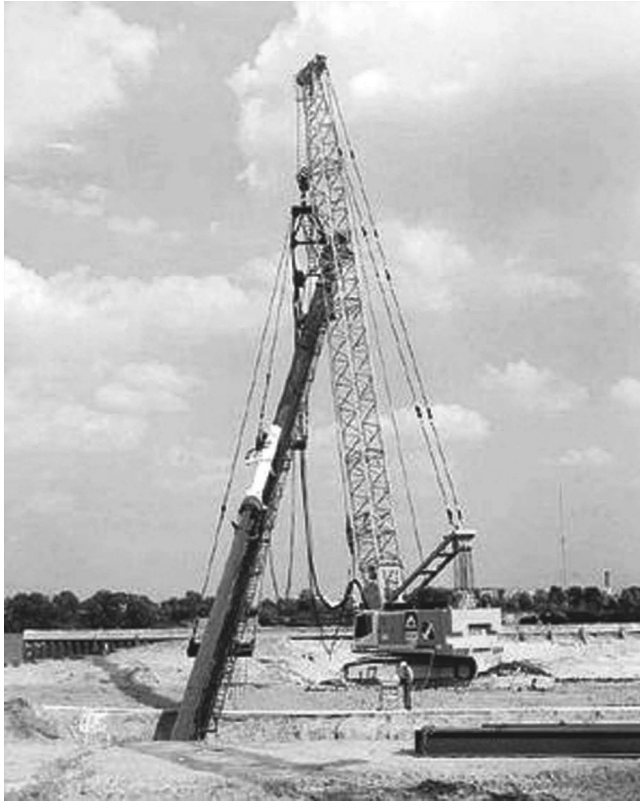
Figure 3.4 Liebherr LRH 400 48 m long swinging leader on HS 885 HD crane. (Courtesy of Liebherr Great Britain Ltd, Biggleswade, UK.)
