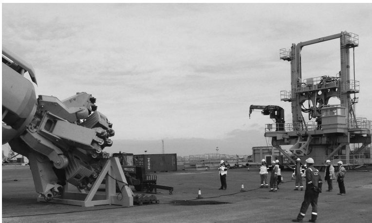
Figure 3.31 LDD reverse-circulation drill bit 4.3 m diameter with expandable under-reamers to maximum 6 m for drilling inside and below tapered piles. (Courtesy of Large Diameter Drilling Ltd, Penryn, UK.)
