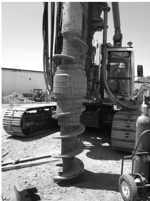
Figure 2.29 Omega displacement pile auger. (Courtesy of Malcolm Drilling Company, San Francisco, CA.)
