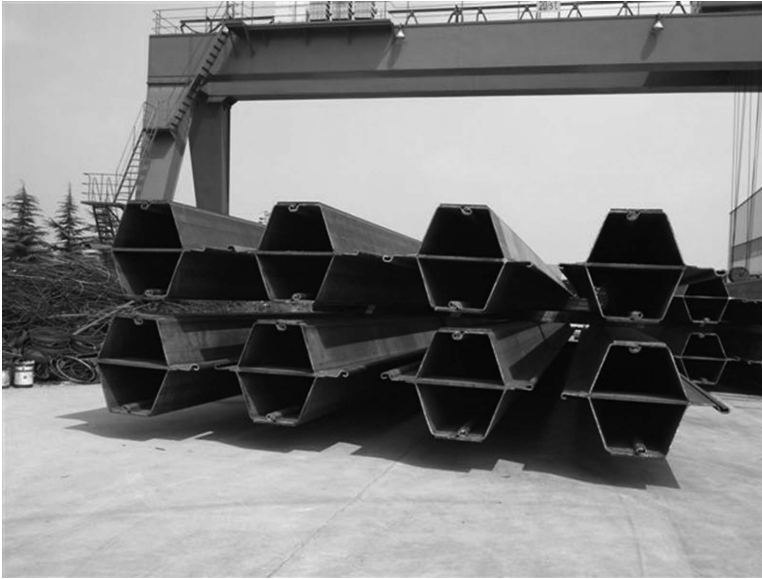
Figure 2.15 Box piles using Z-sheet pile sections in fabrication yard. (Courtesy of Maxx Piling Ltd., Shenfield, UK.)
