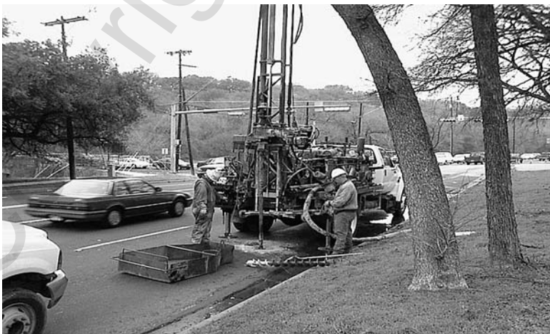
Figure 4.2 A typical drilling machine and its associated equipment.
