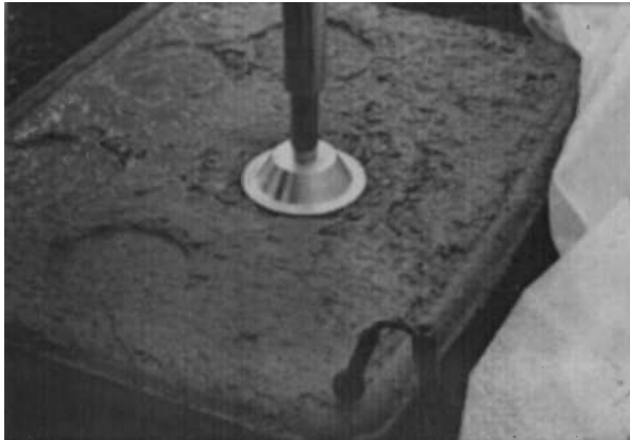
Fig. 6—Finisher’s foot apparatus being using on a concrete slab to determine penetration resistance (after Abel and Hover [6]).
