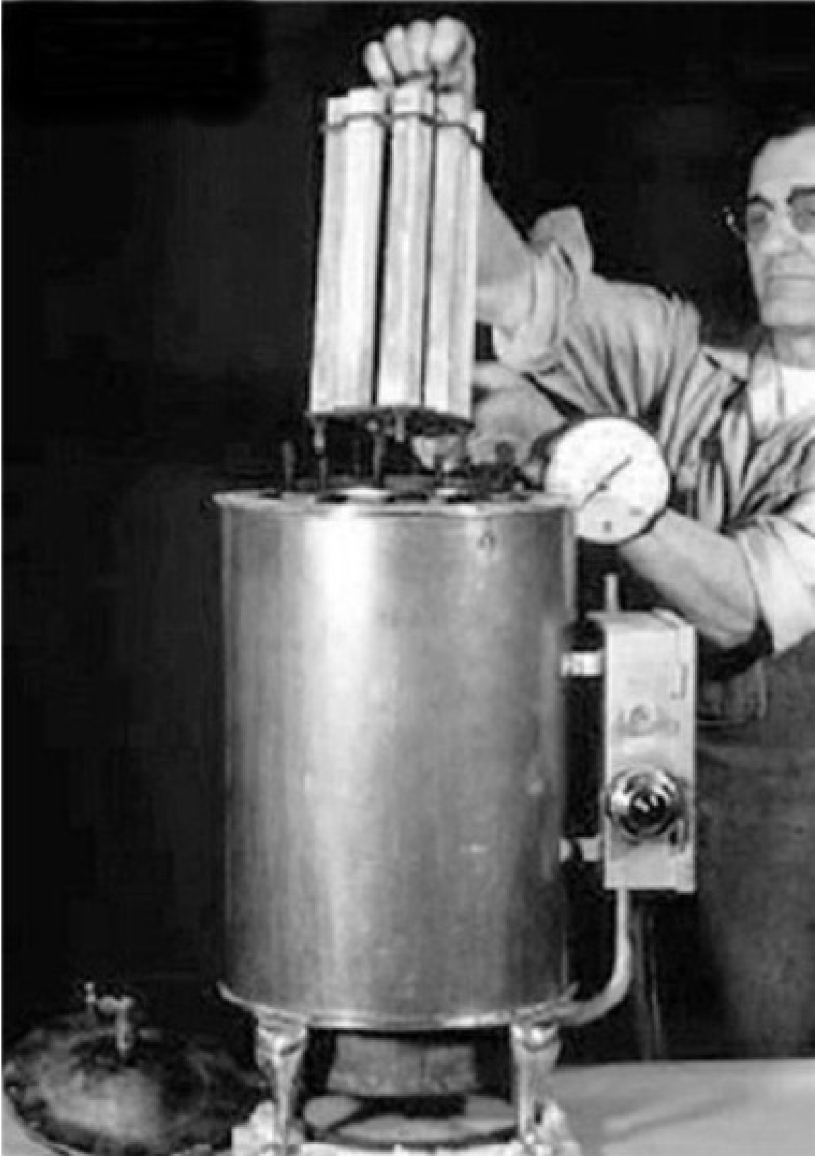
Fig. 4—Autoclave expansion apparatus and specimens (reprinted with permission from Ref 7).
