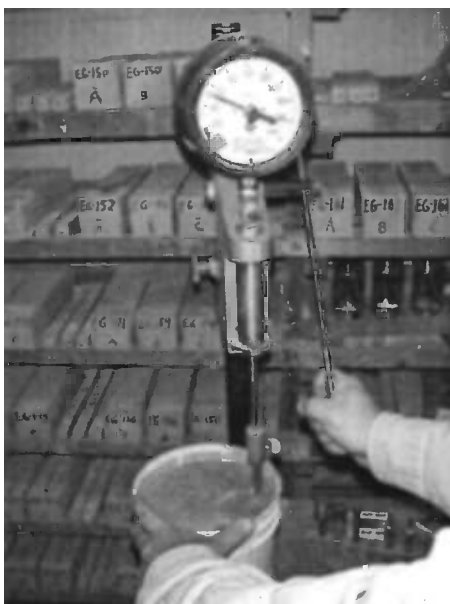
Fig. 1—One style of bench-top penetrometer used to perform the ASTM C 403/C 403M method.
