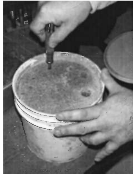
Fig. 2—Pocket penetrometer used to perform the ASTM C 403/C 403M method when a bench-top style is not available.
