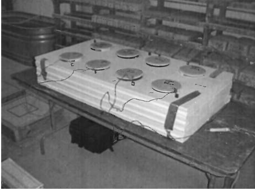
Fig. 11—Insulating chamber with cavities for concrete specimens used in proposed thermal method. Thermocouple tips are imbedded in the base of the cavity.
