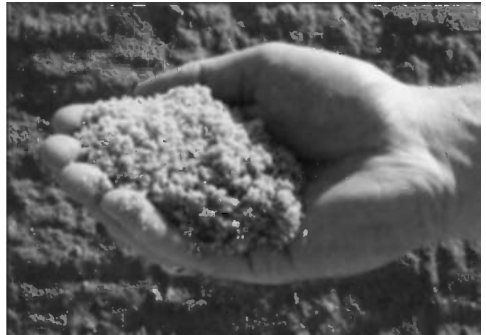
Fig. 5 —Slag granules in a stockpile (background) waiting to be finely ground into slag cement.
