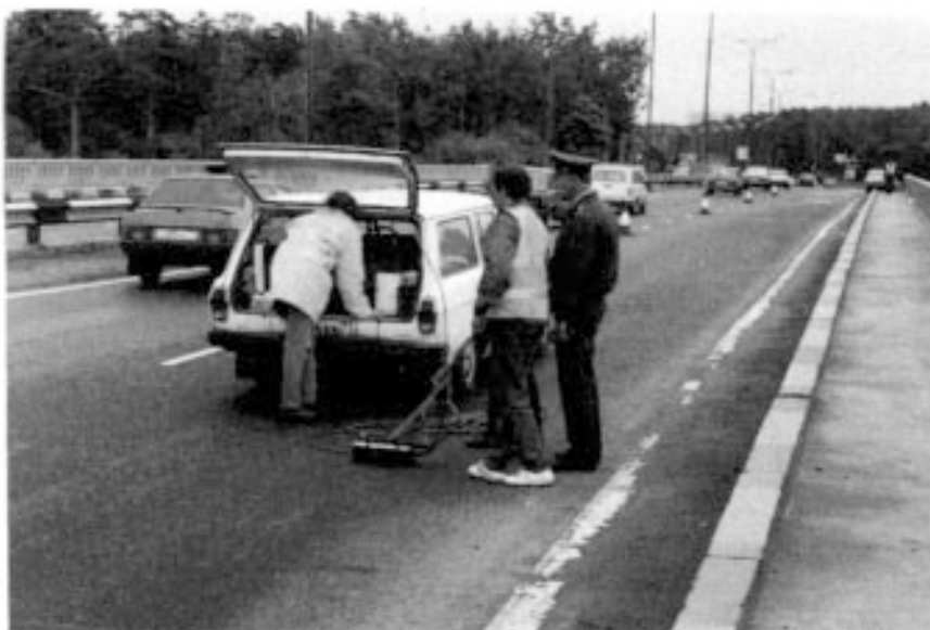
Figure 6.6 Impulse radar survey on Khimkinski Bridge, Moscow. Courtesy, GB Geotechnics.
