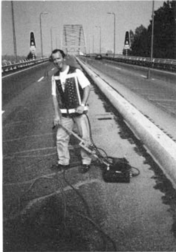
Figure 6.5 Impulse radar survey on Papendrecht Bridge, Netherlands. Courtesy, GB Geotechnics.
