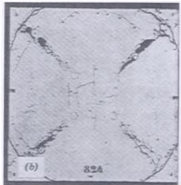
Figure 7.74 Yield line pattern at failure of simple supported uniformly loaded square slabs: 7.2 (a) bottom surface; (b) top surface.
