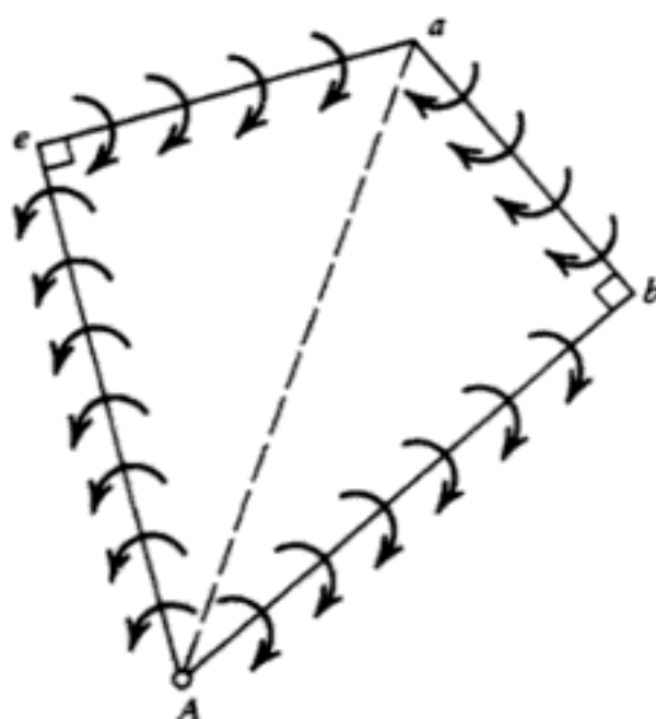
Figure 6.39 Bending moments acting on edges of trapezium shaped element.
