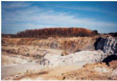
Fig. 2-6. Limestone, a primary raw material providing calcium in making cement, is quarried near the cement plant. (IMG12437)
