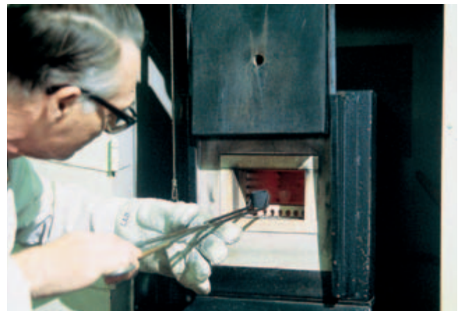
Fig. 2-46. Loss on ignition test of cement. (IMG12305)
