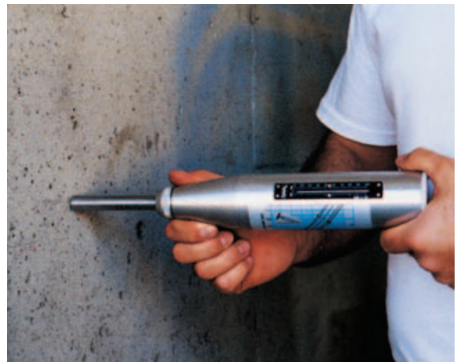
Fig. 16-20. The rebound hammer gives an indication of the compressive strength of concrete. (IMG12176)
