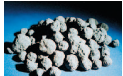
Fig. 2-9. Portland cement clinker is formed by burning calcium and siliceous raw materials in a kiln. This particular clinker is about 20 mm (% in.) in diameter. (IMG12434)
