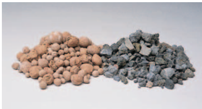
Fig. 5-3. Lightweight aggregate. Expanded clay (left) and expanded shale (right). (IMG12186)
