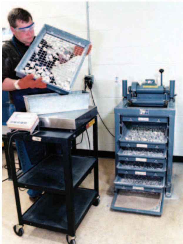
Fig. 5-5. Making a sieve analysis test of coarse aggregate in a laboratory. (IMG15129)
