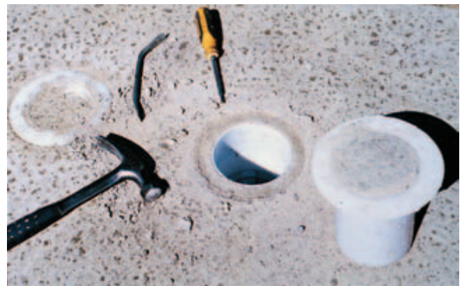
Fig. 16-13. Concrete cylinders cast in place in cylindrical molds provide a means for determining the in-place compressive strength of concrete. (IMG12175)
