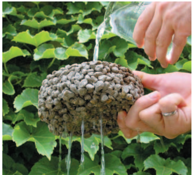
Fig. 18-14. Pervious concrete's key characteristic is the open-pore structure that allows high rates of water transmission.
