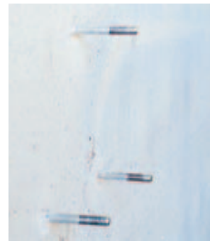
Fig. 16-22. The Windsor-probe technique for determining the relative compressive strength of concrete.
