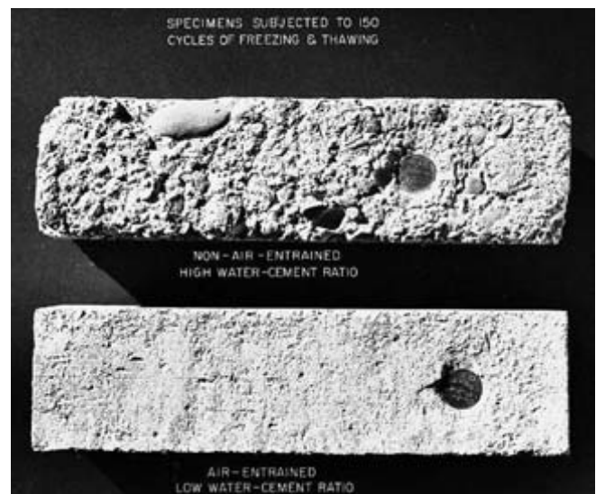
Fig. 1-25. Air-entrained concrete (bottom bar) is highly resistant to repeated freeze-thaw cycles. (IMG12294)
