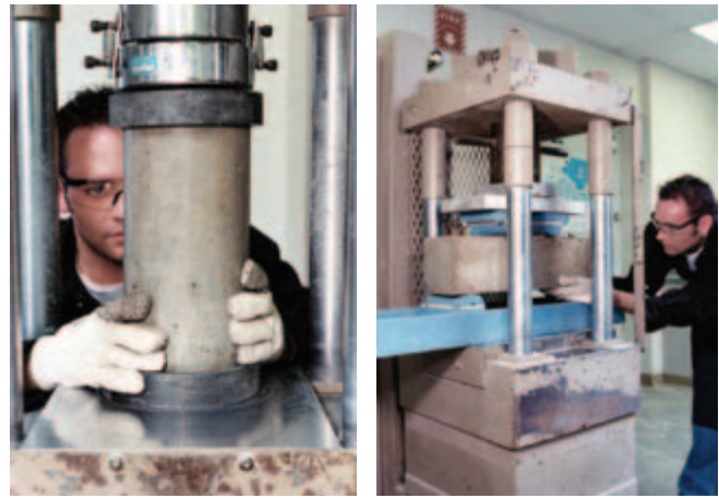
Fig. 16-15. Testing hardened concrete specimens: (left) cylinder, (right) beam (IMG15126, IMG15127).
