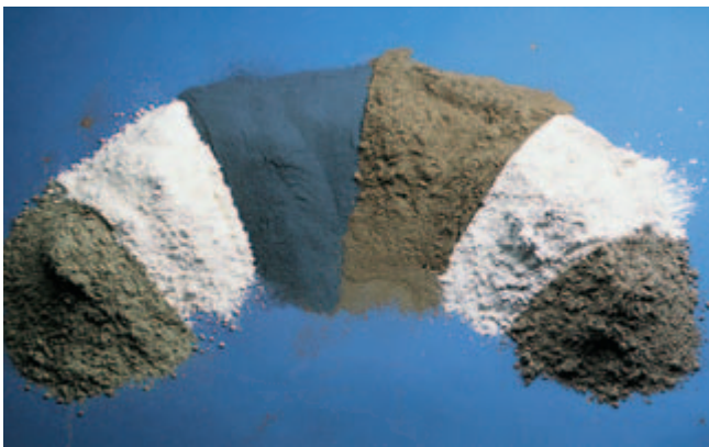
Fig. 3-1. Supplementary cementitious materials. From left to right, fly ash (Class C), metakaolin (calcined clay), silica fume, fly ash (Class F), slag, and calcined shale. (IMG12187)
