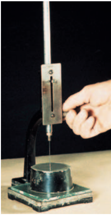
Fig. 2-38. Time of set test for paste using the Vicat needle. (IMG12502)
