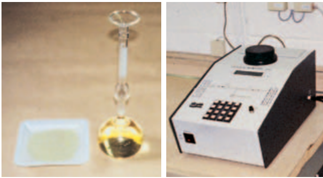
Fig. 2-47. Density of cement can be determined by (left) using a Le Chatelier flask and kerosine or by (right) using a helium pycnometer. (IMG12446, IMG12445)
