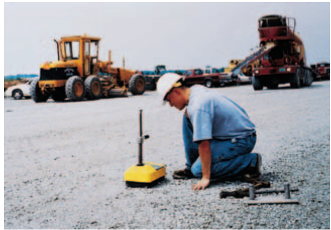
Fig. 11-15. Nuclear gauges containing radioactive sources used to measure soil density and moisture can determine if a subbase has been adequately compacted. (IMG12384)
