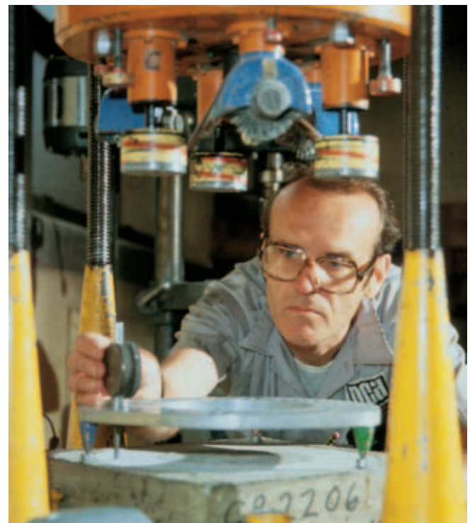
Fig. 1-24. Test apparatus for measuring abrasion resistance of concrete. The machine can be adjusted to use either revolving disks or dressing wheels. With a different machine, steel balls under pressure are rolled over the surface of the specimen. The tests are described in ASTM C779. (IMG12293)
