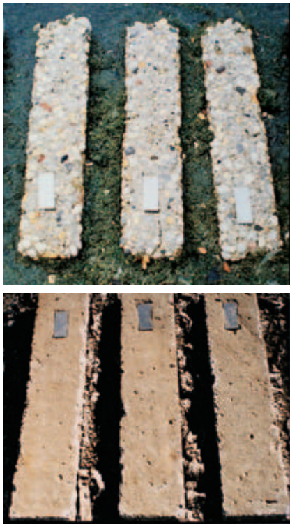
Fig. 2-15. Specimens used in the outdoor sulfate test plot in Sacramento, California, are 150 x 150 x 760-mm (6 x 6 x 30-in.) beams. A comparison of ratings is illustrated: (top) a rating of 5 for 12-year old concretes made with Type V cement and a water-to-cement ratio of 0.65; and (bottom) a rating of 2 for 16-year old concretes made with Type V cement and a water-to-cement ratio of 0.39 (Stark 2002). (IMG12481, IMG12480)
