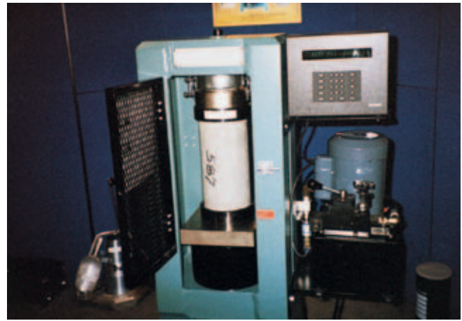
Fig. 1-18. Testing a 150 x 300-mm (6 x 12-in.) concrete cylinder in compression. The load on the test cylinder is registered on the display. (IMG12500)
