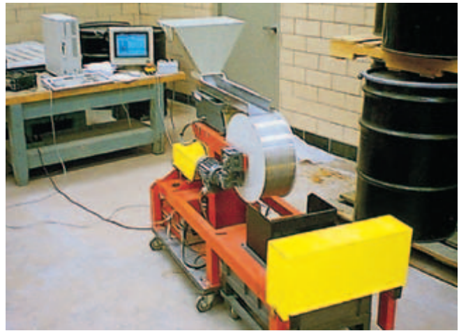
Fig. 5-11. Videograder for measuring size and shape of aggregate. (IMG12424)
