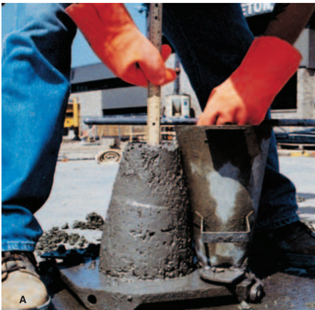
Fig. 16-2. Slump test for consistency of concrete. Figure A illustrates a lower slump, Figure B a higher slump. (IMG12179, IMG12180)
