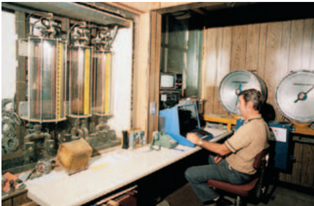
Fig. 6-20. Liquid admixture dispenser at a ready mix plant provides accurate volumetric measurement of admixtures. (IMG12323)
