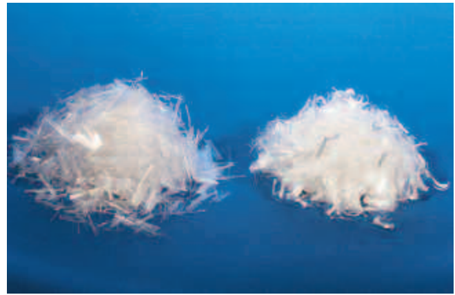
Fig. 7-7. Polypropylene fibers are produced either as (left) fine fibrils with rectangular cross section or (right) cylindrical monofilament. (IMG12403)
