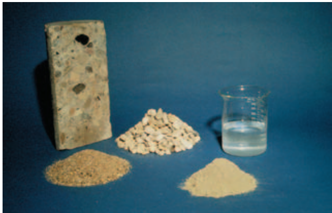
Fig. 1-1. Concrete components: cement, water, fine aggregate and coarse aggregate, are combined to form concrete. (IMG12501)
