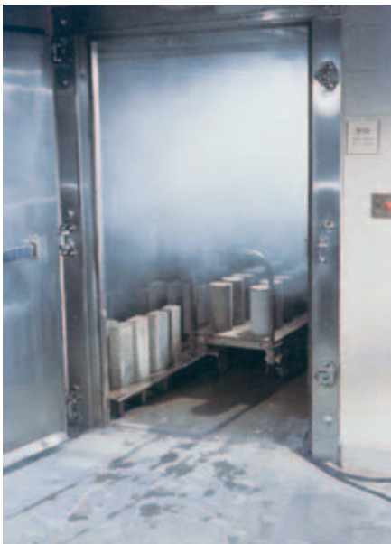
Fig. 16-9. Controlled moist curing in the laboratory for standard test specimens at a relative humidity of 95% to 100% and temperature of 23 \pm 2^\circ\text{C} ( 73 \pm 3^\circ\text{F} ) (ASTM C511 or AASHTO M 201). (IMG12346)
