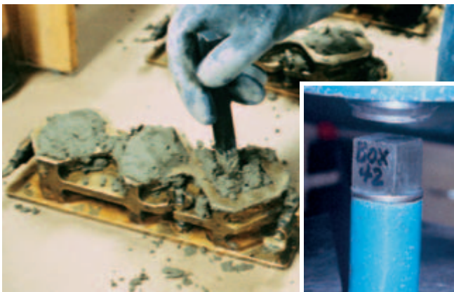
Fig. 2-41. 50-mm (2-in.) mortar cubes are cast (left) and crushed (right) to determine strength characteristics of cement. (IMG12450, IMG12449)
