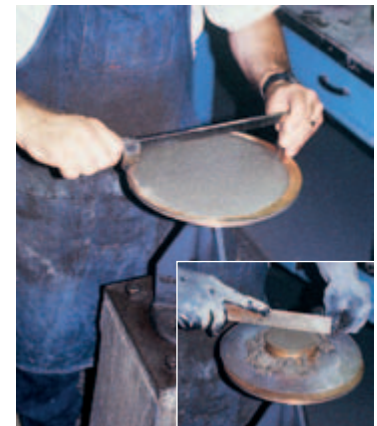
Fig. 2-37. Consistency test for mortar using the flow table. The mortar is placed in a small brass mold centered on the table (inset). For skin safety the technician wears protective gloves while handling the mortar. After the mold is removed and the table undergoes a succession of drops, the diameter of the pat is measured to determine consistency. (IMG12453, IMG12452)
