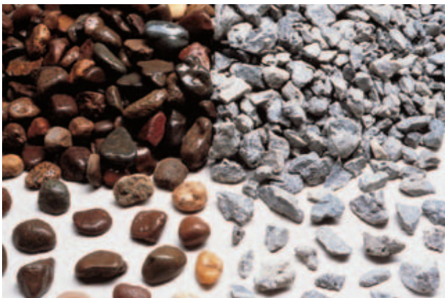
Fig. 5-2. Coarse aggregate. Rounded gravel (left) and crushed stone (right). (IMG12184)
