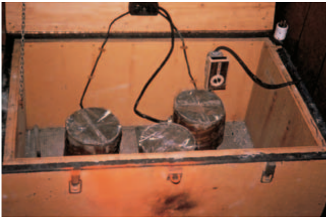
Fig. 14-15. Insulated curing box with thermostat for curing test cylinders. Heat is supplied by electric rubber heating mats on the bottom. A wide variety of designs are possible for curing boxes. (IMG12268)
