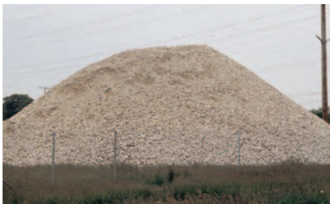
Fig. 5-26. Stockpile of recycled-concrete aggregate. (IMG12219)
