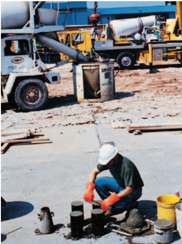
Fig. 16-7. Preparing standard test specimens for compressive strength of concrete. (IMG12183)
