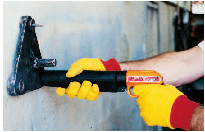
Fig. 16-22. The Windsor-probe technique for determining the relative compressive strength of concrete.
