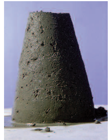
Fig. 1-10. Concrete of a stiff consistency (low slump). (IMG12291)
