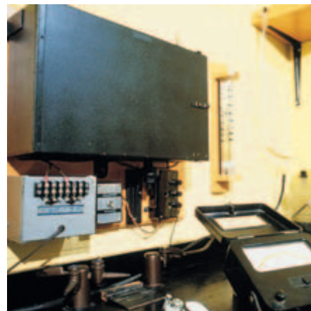
Fig. 2-32. Blaine test apparatus (left) and Wagner turbidimeter (right) for determining the fineness of cement. Wagner fineness values are a little more than half of Blaine values. (IMG12303, IMG12458)
