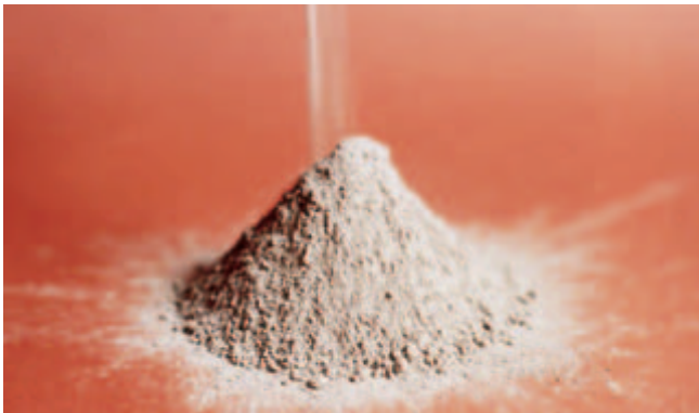
Fig. 2-1. Portland cement is a fine powder that when mixed with water becomes the glue that holds aggregates together in concrete. (IMG12628)
