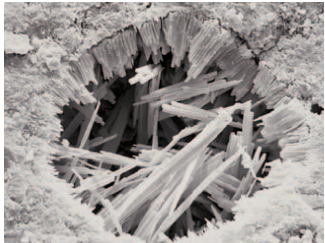
Fig. 1-35. White secondary ettringite deposits in void. Field width 64 \mu m. (IMG12494)
