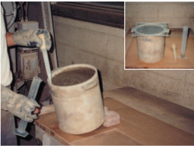
Fig. 16-12. ASTM C232 (AASHTO T 158) test for bleeding of concrete; Method A without vibration. The container has an inside diameter of about 255 mm (10 in.) and height of about 280 mm (11 in.). The container is filled to a height of about 255 mm. Bleed water is drawn off the concrete surface and recorded in regular intervals until cessation of bleeding. Inset: The container needs to be covered throughout the test to prevent evaporation. (IMG12199, IMG15689)
