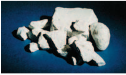
Fig. 2-11. Gypsum, a source of sulfate, is interground with portland clinker to form portland cement. It helps control setting, drying shrinkage properties, and strength development. (IMG12489)
