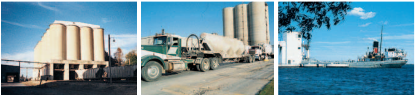
Fig. 2-52. Portland cements are shipped from the plant silos to the user in bulk by (left to right) rail, truck, or water. (IMG12306, IMG12441, IMG12440)
