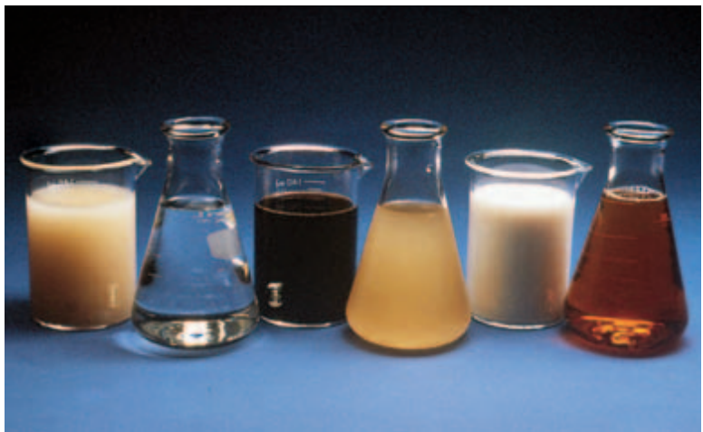
Fig. 6-1. Liquid admixtures, from left to right: antiwashout admixture, shrinkage reducer, water reducer, foaming agent, corrosion inhibitor, and air-entraining admixture. (IMG12188)
