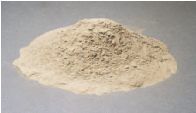
Fig. 3-3. Fly ash, a powder resembling cement, has been used in concrete since the 1930s. (IMG12190)
