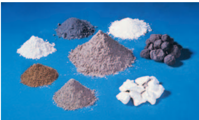
Fig. 2-19. Blended cements (ASTM C595, AASHTO M 240, and ASTM C1157) use a combination of portland cement or clinker and gypsum blended or interground with pozzolans, slag, or fly ash. ASTM C1157 allows the use and optimization of all these materials, simultaneously if necessary, to make a cement with optimal properties. Shown is blended cement (center) surrounded by (right and clockwise) clinker, gypsum, portland cement, fly ash, slag, silica fume, and calcined clay. (IMG12473)
