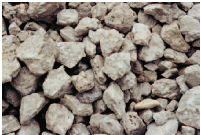
Fig. 5-28. Recycled-concrete aggregate. (IMG12220)
