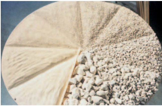
Fig. 5-4. Range of particle sizes found in aggregate for use in concrete. (IMG12320)
