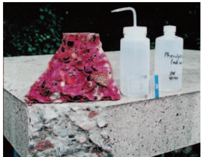
Fig. 16-19. The depth of carbonation is determined by spraying phenolphthalein solution on a freshly broken concrete surface. Noncarbonated areas turn red or purple, carbonated areas stay colorless. (IMG12221)
