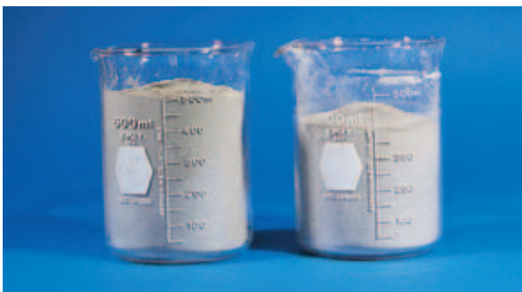
Fig. 2-48. Both 500-mL beakers contain 500 grams of dry powdered cement. On the left, cement was simply poured into the beaker. On the right, cement was slightly vibrated—imitating consolidation during transport or packing while stored in a silo. The 20% difference in bulk volume demonstrates the need to measure cement by mass instead of volume for batching concrete. (IMG12444)
