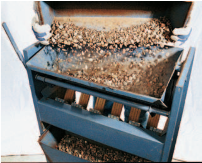
Fig. 16-1. Sample splitter commonly used to reduce coarse aggregate samples. (IMG12347)
