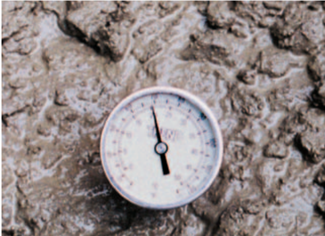
Fig. 16-3. A thermometer is used to take the temperature of fresh concrete. (IMG12201)
