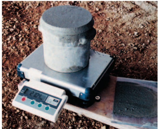
Fig. 16-4. Fresh concrete is measured in a container of known volume to determine density (unit weight). (IMG12178)
