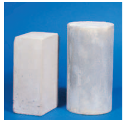
Fig. 2-2. Isle of Portland quarry stone (after which portland cement was named) next to a cylinder of modern concrete. (IMG12472)
