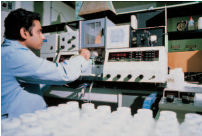
Fig. 4-2. Laboratory analysis of water, in this case using an atomic absorption spectrophotometer to detect concentration of elements. (IMG12313)
