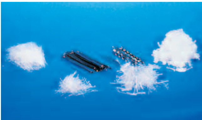
Fig. 7-1. Steel, glass, synthetic and natural fibers with different lengths and shapes can be used in concrete. (IMG12412)
