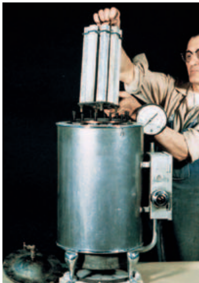
Fig. 2-35. In the soundness test, 25-mm square bars are exposed to high temperature and pressure in the autoclave to determine the volume stability of the cement paste. (IMG12454)
