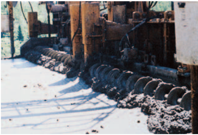
Fig. 10-16. The screw spreader quickly spreads concrete over a wide area to a uniform depth. Screw spreaders are used primarily in pavement construction. (IMG12392)
