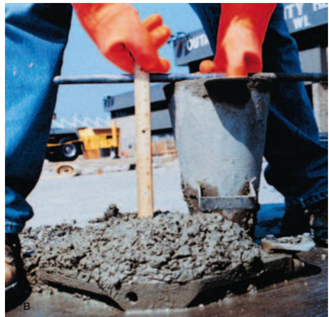
Fig. 16-2. Slump test for consistency of concrete. Figure A illustrates a lower slump, Figure B a higher slump. (IMG12179, IMG12180)
