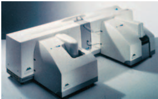
Fig. 2-34. A laser particle analyzer uses laser diffraction to determine the particle size distribution of fine powders. Fig. 2-31 (right) illustrates typical results. (IMG12455)
