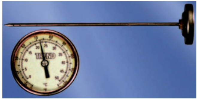
Fig. 14-13. A bimetallic pocket thermometer with a metal sensor suitable for checking fresh concrete temperatures. (IMG12352)
