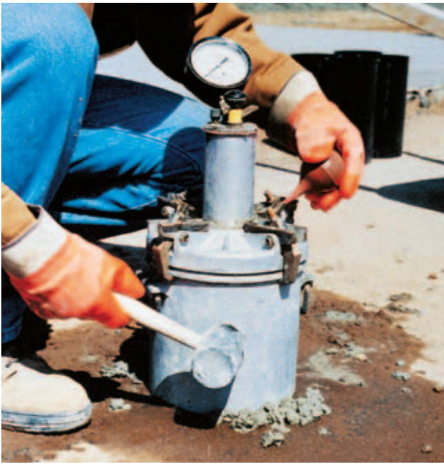
Fig. 16-5. Pressure-type meter for determining air content. (IMG12194)
