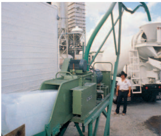
Fig. 13-6. Substituting ice for part of the mixing water will substantially lower concrete temperature. A crusher delivers finely crushed ice to a truck mixer reliably and quickly. (IMG12265)
