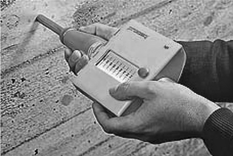
FIGURE 6.6 Rebound hammer test.
