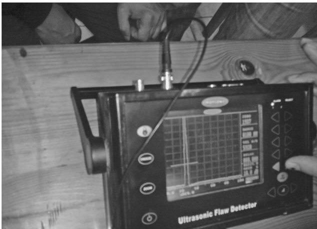
FIGURE 8.42 Echo pattern for discontinuity.
