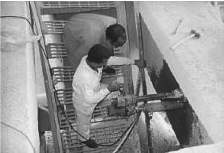
FIGURE 6.2 How to take a core.
