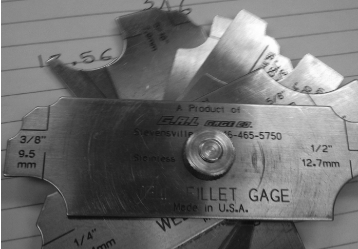
FIGURE 8.1 Fillet weld thickness test.
