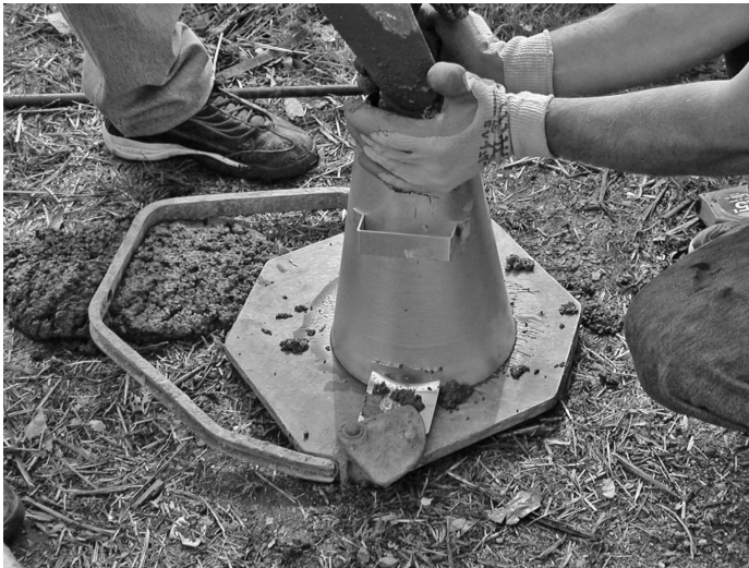
FIGURE 4.12 Pouring concrete in slump.
