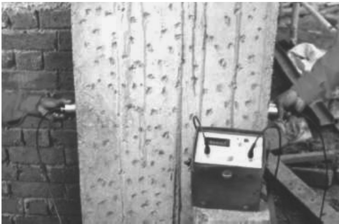
FIGURE 6.10 (a) Direct transmission concept. (b) Direct transmission setup.
