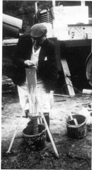
Fig. 6. Timing of the flow (FT) mix. It will also indicate a boundary beyond which the fresh NUWC will cease to be effectively self-compacting.
