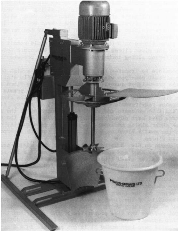
Fig. 2. A high shear cement slurry mixer.
