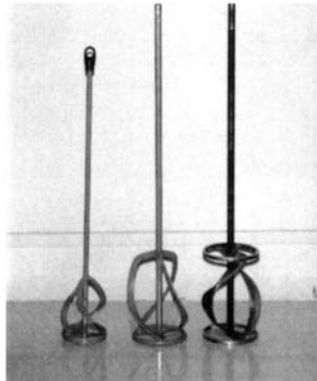
Fig. 6. Different designs of mixing paddles mortar is literally rubbed into the surface of the concrete using a piece of hessian, stiff cloth or polystyrene block.
