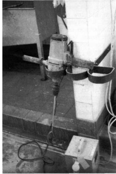
Fig. 5a. and 5b. Slow speed drill and paddle for mixing repair materials
