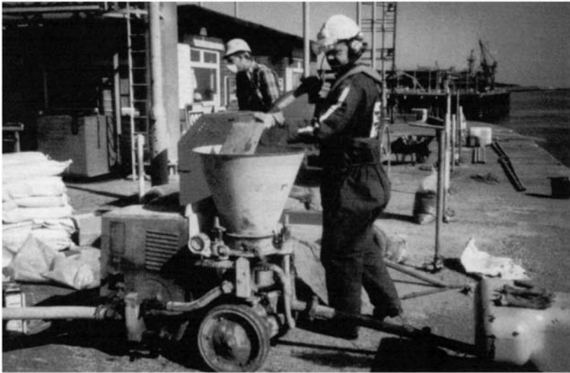
Fig.b 1. Gunite spraying machine showing feed hopper being filled with pre-mixed material machines. Typically, the sand, cement and aggregate and or additives are premixed in a conventional concrete mixer or hand-mixed for smaller jobs. This pre-mix is then introduced into the spraying machine, of which there are several types.
