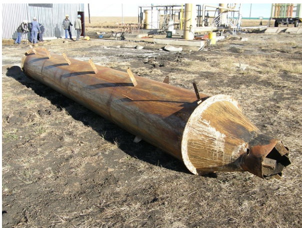
Fig. 14.18 Flare stack replaced due to corrosion.
