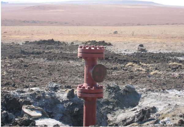
Fig. 14.7 First Majuba “cold air testing” UCG well.
