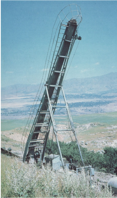
Picture 3.1 Drilling rig NBU ZIF1200.
