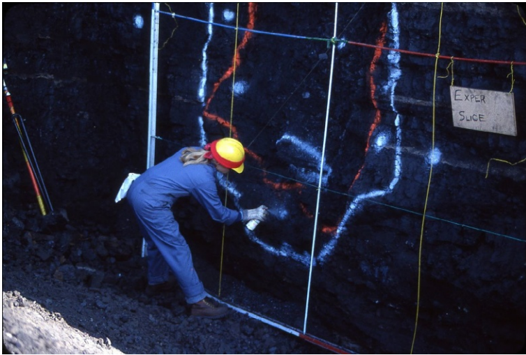
Fig. 4.5 All five of the Centralia Large Block tests were excavated, inspected, described, and documented. This advanced an understanding of the rubble-filled nature of UCG cavities. Photo courtesy of LLNL photo.
