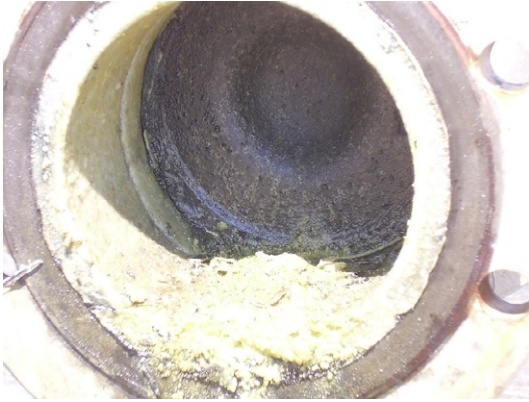
Fig. 14.16 Surface piping scaling—solidified organic condensate deposits.
