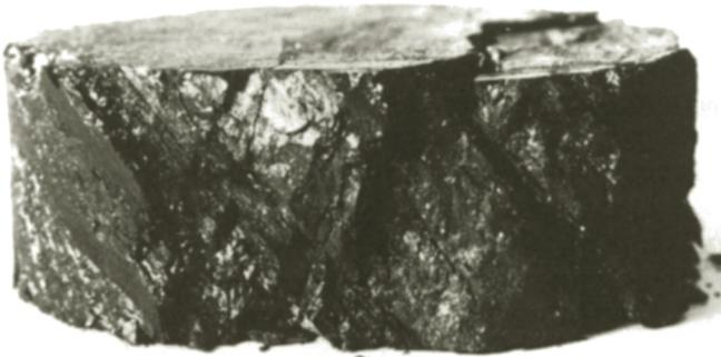
Fig. 12.1.7. Development of tensile fracture-periphery and shear failure-inner body of the model pillar with ratio  $D/H = 3$ .
