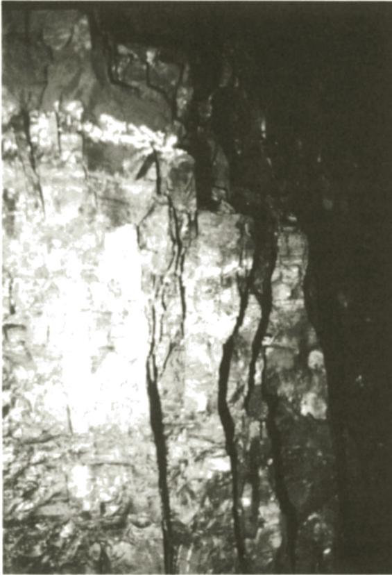
Fig. 1.2.2. Axial failure of coal rib (Western Collieries, Australia).
