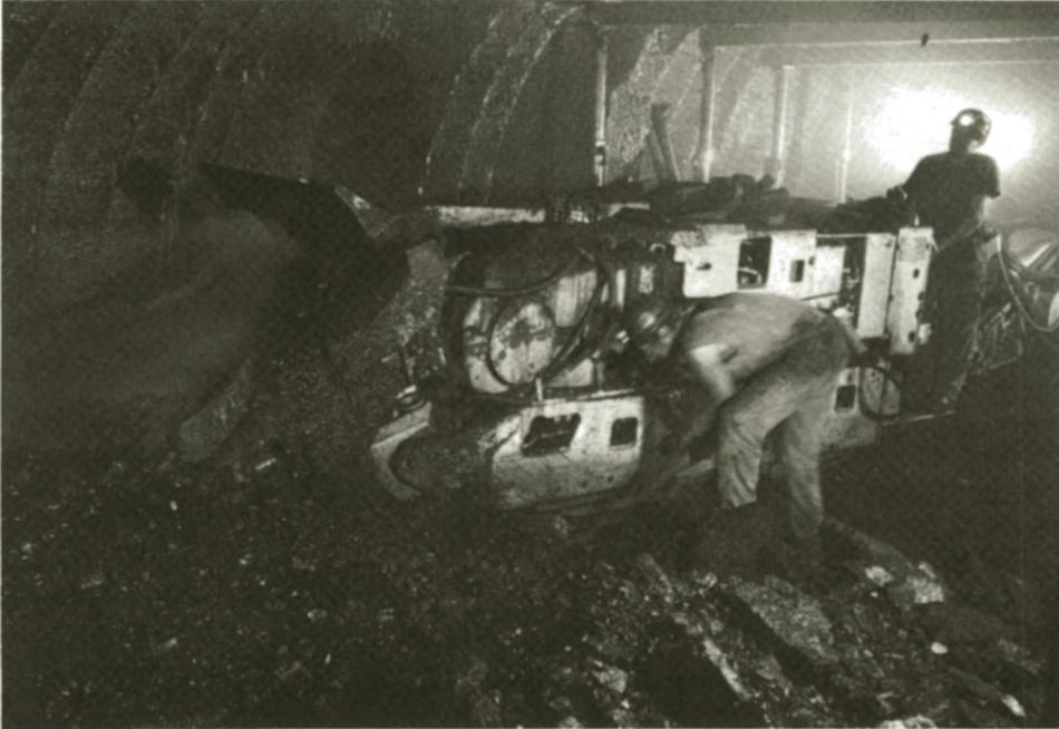
Fig. 7.1.3. Coal excavation by continuous miner (Western No. 2 Mine, Collie Basin, Western Australia).
