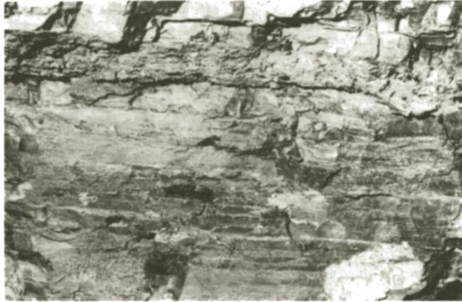
Fig. 6.2.2. Rib wall along cleat in unweathered coal.
