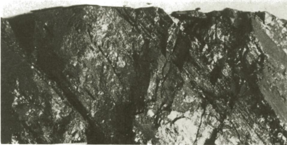
Fig. 6.3.3. Disintegration of coal seam due to intensive shear movement along bedding planes of soft friable coal bands (Cardinal River).
