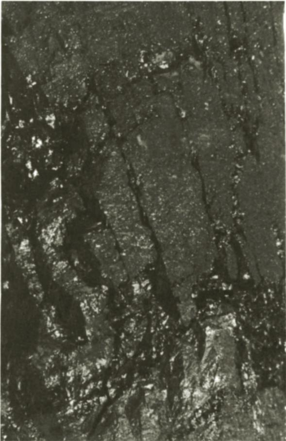
Fig. 3.4.4. Induced cleavage by mining operation (Canmore Mine).
