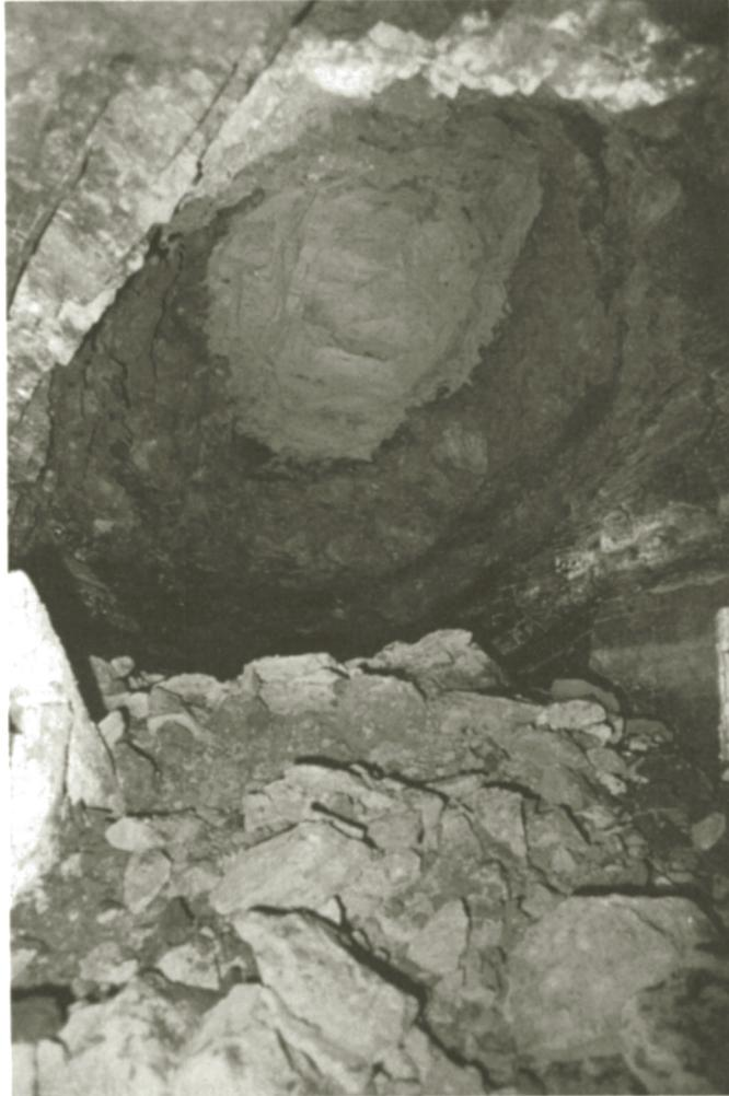
Fig. 4.2.10. Caving geometry and caved rock fragmentation of the thin and friable roof.
