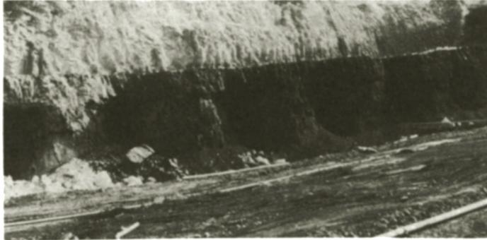
cycle. Coal is drilled with electric auger drills and blasted using half second delay detonators and semi-gel non-permitted explosives. The broken coal is loaded by small 'Bobcat' front end loaders onto a chain conveyor, which delivers coal to a belt conveyor system for transportation to the surface.<sup>1</sup>
