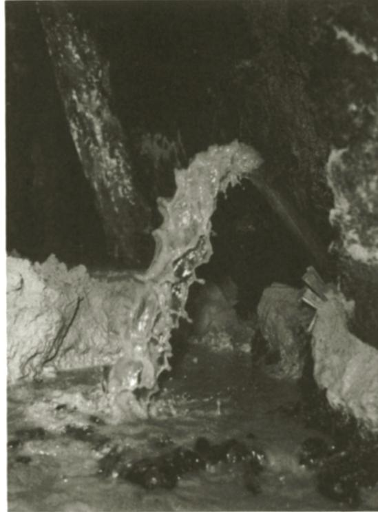
Fig. 5.4.6. Dewatering of the water saturated sand which is immediate floor of the thick coal seam (Kreka Coal Mine, Yugoslavia).
