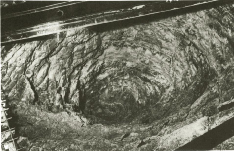
Fig. 6.1.5. Cavity left by a coal outburst at Leichhardt Colliery Australia (courtesy of Lama).
