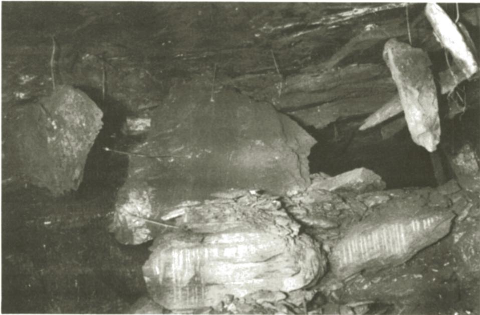
Fig. 5.2.4. Roof falls in compressive stress field (sandstone).
