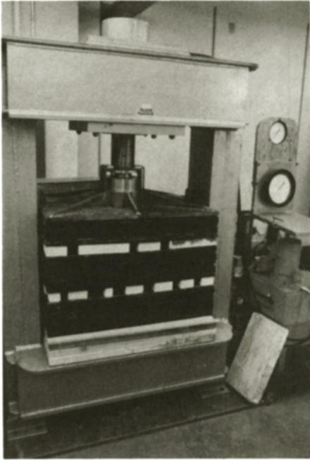
7.3.10. Set up of three-dimensional model of multiple seam mining by room-and-pillar system.
