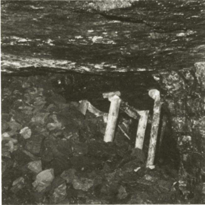
Fig. 4.1.9. Uncaved part of a mine roof after the timber was withdrawn from the room.
