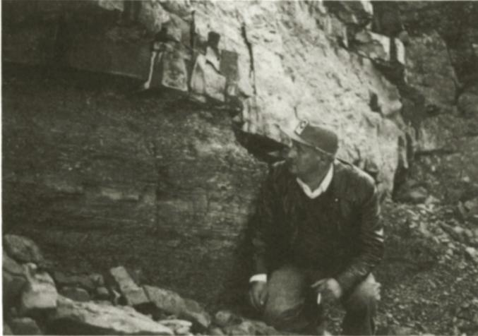
Fig. 2.3.3. Laminated shale beds without self-supporting abilities (false roof) covered with medium bedded siltstone (immediate roof).
