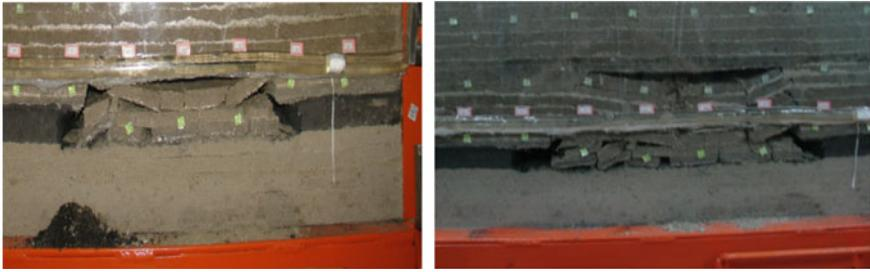
**Fig. 6.18** Continued fall and initial collapse of roof
