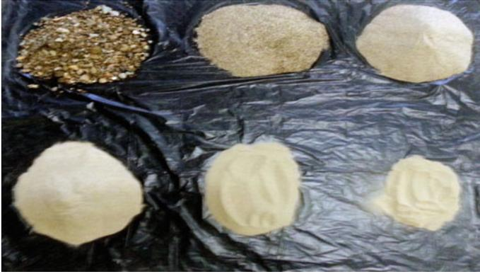
**Fig. 6.28** The screening results of sandstone particles
