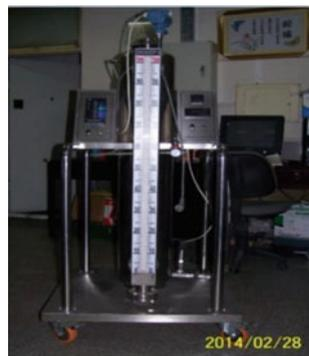
**Fig. 6.4** Automatic injection device for water. Notes 1—flat car; 2—water outlet; 3—water inlet valve; 4—water pressure sensor; 5—water level display; 6—water level record scale; 7—air inlet; 8—water seepage flow time display; 9—Water pressure indicator; 10—pressure gauge; 11—container tank filled with water (alkaline water); 12—high pressure nitrogen tank
