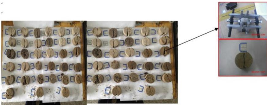
**Fig. 6.14** Samples for tensile strength
