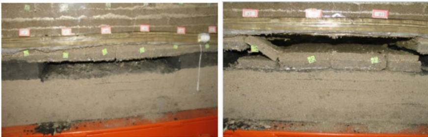
Fig. 6.17 Cracks and initial caving in direct roof
