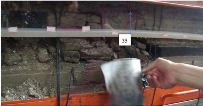
**Fig. 6.27** Water–sand inrush channel near stop mining line
