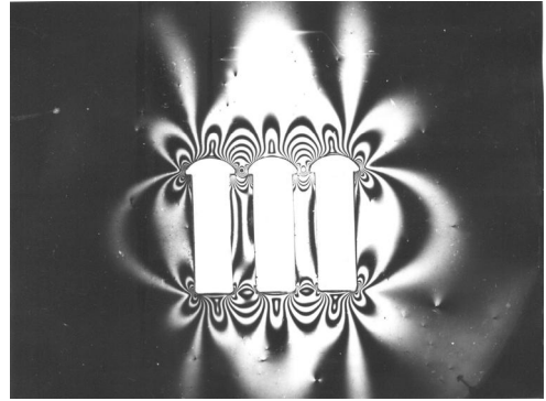
Figure 3. Isochromatic lines of stresses around the excavations obtained with photo elasticity method.
