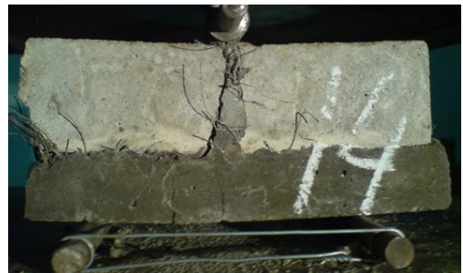
Figure 2. Test of bilayer specimen with 20 mm height of macro synthetic FRC: disrupted shotcrete (top), restored coating of FRC with a rigid macro synthetic fibers (bottom).
