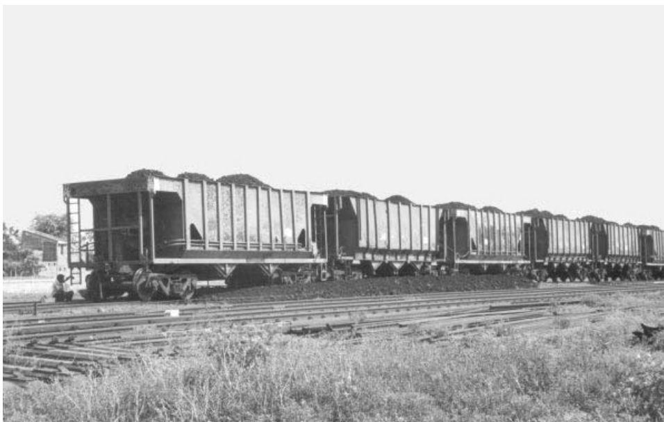
Figure 13.9 Bottom discharge wagons (60 t), on Eastern Railways, India. (Photograph by courtesy of Dargo Associates Ltd.)
