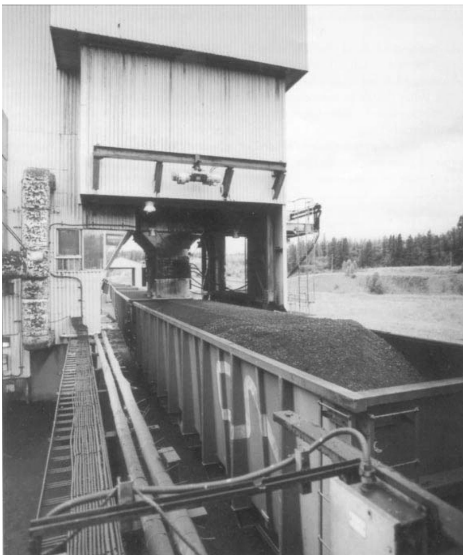
Figure 13.7 Automatic loading of trains, each wagon receives exact tonnage as train moves slowly through loading bay, Alberta, Canada. (From Howland, 1998.)
