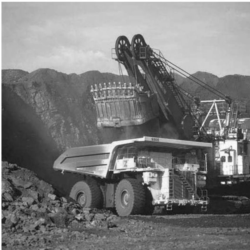
Figure 10.17 Large dump truck (280 t) being loaded at Fording coal mine, Canada. (Photograph by courtesy of Komatsu Mining Systems.)
