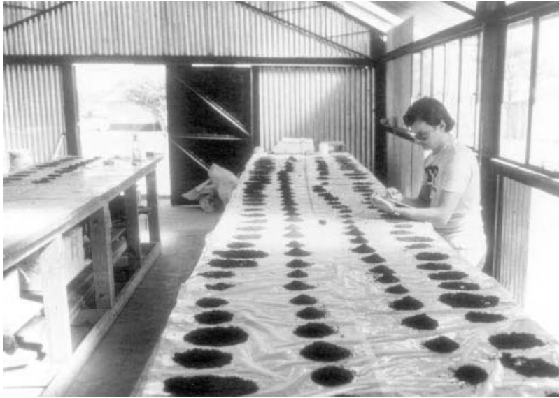
Figure 6.22 Coal geologist logging borehole chip samples in an on-site core shed. (Photograph by M. C. Coultas.)
