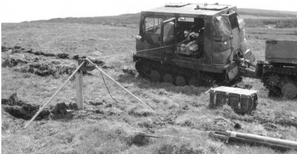
Figure 8.21 Mobile geophysical logging unit. (Reproduced with permission of Robertson Geologging Ltd.) This figure is reproduced in colour in the Plates section.
