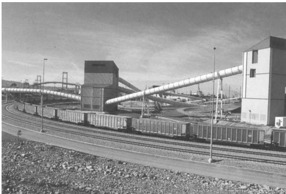
Figure 13.10 Large train units transporting 12,000 t over 1200 km in western United States. (From Harder, 1998.)
