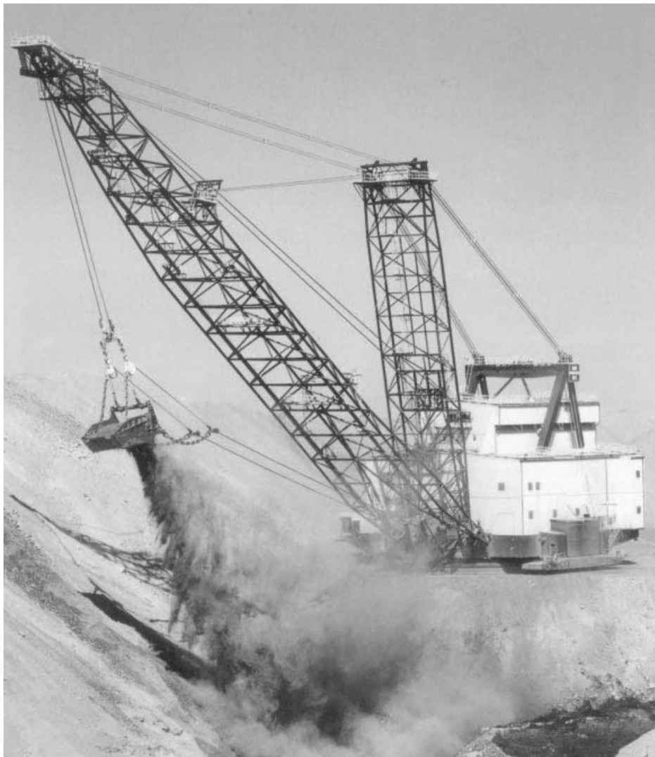
Figure 10.15 Dragline removing overburden in opencast mine, USA. courtesy of Bucyrus International Inc. Reproduced by permission of World Coal , Palladian Publications Ltd.
