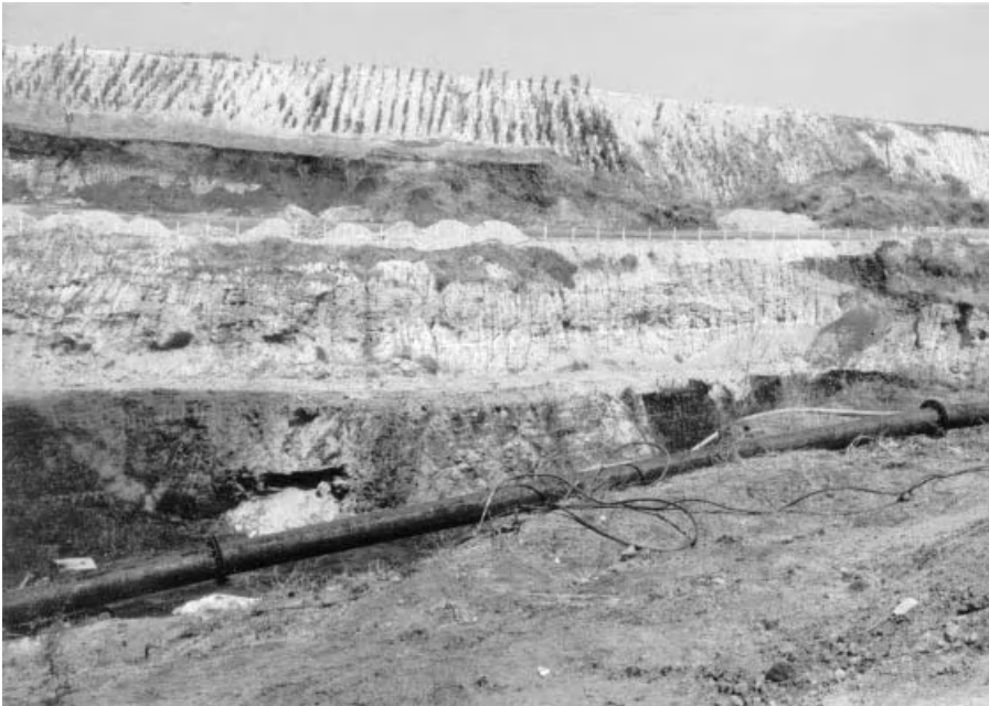
Figure 12.5 Opencast mine in Maharashtra State, India, showing protective bund of overburden to prevent flooding from nearby river. (Photograph by courtesy of Dargo Associates Ltd.)
