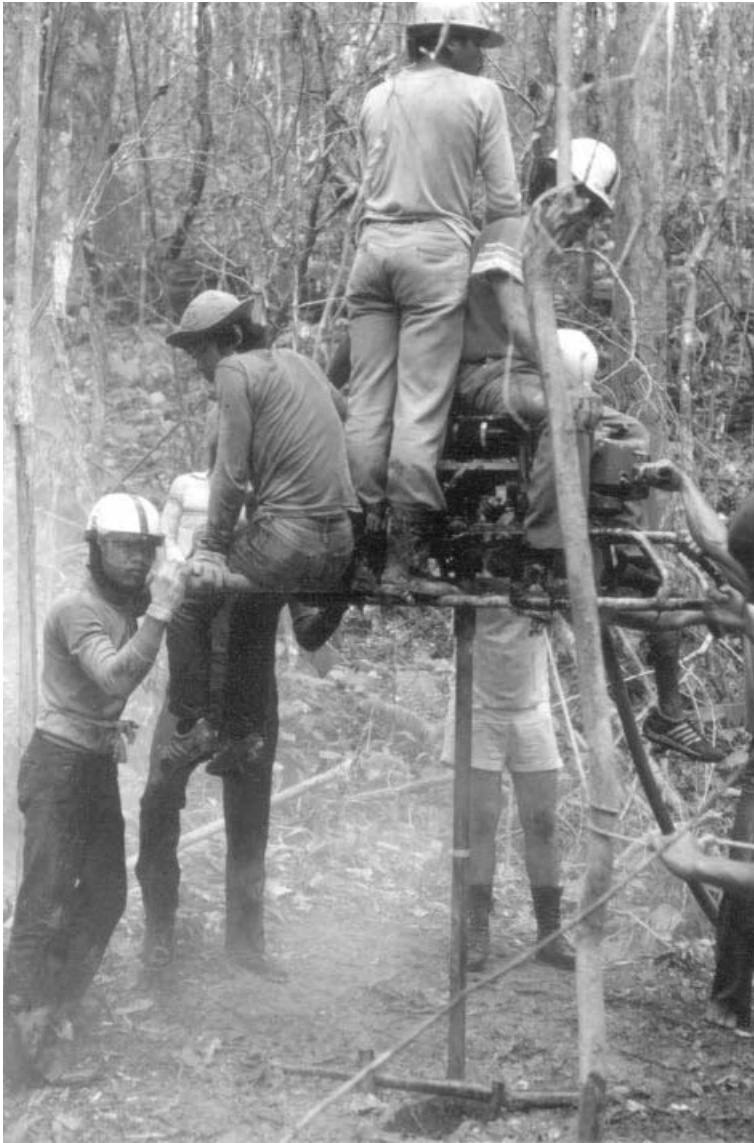
Figure 6.18 Portable drilling rig using manpower to exert downward pressure on the drill bit. In use in East Kalimantan, Indonesia. (Photograph by LPT.)
