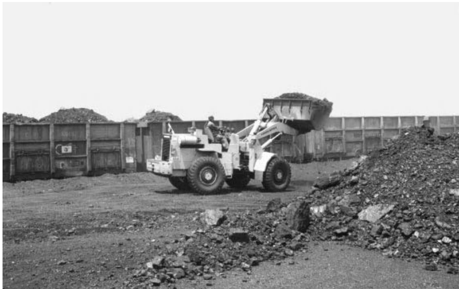
Figure 13.8 Train being loaded by payloader, Orissa State, India. (Photograph by courtesy of Dargo Associates Ltd.)
