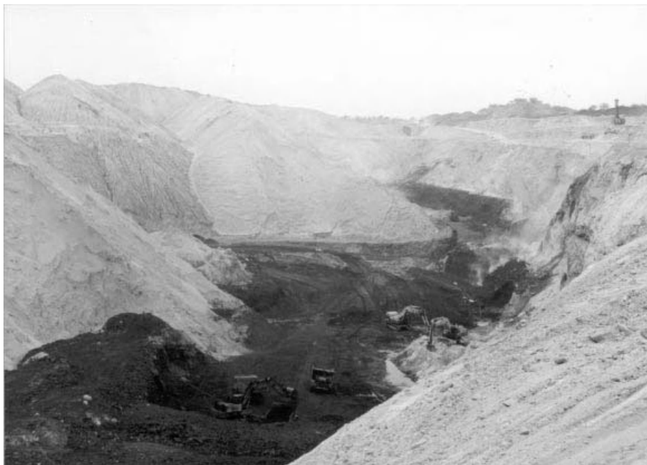
Figure 10.19 Coal being loaded into trucks by hydraulic excavators, Western Coalfields, India. (Photograph by courtesy of Dargo Associates Ltd.)
