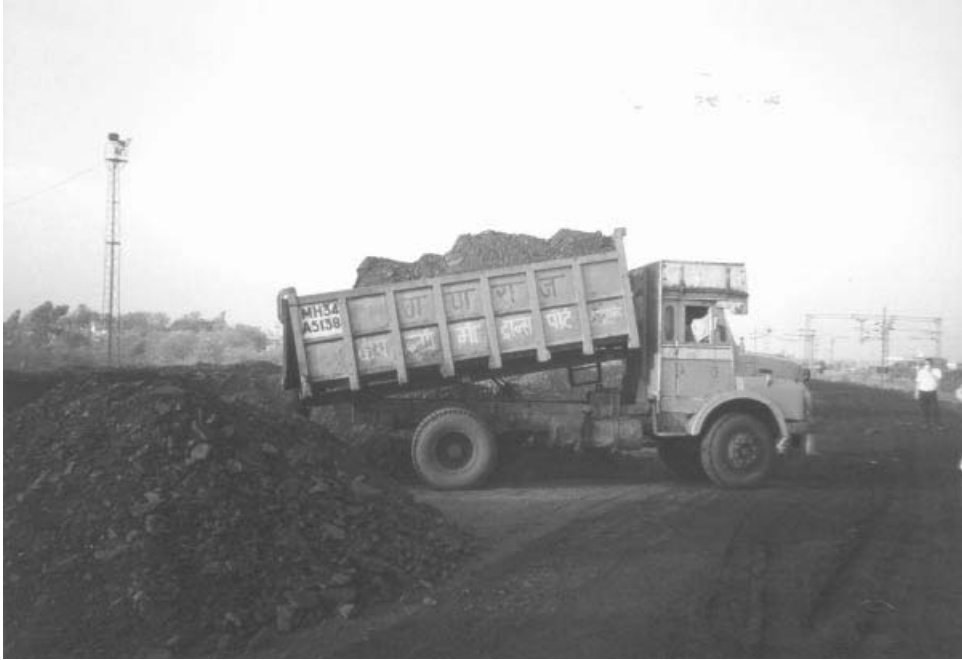
Figure 13.5 Coal transportation by small capacity 10 t truck, India. (Photograph by courtesy of Dargo Associates Ltd.)
