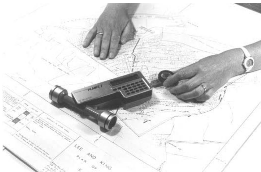
Figure 7.8 Digital planimeter being used to calculate coal reserve areas within a working mine. (Photograph by M.C. Coultas.)
