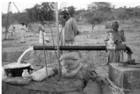
Figure 9.3 Pumping test in operation in the Thar Coalfield, Pakistan. (Photograph by Dargo Associates Ltd.)
