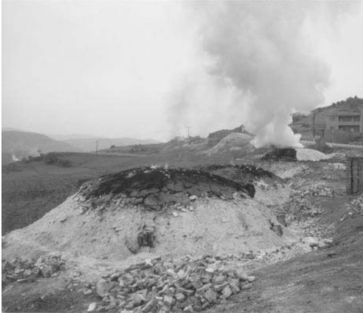
Figure 12.16 Local coke manufacture in small ‘ovens’, Guizhou Province, People’s Republic of China. (Photograph courtesy of Dargo Associates Ltd.)
