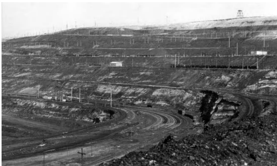
Figure 10.25 Multiple rail system in Ekibastuz mine, Kazakhstan. (Photograph by courtesy of Dargo Associates Ltd.)
