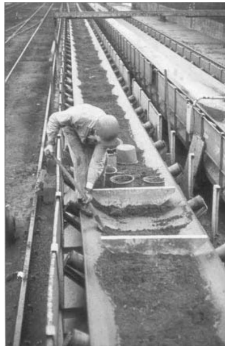
Figure 5.5 The collection of a stop belt sample from a main conveyor. (From Mazzone 1998.)
