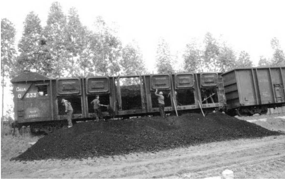
Figure 13.11 Top discharge wagons with drop down doors for side unloading. Guizhou Province, People's Republic of China. (Photograph by courtesy of Dargo Associates Ltd.)
