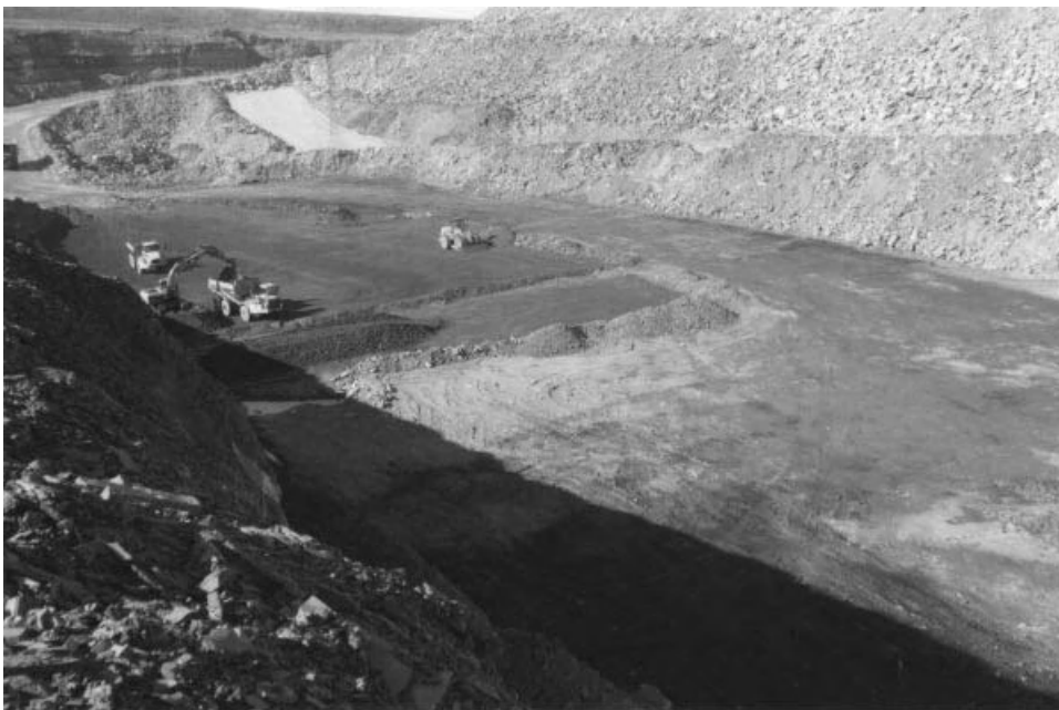
Figure 10.21 Truck and shovel operation, Shotton opencast mine, Northumberland, United Kingdom. (Photograph by courtesy of M. C. Coultas.)
