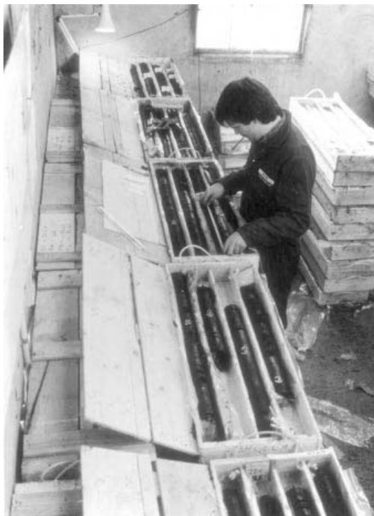
Figure 6.19 Coal geologist logging borehole core in a core shed on-site. (Photograph by LPT.)
