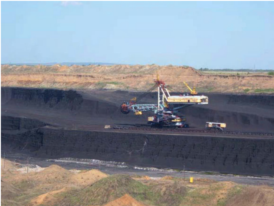
Figure 10.18 Large BWE and conveyor system in operation in Bereзовский opencast mine, Kansk-Achinsk Basin, Russian Federation. (Photograph by courtesy of Dargo Associates Ltd.)
