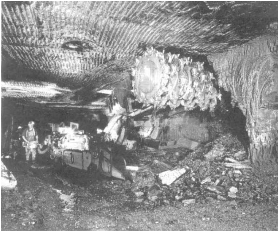
Figure 10.6 The EIMCO Dash Three Continuous Miner in operation in Alabama, United States. (Photograph by courtesy of EIMCO, Bluefield, West Virginia, United States.)
