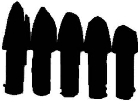
Figure 9.8 Stages of wear on a cutting bit.
