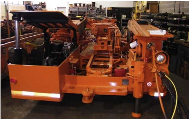
Figure 15.1 The drill unit for in-mine horizontal drilling.
