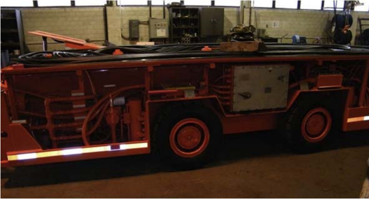
Figure 15.2 The auxiliary unit for in-mine horizontal drilling.
