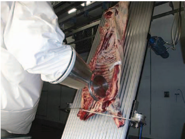
Figure 2.14: Beef scribing robot. Source: Machinery Automation & Robotics.
