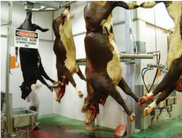
Figure 2.7: Electronic bleeding unit used immediately post stunning and before the carcasses are dressed. The electrodes operate through the hind leg as shown. Source: I.J. Richards.
