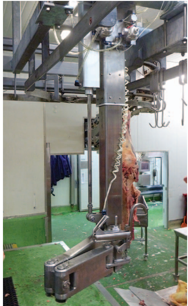
Figure 2.15: Beef boning unit, involving a mechanical arm. Source: Robotic Technologies Ltd.
