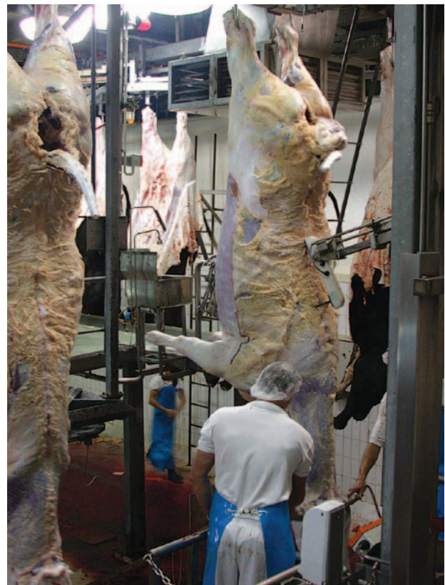
Figure 2.9: Rigidity probe in combination with a downward hide puller. Source: CSIRO Food and Nutritional Sciences.
