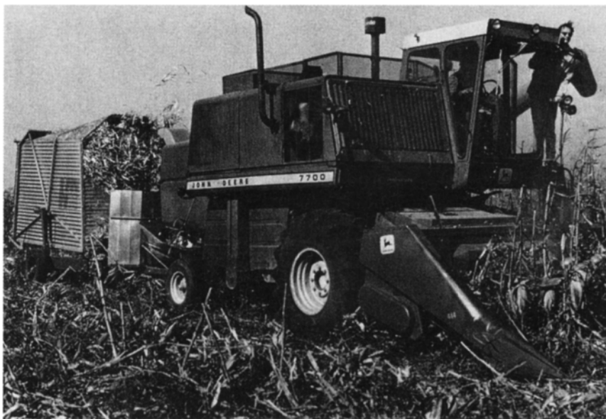
Fig. 12.3 The equipment illustrated here gathers husks, cobs, and bypassed grain into stacks. (Photo courtesy of BEEF Magazine.)
