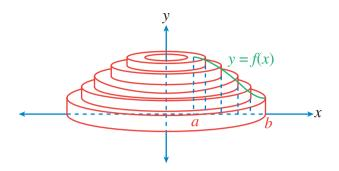
4 Let's take a look at just one of those many "shells" (or pieces of pipe). The shell has an outer radius, r<sub>2</sub>; an inner radius, r<sub>1</sub>; and a height of just h. One other dimension, labeled R, is the distance from the axis of revolution to the center of the thin red shell.
