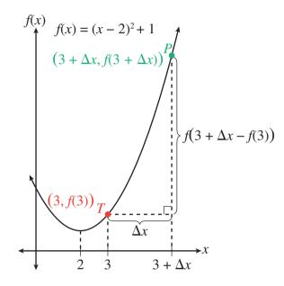
**6** As  $\Delta x \rightarrow 0$ , the point P moves extremely close to the point T; in this case, the slope of the line tangent at point T will be the expression in Step 5 above.
