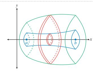
3 Let's look at just the thin red washer for a moment. It has an inner radius of *r* and outer radius of *R*, with a height (or thickness) of *h*.
