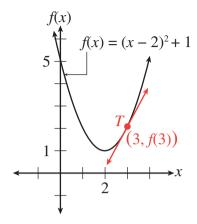
2 Let's approximate the slope of that red tangent line. Select some values of x that approach 3 from the right side: 4, 3.5, 3.1, 3.01, and, of course, 3. Letting  $\Delta x$  (read "delta x") equal the difference between the selected value of x and 3, you can complete the chart at the right.
