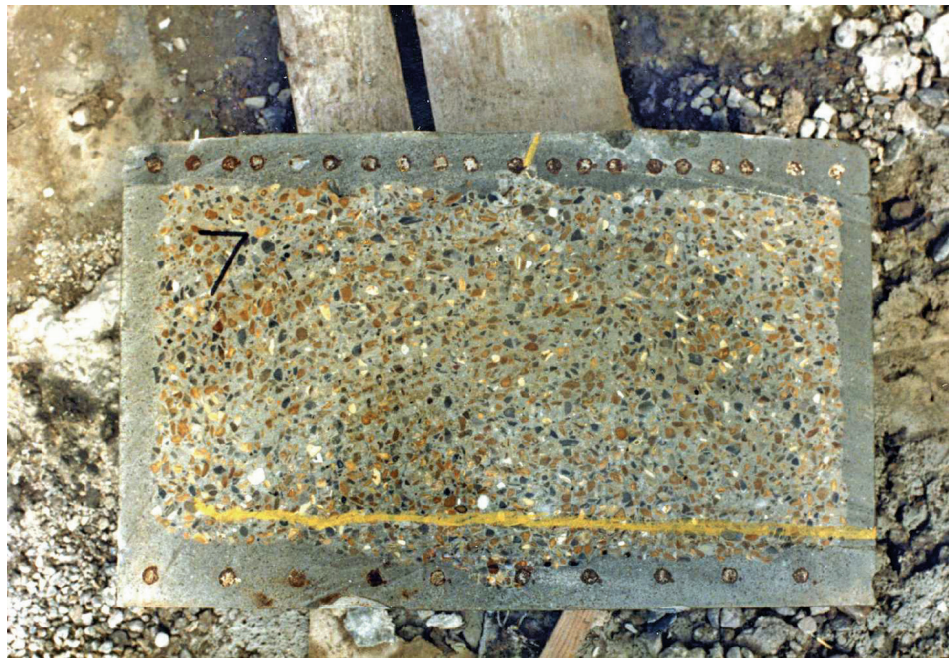
Figure 5.1 – Model beam repair
