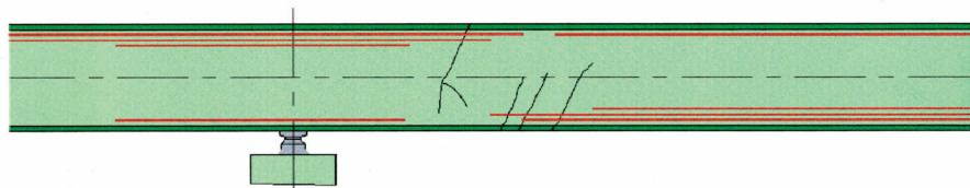
Figure 1.3 – Beam elevation showing main reinforcement and cracks
