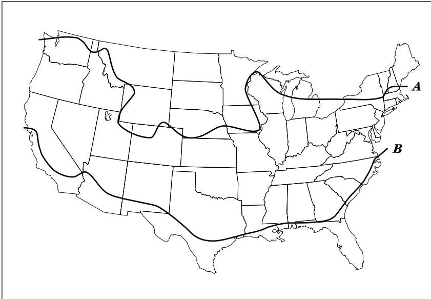
Figure 2.7 Regions of termite and drywood damage. (Adapted from Timber Construction Manual , fifth edition, Ref. 2.17.)
