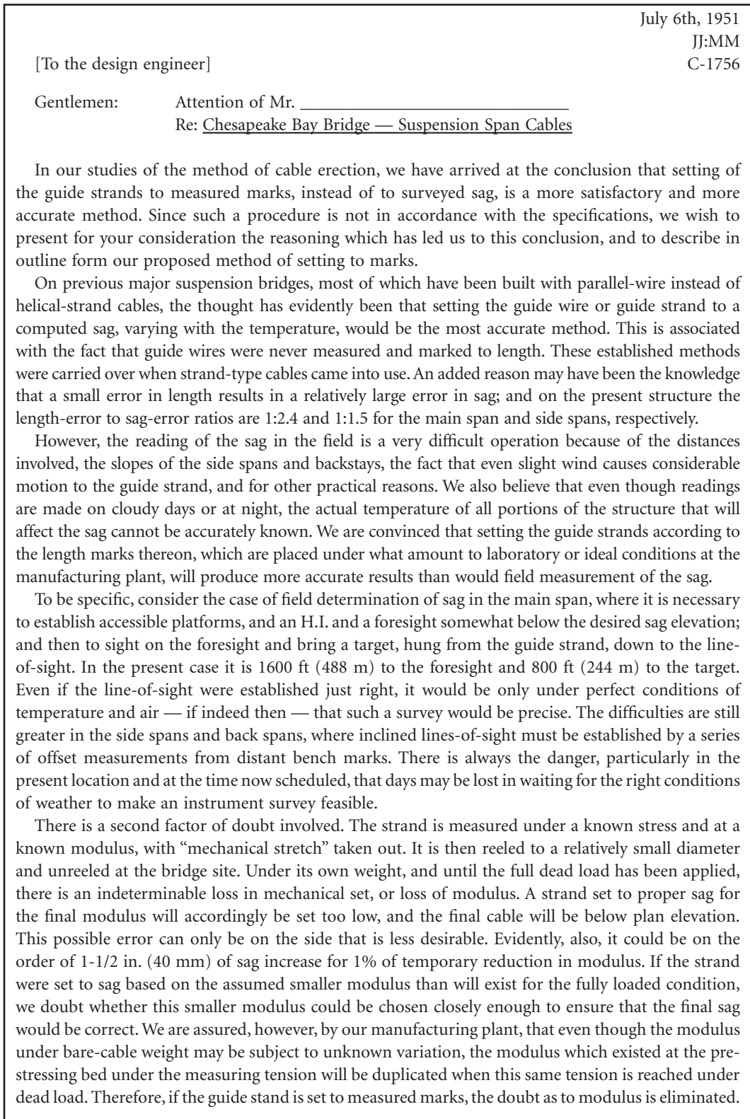
FIGURE 1.7 Setting cable guide strands to marks.
