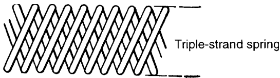
Fig. 8 This flexible shaft permits any shaft angle. These shafts, if long, should be supported to prevent backlash and coiling.
