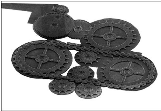
Fig. 12 Microchain Drive: This 50-link microchain drive resembles a bicycle chain and sprocket assembly except that each link of the microchain could rest with atop a cross section of human hair with space to spare. The distance on centers between chain links is 50 \mu\text{m} . (The diameter of a human hair is 70 \mu\text{m} .) Because this microchain can rotate many sprockets, a single tiny MEMS motor coupled to the drive shaft of a single sprocket can rotate many other sprockets linked to the microchain. Typically, a single MEMS motor powers each MEMS device. Chain systems, unlike stroke systems, perform oscillatory motions permitting both continuous and intermittent drive translation.
