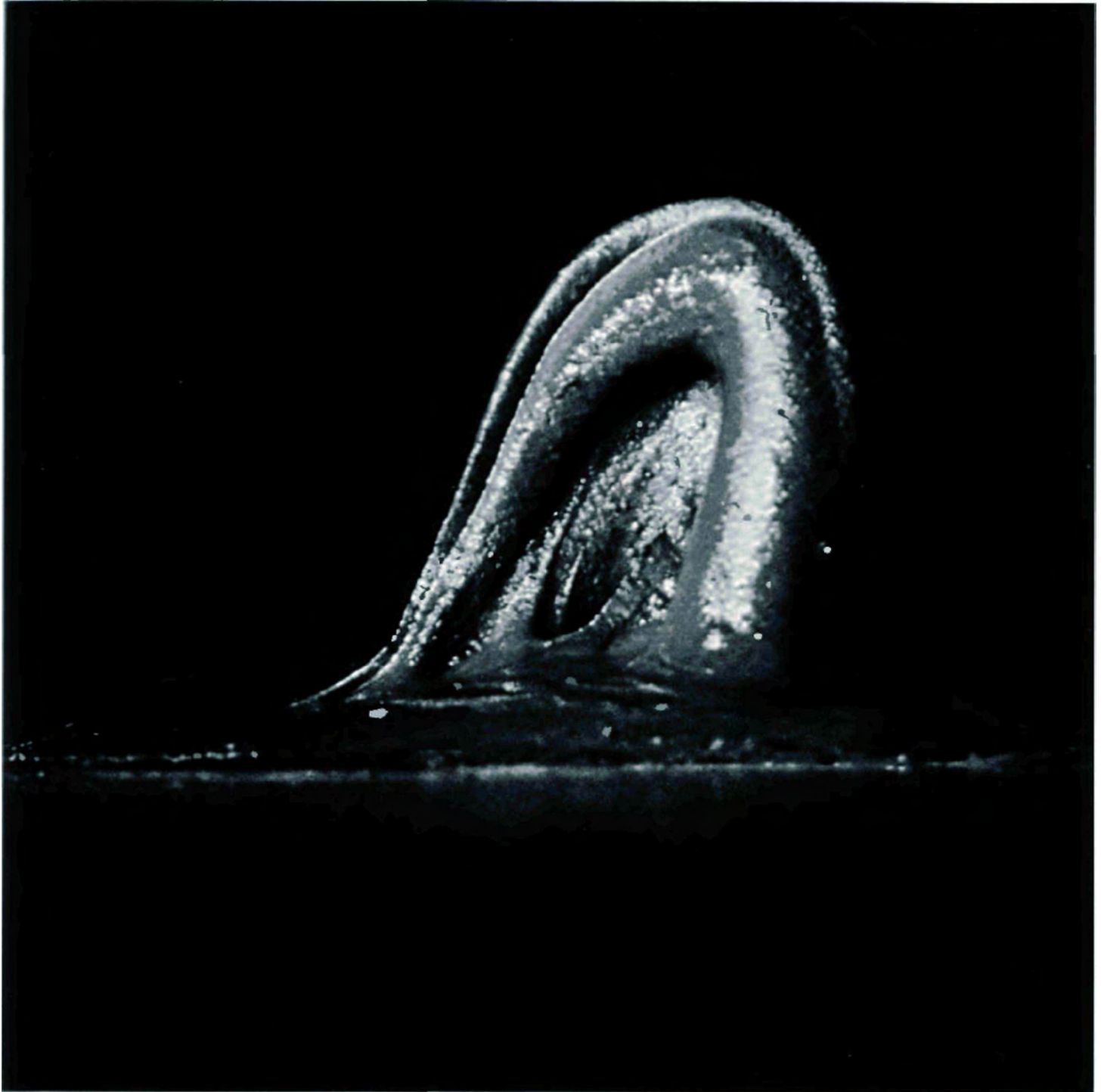
53 A ferromagnetic mass placed in the magnetic field can conform to the pattern of its lines of force when excited by vibration. Adhesion and cohesion are reduced. Under these conditions the characteristics of magnetic space are made visible. What we see here is not a rigid arch but, so to speak, a flowing piece of sculpture. (See page 174.)
