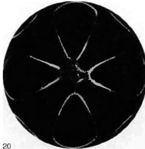
20 Sonorous figure on a circular plate. Diameter 16 cm, frequency 1060 cps. The nodal lines are made visible by sand.
