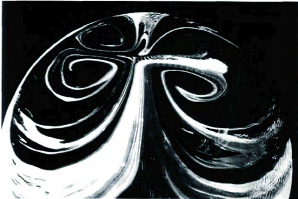
63 Another detail from an experiment with vortices. A pair of vortices, the one on the right turning in a clockwise direction and the one on the left in a counterclockwise direction. This experiment is also audible.
