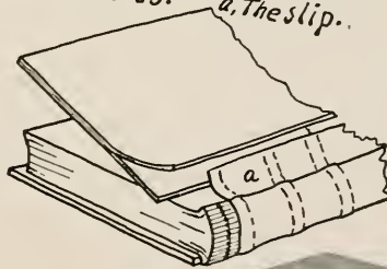
Fig.22. Ready for backing. a. Joint. b. Backing boards. c. Lying, or finishing press.
