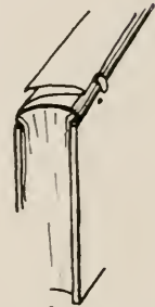
Fig.33. Folded paper for hollow back cover.
