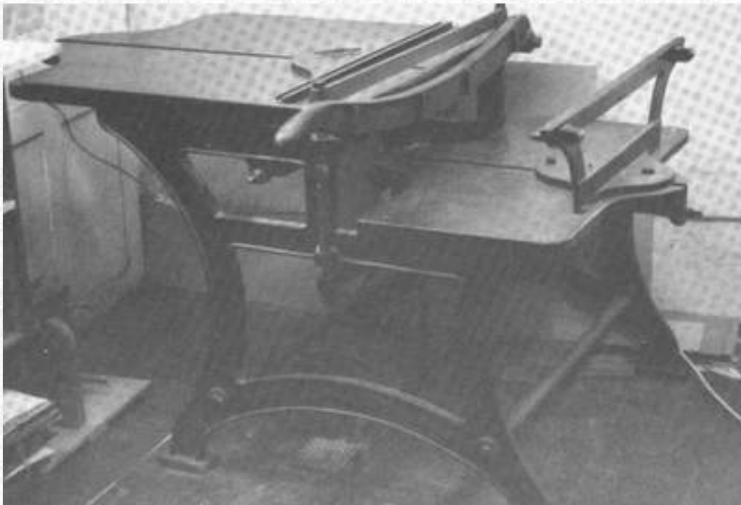
Fig 12. Board cutter in a corner of the author's bindery
