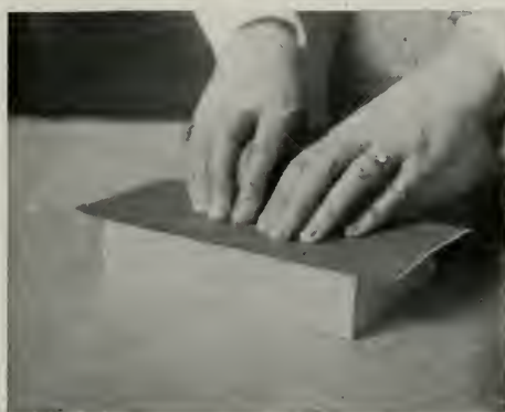
PLATE XXXVI. An illustration of the method of covering the outside of the case when a block of wood is used.
