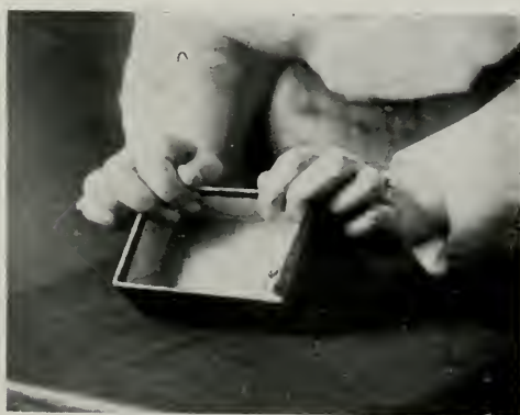
PLATE XXXI. Showing method of pasting the laps to the inside of the box.
