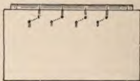
Fig. 58—English style of lacing boards.
