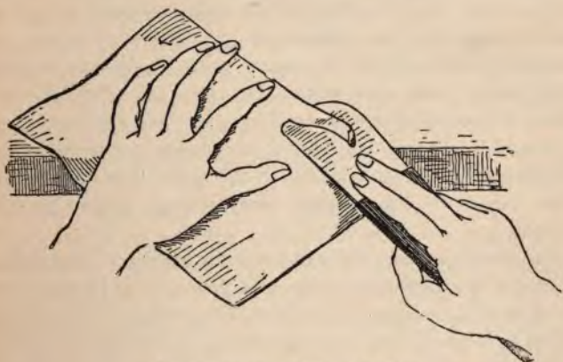
Fig. 63—Paring with French knife.
