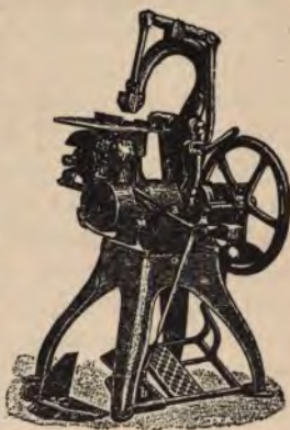
Fig. 19—Small stapling machine for single sheets.
