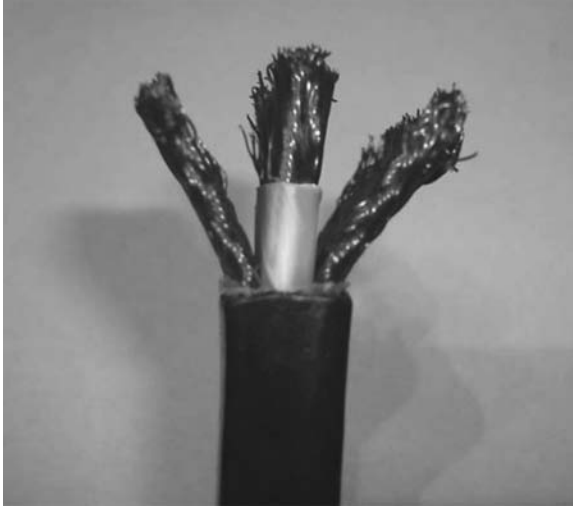
FIGURE 8.11 Virtually concentric Litz cable for 20 kHz power distribution (from M.R. Patel, NASA Report CR-175071, 1986).
